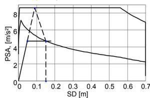
Figure 5. Seismic demand spectra vs. capacity diagram for Frame B - Vrancea
