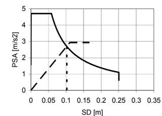
Figure 2. Seismic demand spectra vs. capacity diagram for Frame A - Banat
