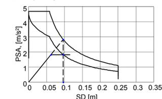
Figure 4. Seismic demand spectra vs. capacity diagram for Frame B - Banat
