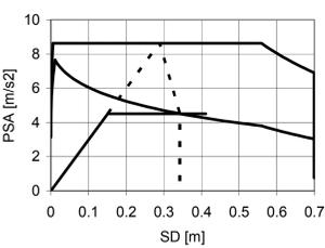
Figure 3. Seismic demand spectra vs. capacity diagram for Frame A - Vrancea
