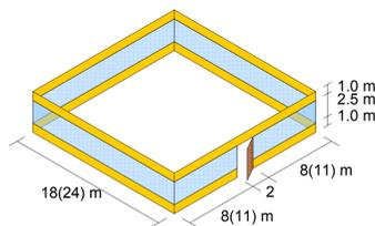
Figure 6. The fire compartment
