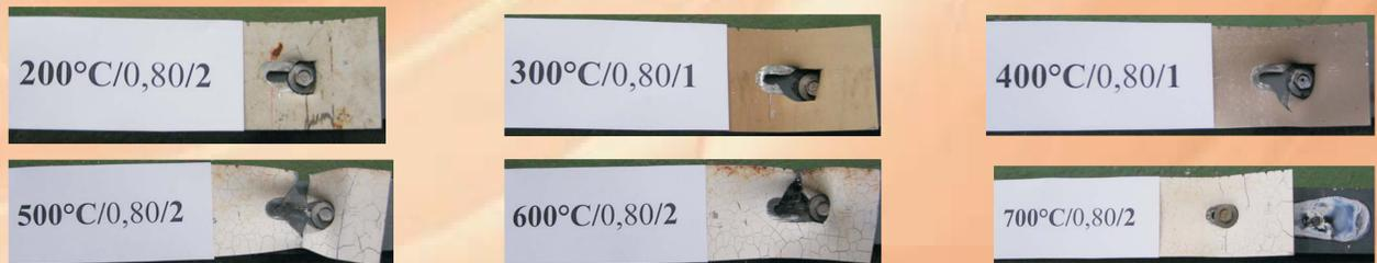
The collapse modes of the connection at specific temperatures
