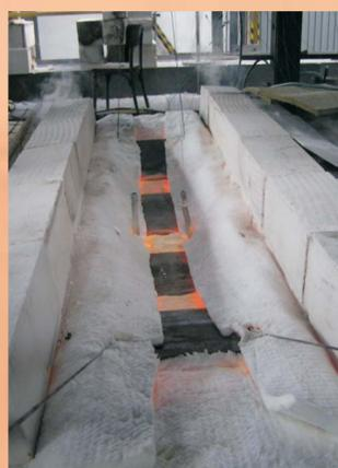
The catenary action of trapezoidal sheet during the fire test
