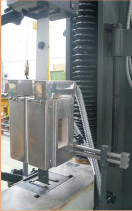
The electric furnace with window
