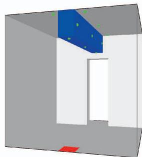
Figure 1 The model set up in FDS. Grey walls of concrete, blue box represents the structural element, the red plate represents the heat source and the green points represents the reference point in which the adiabatic surface temperature was calculated.
