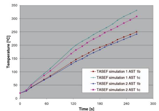
Figure 2 Comparison of thermal calculations performed on the beam of dimensions 200 mm x 300 mm x 9.5 mm with  $T_{AST}$  from each of the two simulations.
