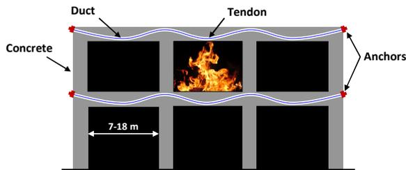
Figure 1: Single bay fire in a multi-bay structure
