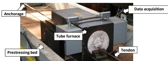
Figure 3: Localized heating relaxation tests on stressed tendons
