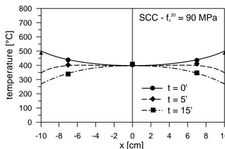
temperature profiles in a typical test ( $T = 400^\circ\text{C}$ )
