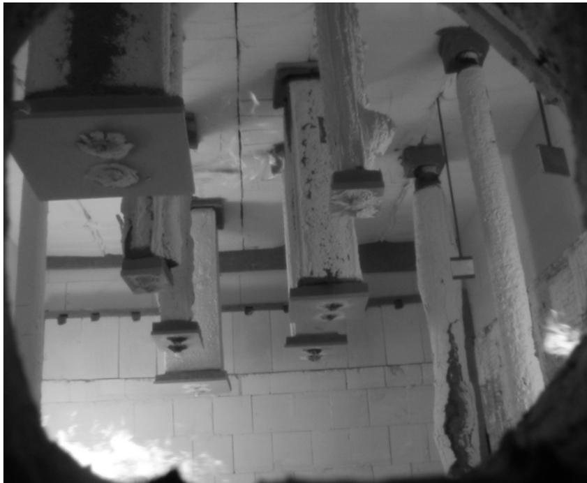
*Fig. 1* The fire test of Promapaint SC, see [7]
