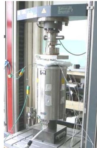
Fig. 2. Testing device at high temperatures
