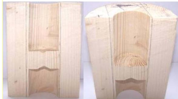
Fig. 10. Views of a cut specimen after test (test 5)
