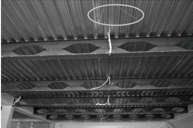
*Fig. 5* Thermocouples for gas and steel temperatures
