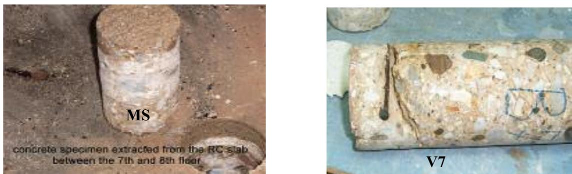
*Fig. 5.* Change of concrete colour and deterioration of surface layers of specimens
