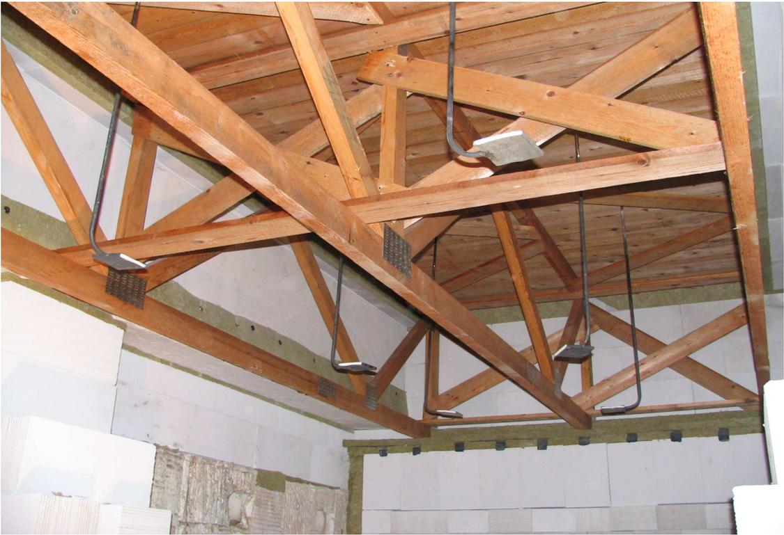
*Fig.2.* Structure No. 1 before the fire test
