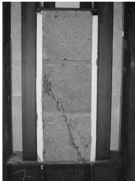
*Fig.7. 1100°C concrete block unexposed face*
