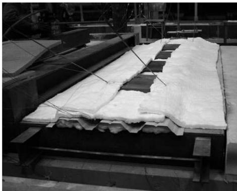
Fig. 4 The tested specimen before fire experiment
