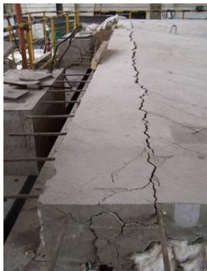
Fig. 11. Cracks along the long edge
