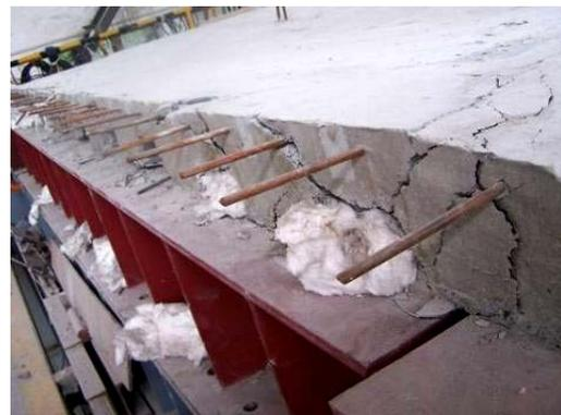
Fig. 12. Cracks along the short side face
