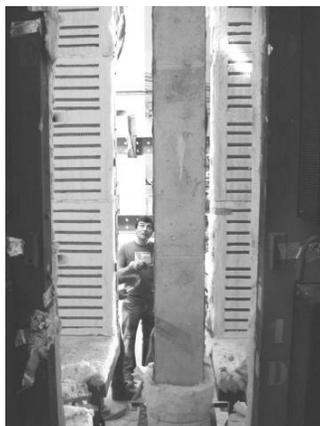
Fig. 9. Column C1 after test
