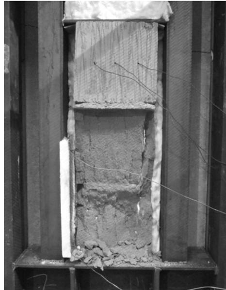
*Fig .5. 1100°C unexposed face*
