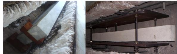
Fig. 4. Heating of beam specimens in oven
