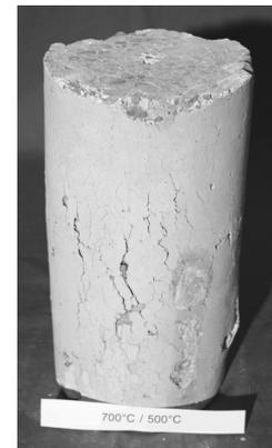
*Fig.4.* Concrete specimen after the test
