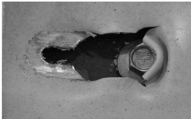
Fig. 9 The collapse mode of the connection from set C, temperature 200°C
