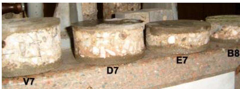
*Fig. 6.* Deteriorated concrete specimens, prepared for testing
