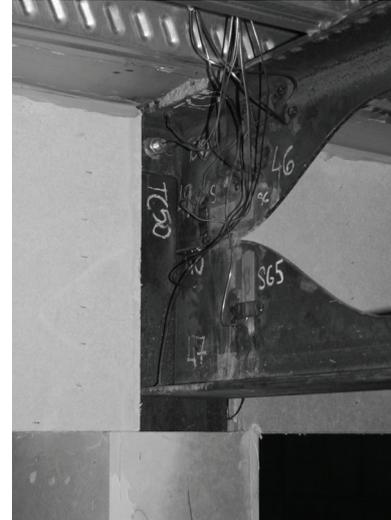
*Fig. 6* Thermocouples on beam to column connection
