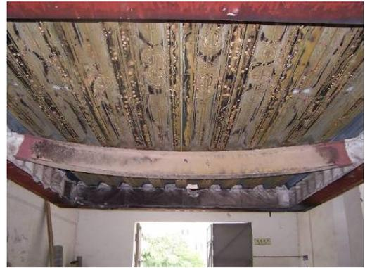
*Fig.16.* The deformation at the bottom of S-2 after the test
