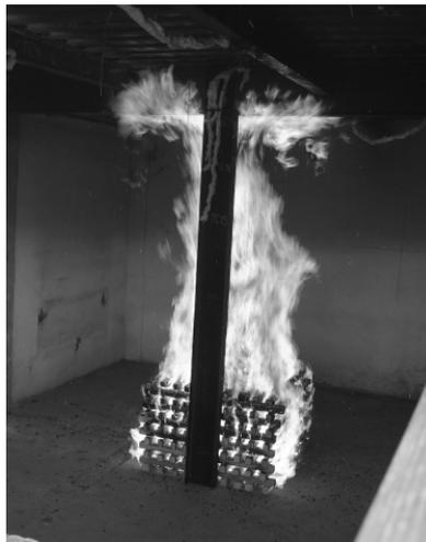
Fig. 1. Column exposed to localised fire, fire test Mittal Steel, Ostrava, June 2006
