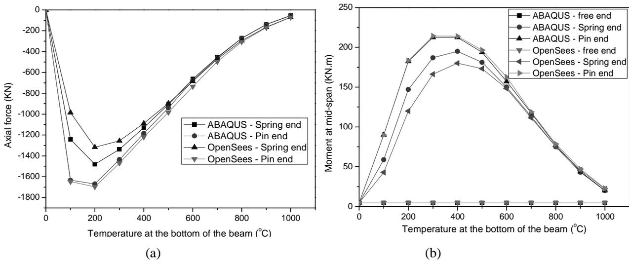
Fig. 6 Forces in the beam with different translational end restraint: (a) axial force; (b) mid-span moment
