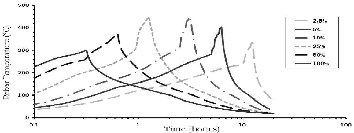
Fig. 4 Resulting temperature of the rebar in the concrete slabs for the family of fire sizes (Law et al., 2011)
