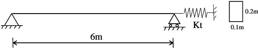
Fig. 3 Simply supported beam with a translational spring at end
