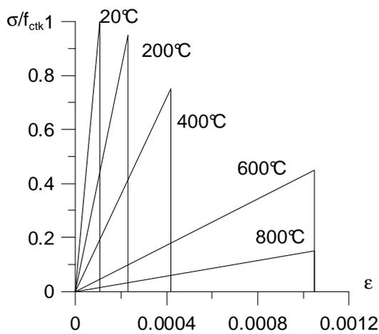
Fig. 4 Concrete in tension.
