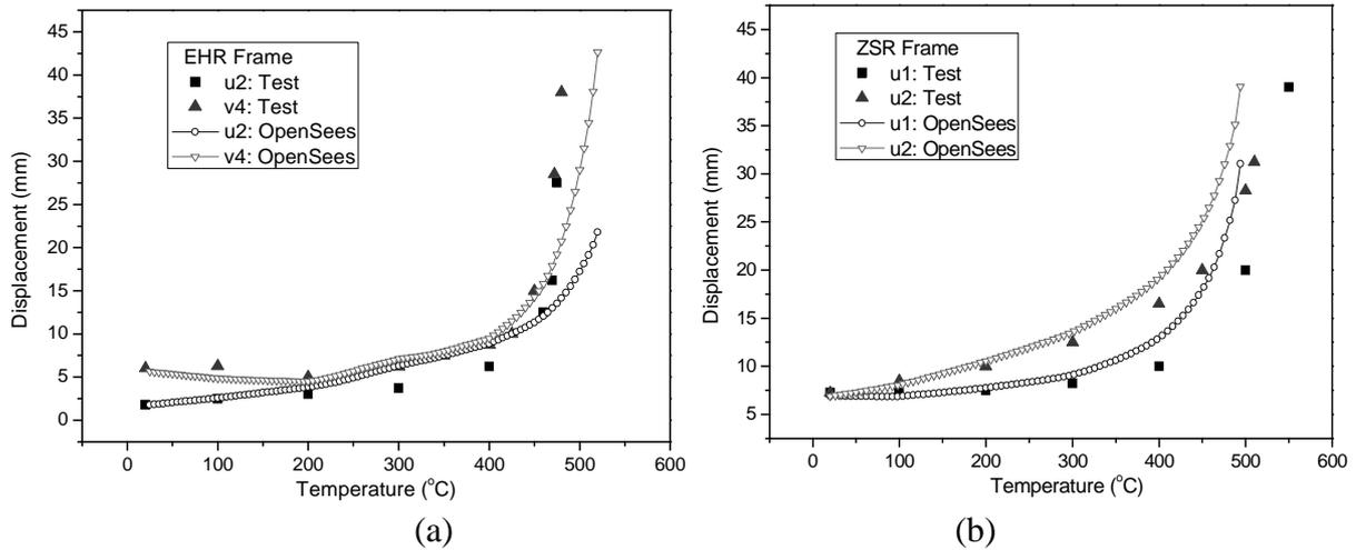
Fig. 8 Comparison between predicted and test deflection results: (a) frame EHR3; (b) frame ZSR1
