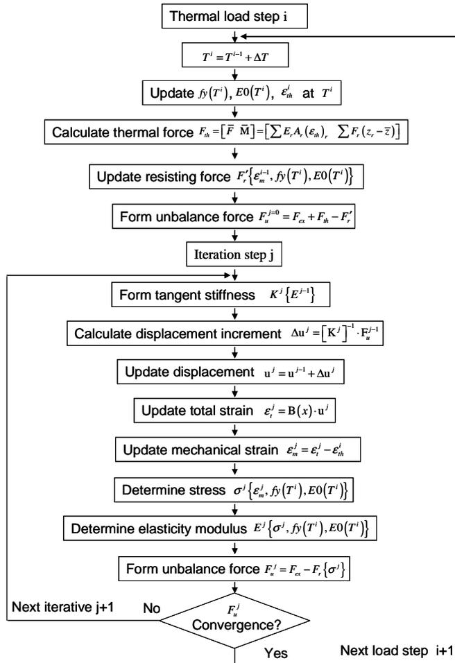
Fig. 2 Flowchart for thermo-mechanical analysis in OpenSees
