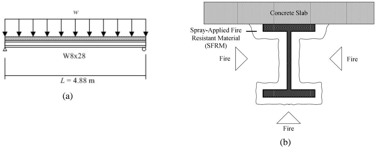
Fig. 2 Problem statement: (a) Loading and support conditions; (b) Cross-section
