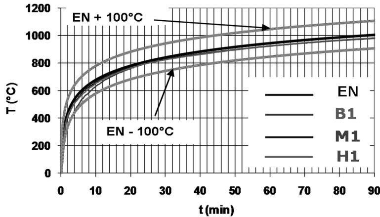
Fig. 5 Temperatures calculated by Plate Thermometers B1, M1 and H1 as function of time.
