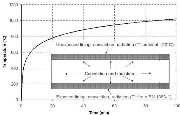
Fig. 3 Boundary conditions and thermal load for period 1
