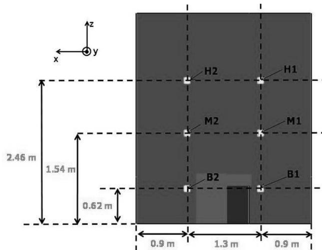
Fig. 3 Position of the plate thermometers
