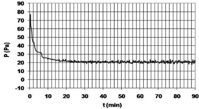
Fig. 7 Over pressure at the top of the furnace as function of time
