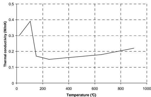
Fig. 2 Conductivity of plasterboard
