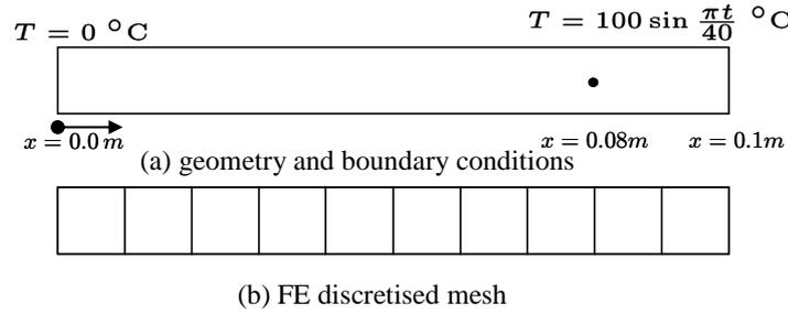
Fig. 4 Benchmark test with transient temperature boundary condition
