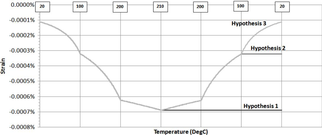
Fig. 3 Single-element implementation of USRYOU subroutine: temperature-strain plots for a constant nominal load
