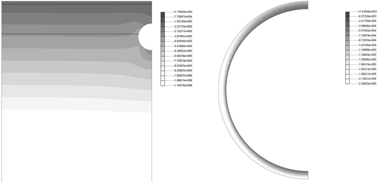
Fig. 6 Stresses in the soil and in the lining after installation of the tunnel (values in N/m<sup>2</sup>).
