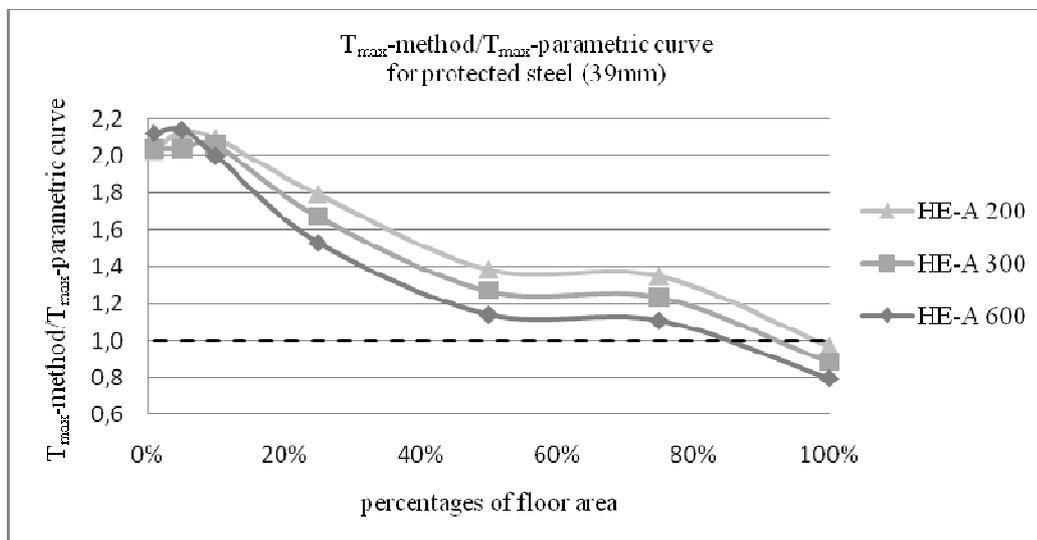
Fig. 5 Maximum steel temperature using the travelling fire method normalised by the maximum steel temperature using the parametric curve - protected steel (Jonsdottir et al. 2010).
