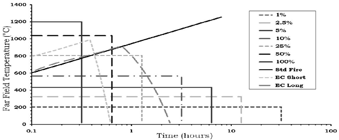
Fig. 3 Fire temperature in the family of fire sizes (Law et al., 2011)
