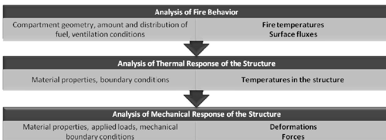
Fig. 1 Propagation of uncertainty in the structural fire simulation
