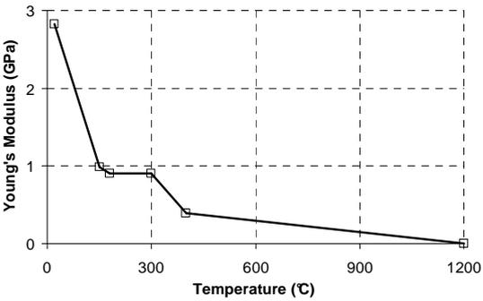
Fig. 5 Elastic modulus of plasterboard
