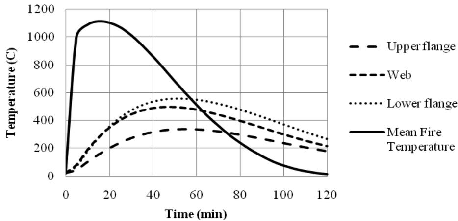
Fig. 5 Average temperatures in the steel
