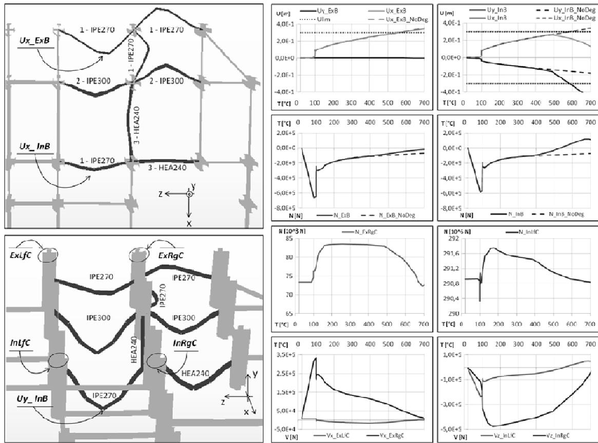
Fig. 3 Results for fire scenario 1, in term of deformed configurations, forces and displacements.
