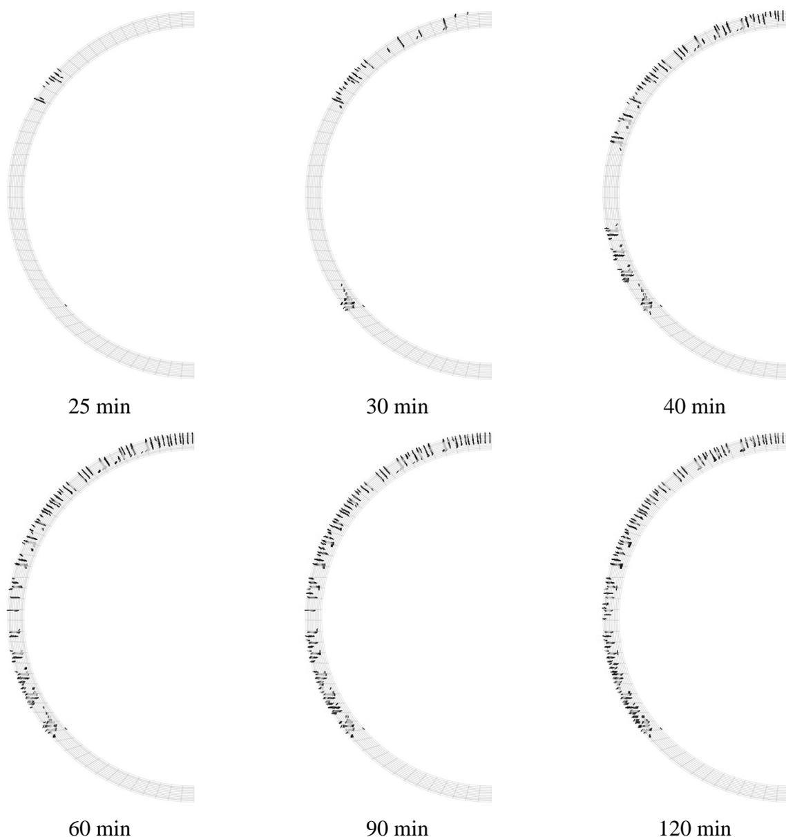
Fig. 8 Crack patterns during fire.
