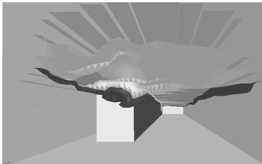
Fig. 4 Isotherms just behind the train set at 40 °C - 60 °C in the 15<sup>th</sup> minute
