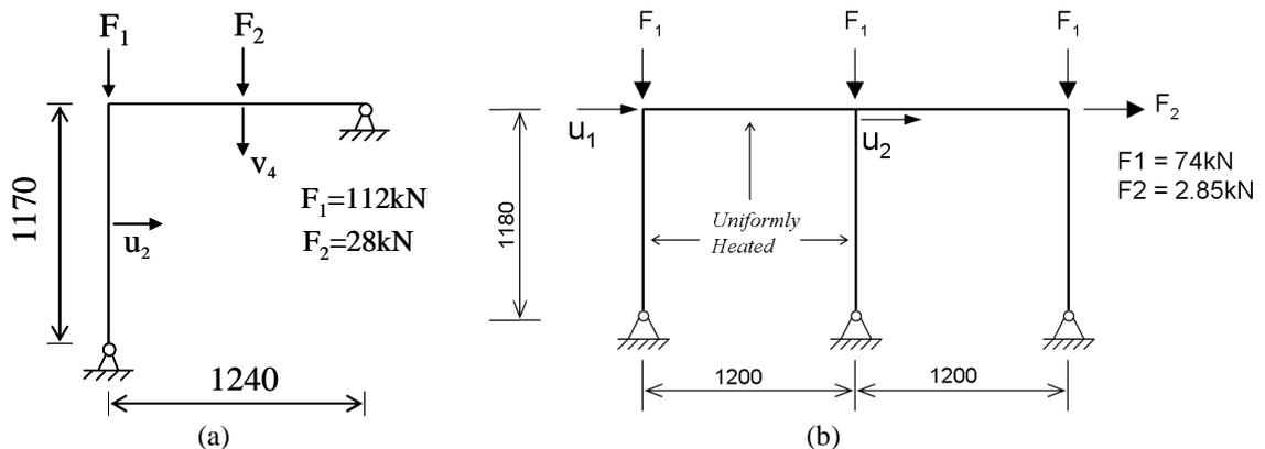
Fig. 7 Schematic of the tested steel frames (mm): (a) frame EHR3; (b) frame ZSR1
