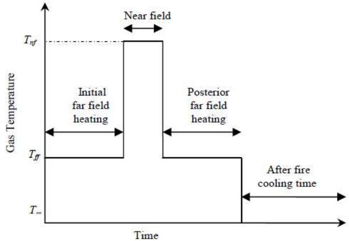
Fig 2 Temperature-time curve at one ceiling location for a travelling fire
