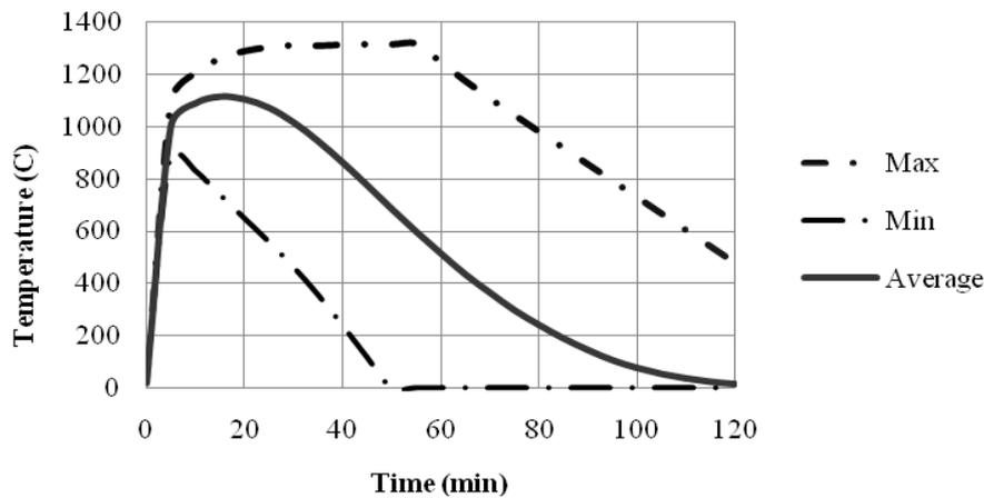
Fig. 4 Compartment temperature
