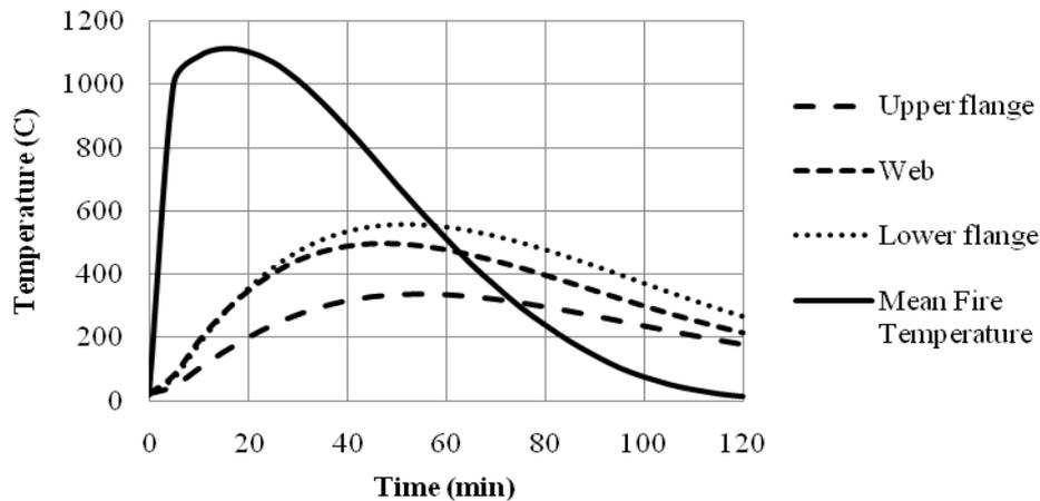
Fig. 5 Average temperatures in the steel
