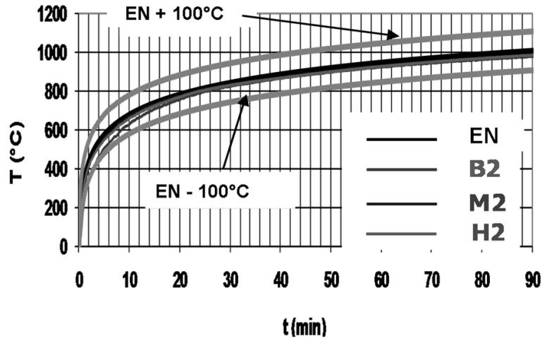
Fig. 6 Temperatures calculated by Plate Thermometers B2, M2 and H2 as function of time.
