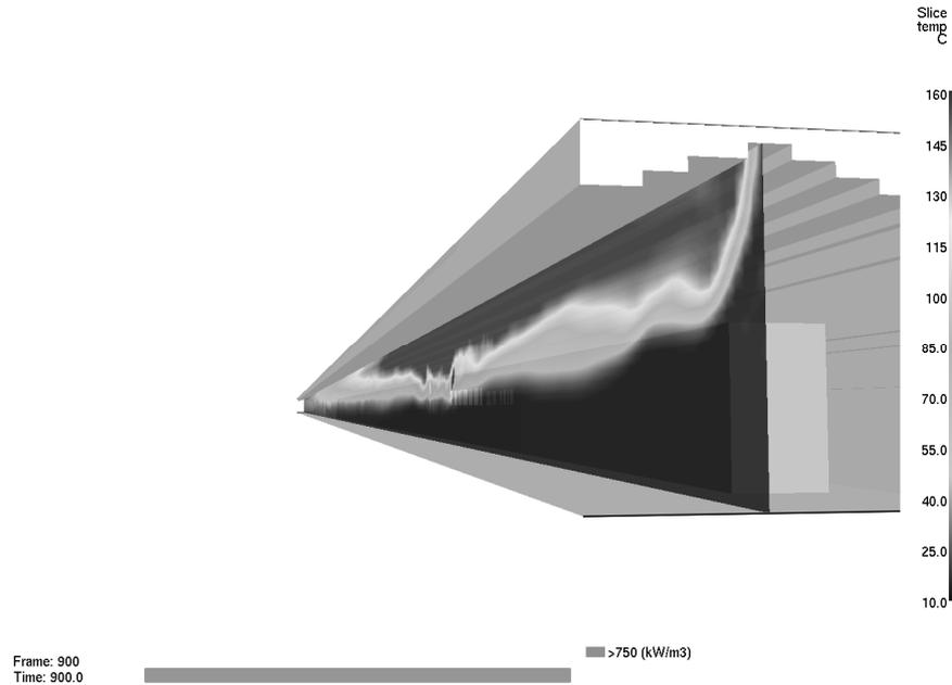
Fig. 3 Isotherm in the longitudinal cross-section of tunnel in the vicinity of fire seat in the 15<sup>th</sup> minute
