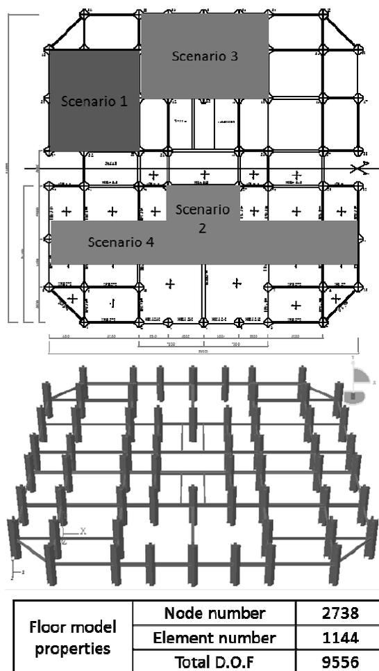
Fig. 2 floor plan FEM model and fire scenarios
