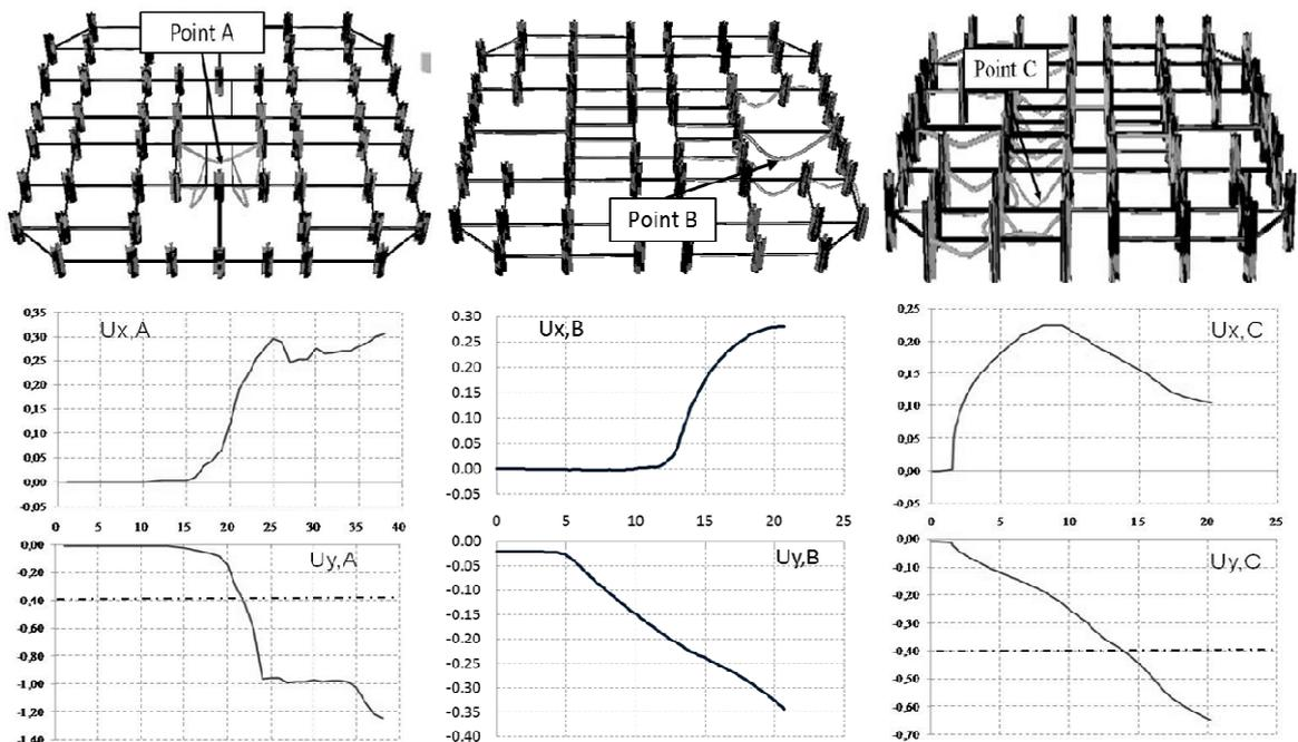
Fig. 4 Results for fire scenario 2, 3, 4 (from left to right) in term of deformed configurations (top) and trend of the horizontal and vertical displacements (in m) versus time (in min) of monitored points (bottom).
