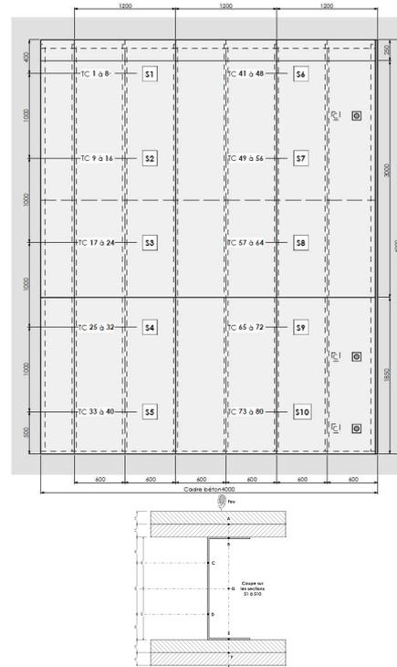
Fig. 8 Locations of the instrumentation
