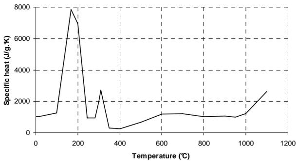
Fig. 1 Specific heat of plasterboard
