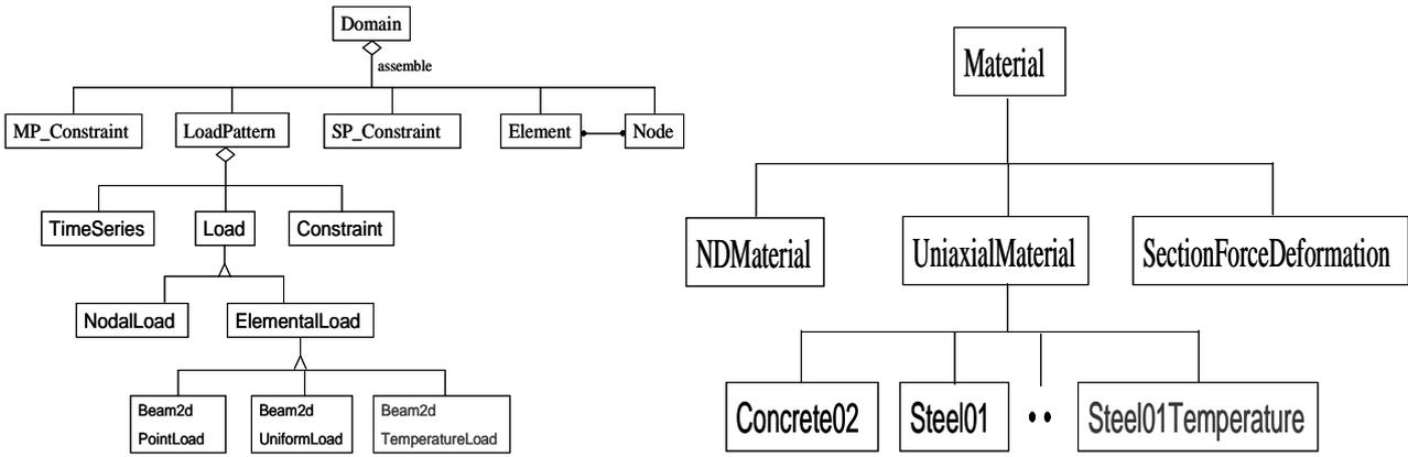
Fig. 1 Class diagram for thermal load and material in OpenSees
