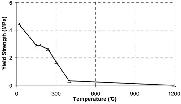
Fig. 6 Yield strength of plasterboard
