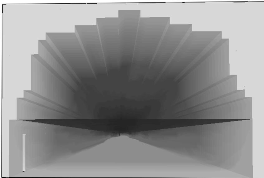
Fig. 5 Smoke layer at the entry to the escape shaft in the 12<sup>th</sup> minute
