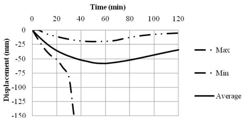
Fig. 6 Mid-span displacement
