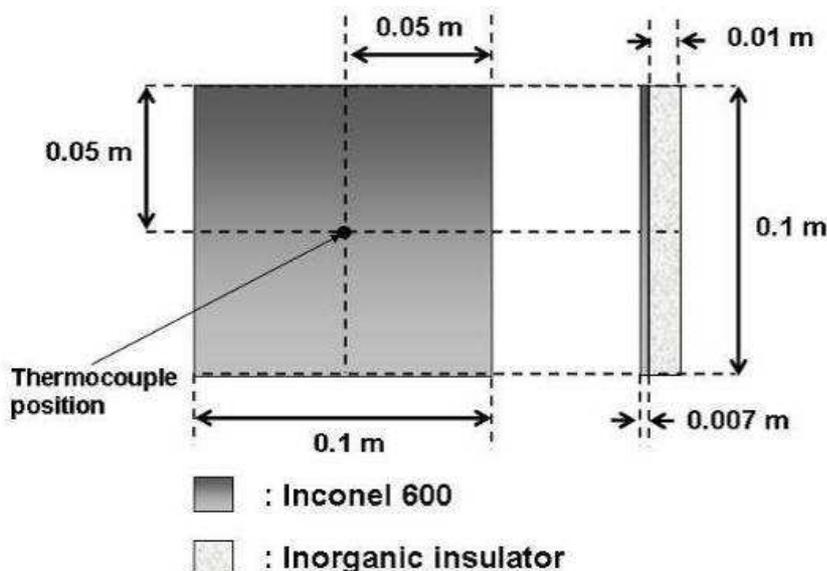
Fig. 2 Outline of the plate thermometer structure
