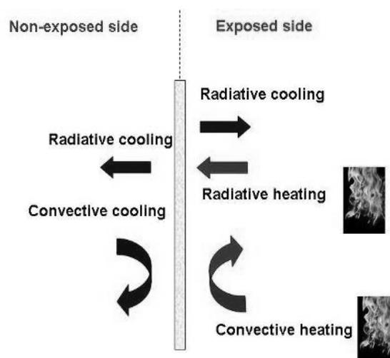
Fig. 4 Heat flux at the exposed and non-exposed sides of the tested element.
