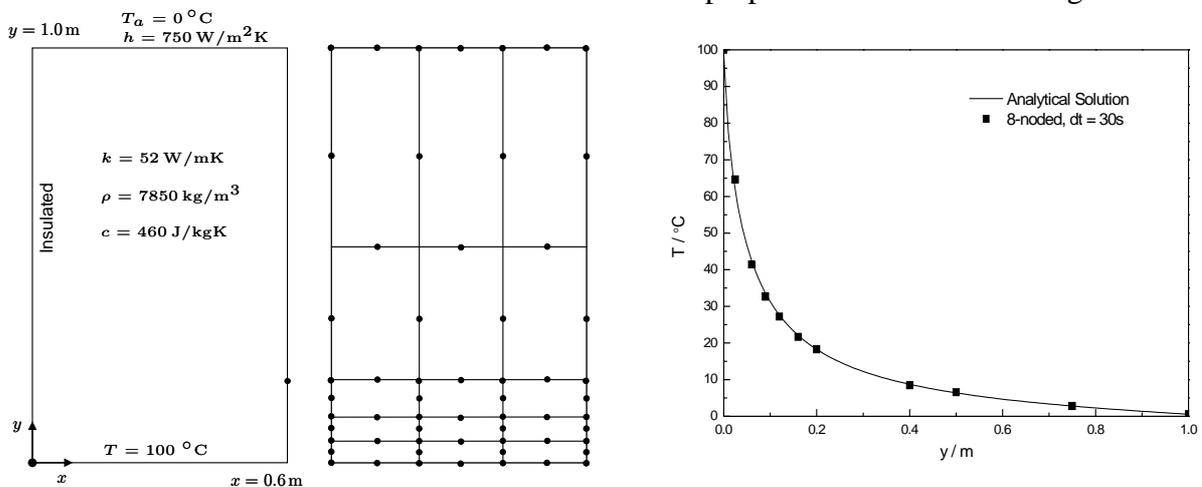
Fig. 7 Benchmark test with convection boundary condition Fig. 8 Temperature distribution along right-side boundary
