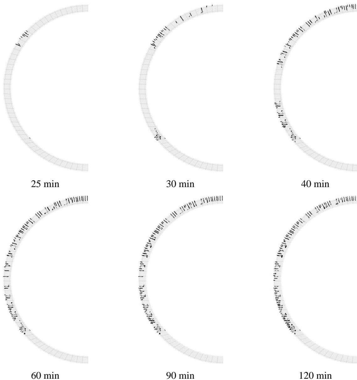
Fig. 8 Crack patterns during fire.
