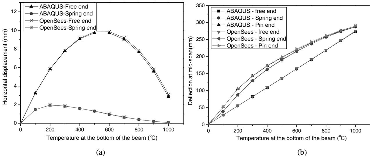
Fig. 5 Displacement of beam with different translational end restraint: (a) Horizontal displacement; (b) mid-span displacement
