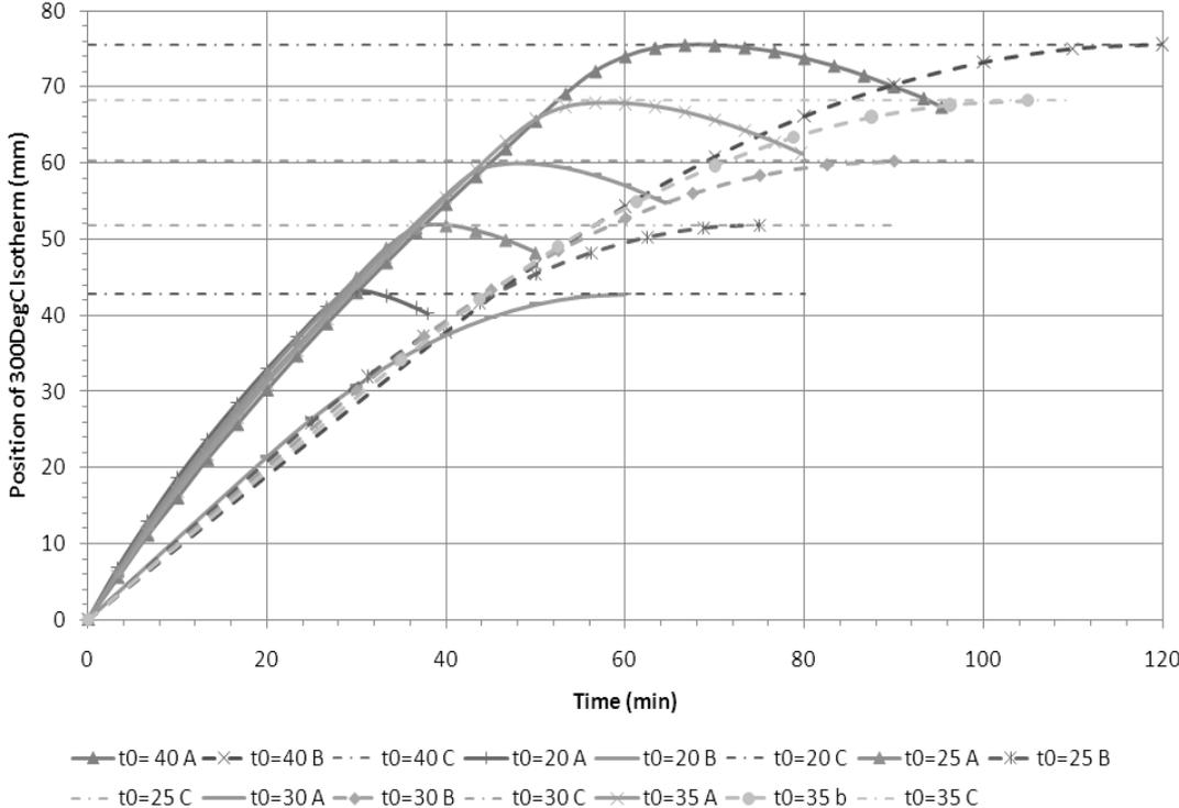
Fig. 3 Position of 300°C isotherm using modified  $k_{qtd,mod}$  (A) and EN 1995-1-2 Annex A (B). Target depth of char shown as (C).
