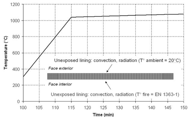
Fig. 4 Boundary conditions and thermal load for period 2
