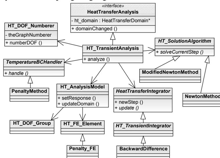
Fig. 3 Class diagram representing heat transfer analysis algorithms
