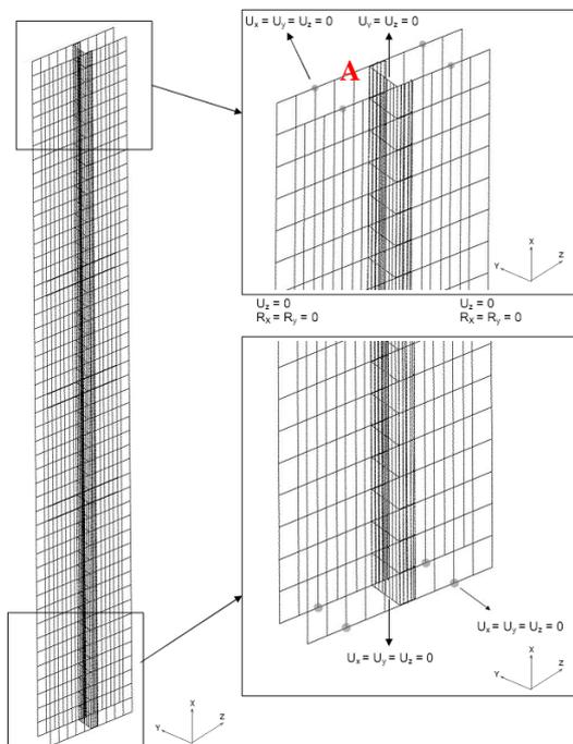
Fig. 13 Mesh and boundary condition
