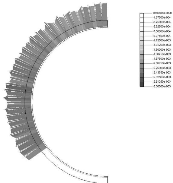
Fig. 11. Plastic strains in the reinforcement.
