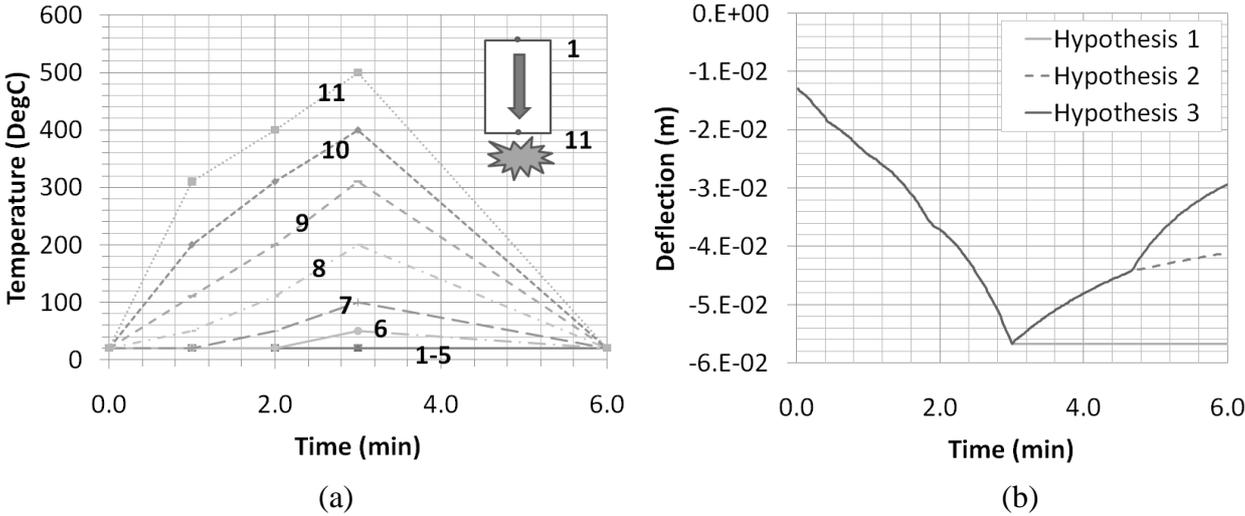
Fig. 4 Beam implementation of USRYOU and USRCST/TST subroutines: (a) Temperature profiles at integration points (b) Deflection–time plots.
