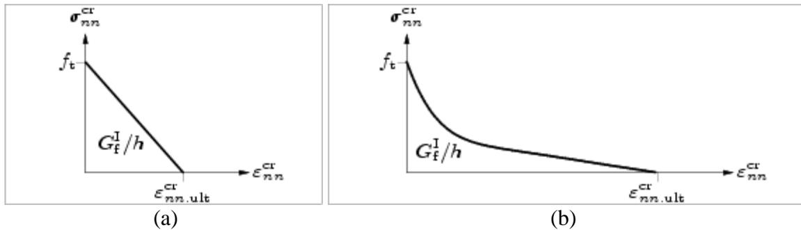
Fig. 2 Tension-softening relationships available in DIANA (Manie 2010):- linear (a) and Hordyk (b)
