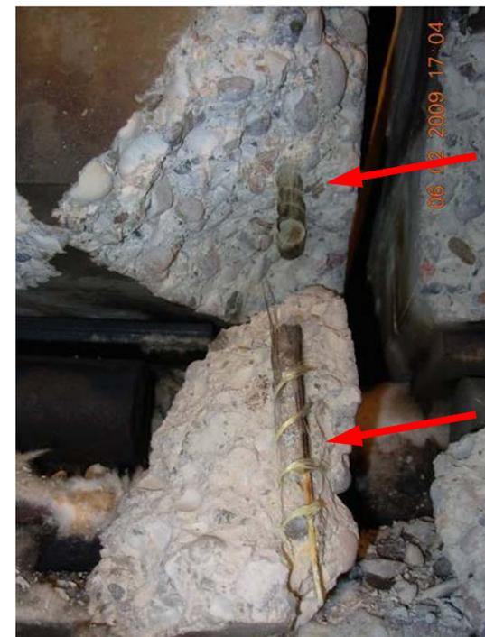
ADHESION AT HIGH TEMPERATURE OF FRP BARS STRAIGHT OR BENT AT THE END OF CONCRETE SLABS
