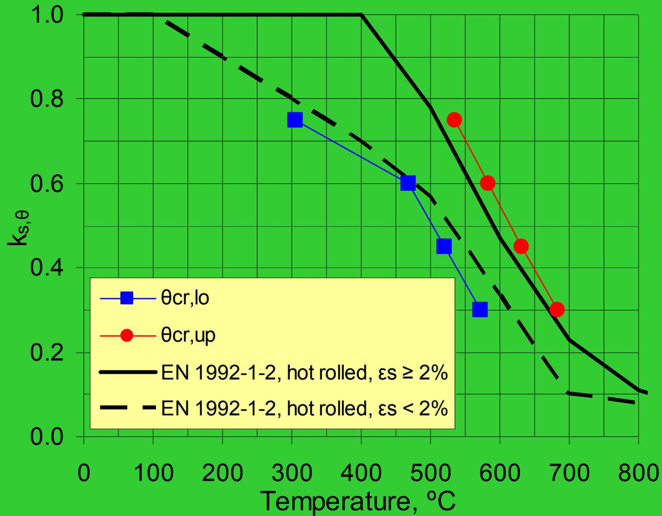
Steel strength reduction factor ( $k_{s,\theta} = f_{y,\theta}/f_{yk}$ )
