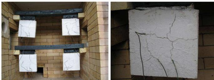
Fig. 3 Reaction of spray coating in fire
