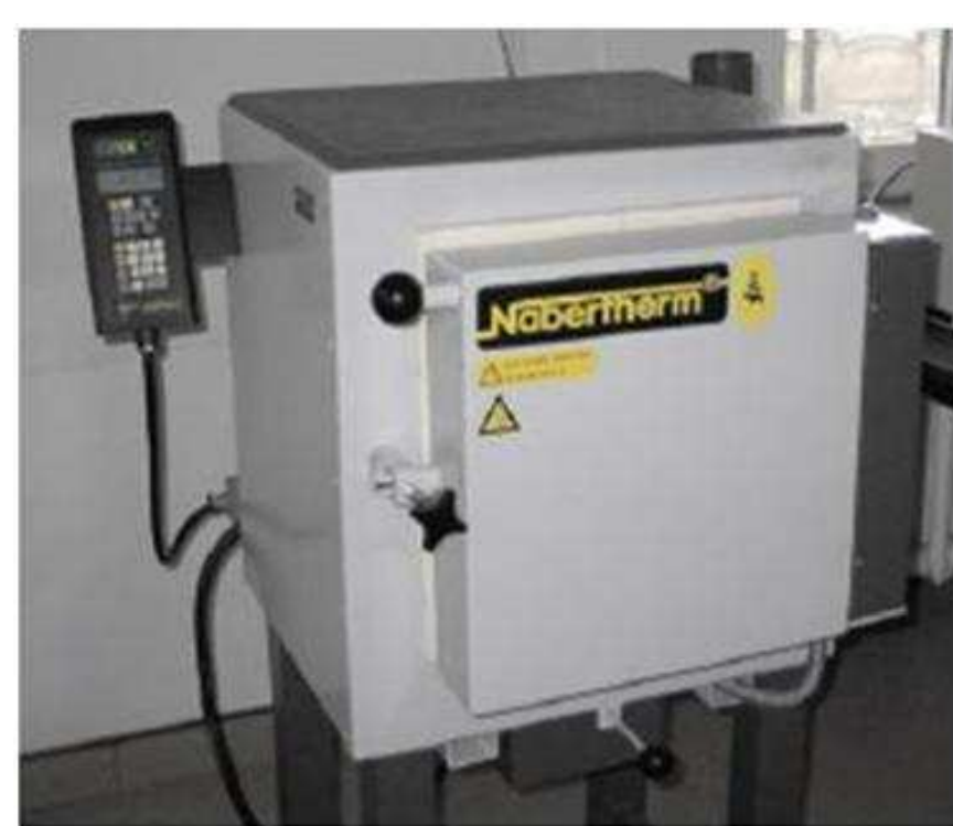
Concrete samples heating
