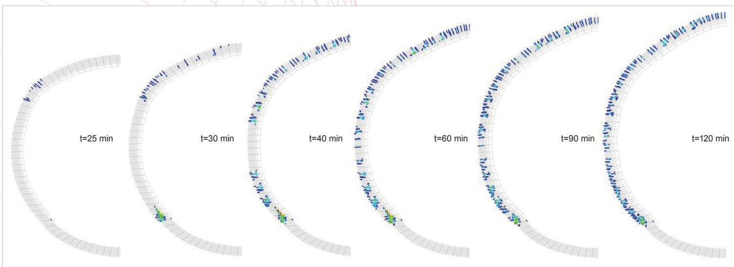
Equivalent plastic strains in concrete (left) and plastic strains in the reinforcement at the intrados (right)
