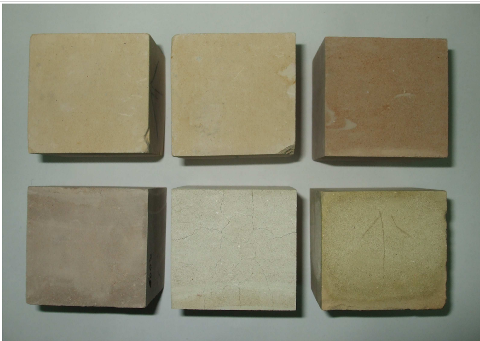
Fig. 4 Discolouration of Globigerina limestone Samples from top left to right, bottom left to right: yellow 100°C; yellow 200°C; reddish-brown 400°; grey 600°C; white 800°C; grey-white 1000°C
