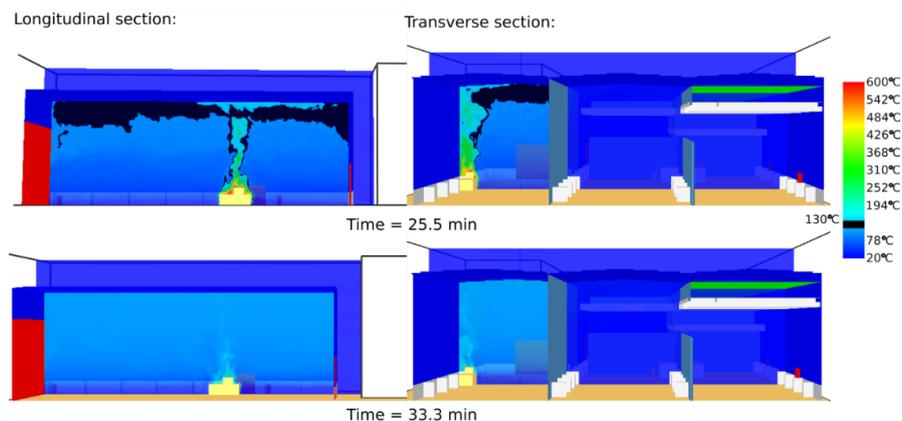
Figure 6–6 Gas temperature distributions in longitudinal and transverse cross-sections.
