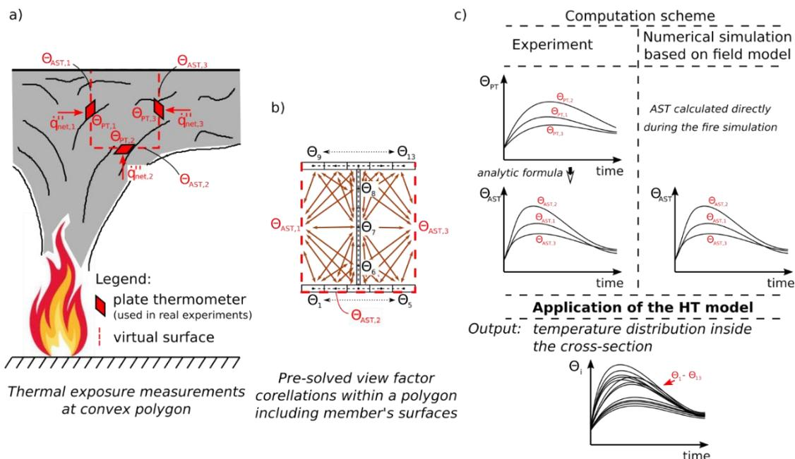
**Figure 3–15** Visual representation of connection between the heat transfer approach, experiments and numerical simulations: a) visualization of the polygon inside the fire compartment that consists of virtual surfaces, b) co-radiating surfaces and temperature points inside the cross-section, c) computation scheme.
