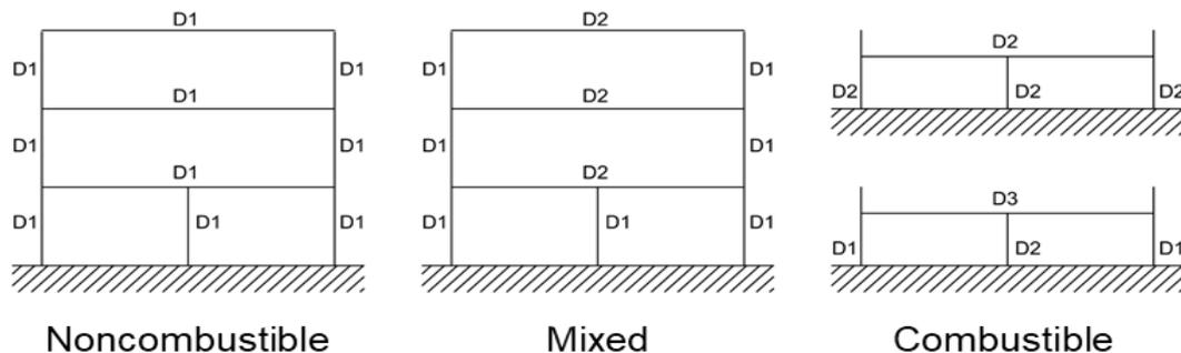
Figure A-5 Classification of construction system types
