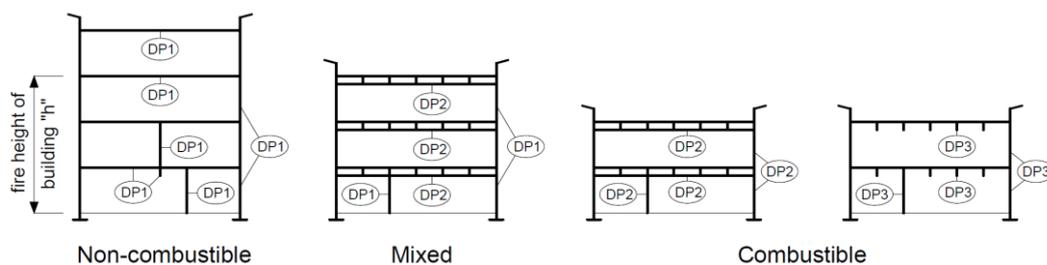
Figure A-1 Classification of construction system types
