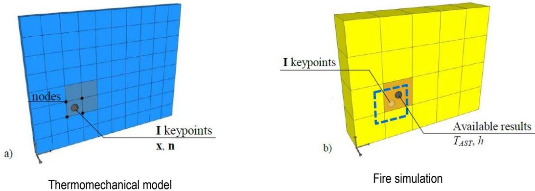
Figure 4–3 Illustration of the exposed surfaces and the mapping procedure.
