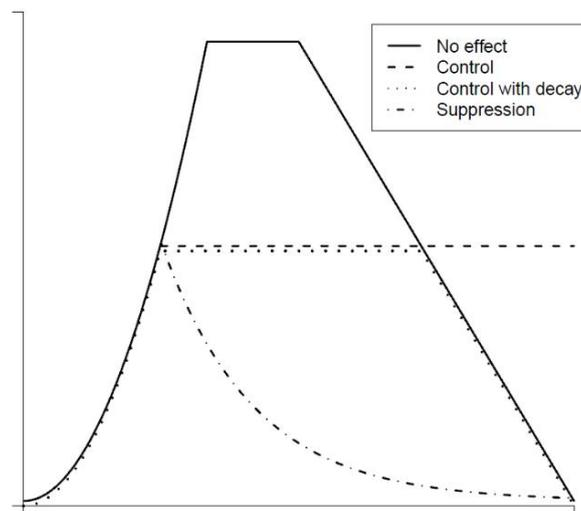
Figure 2-9 Typical heat release rates of sprinkler controlled fire scenarios. For fire modelling, controlled fire scenarios are used at normal sprinklers, suppression effect is accepted only at ESFR sprinkler nozzles.
