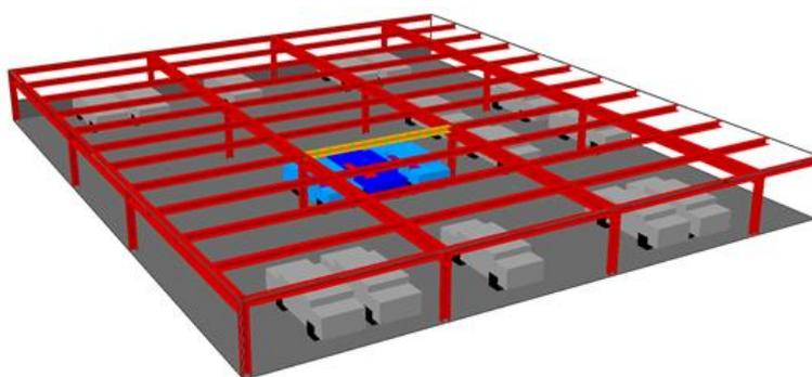
**Figure 6-32** Visualisation of fire simulation in Fire Dynamics Simulator – analysed beam highlighted.
