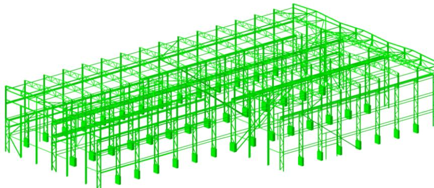
Figure 6–4 Plot of a 3D Abaqus model of the structure (beams' cross-section rendered).
