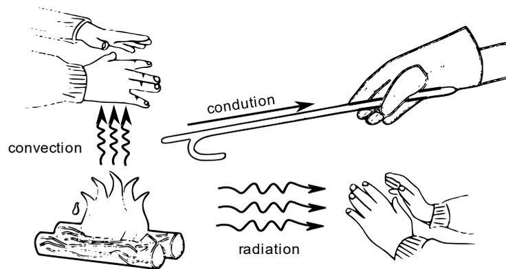
Figure 3–2 Illustration of the three fundamental heat transfer mechanisms
