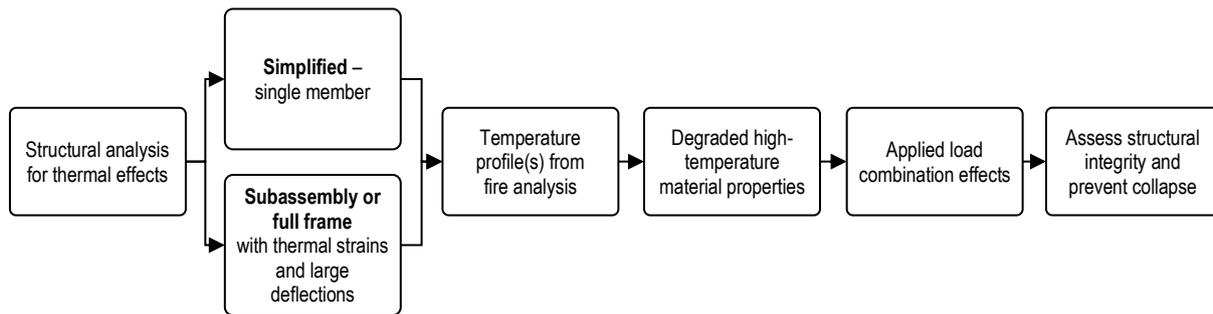
Figure 4–1 Schematic of structural analysis for fire effects, adapted from ch. 52 of [15].
