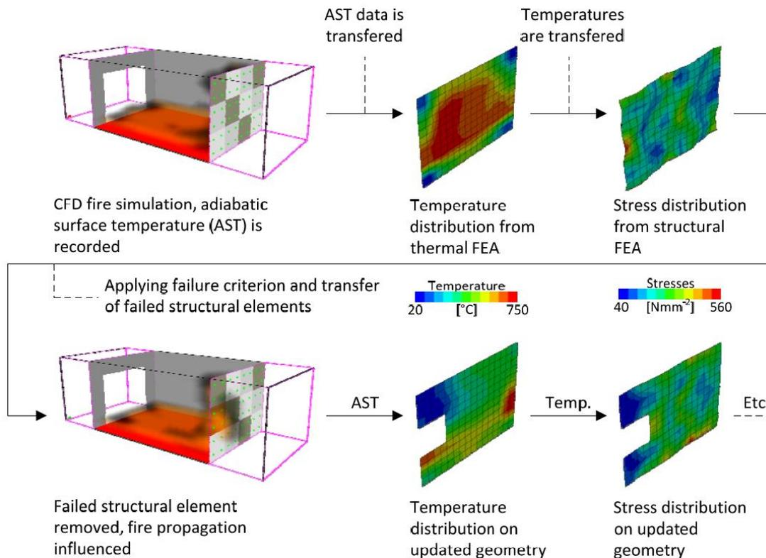
Figure 4–4 Two-way coupled fire to thermomechanical analysis using a stress-based failure criterion [38].
