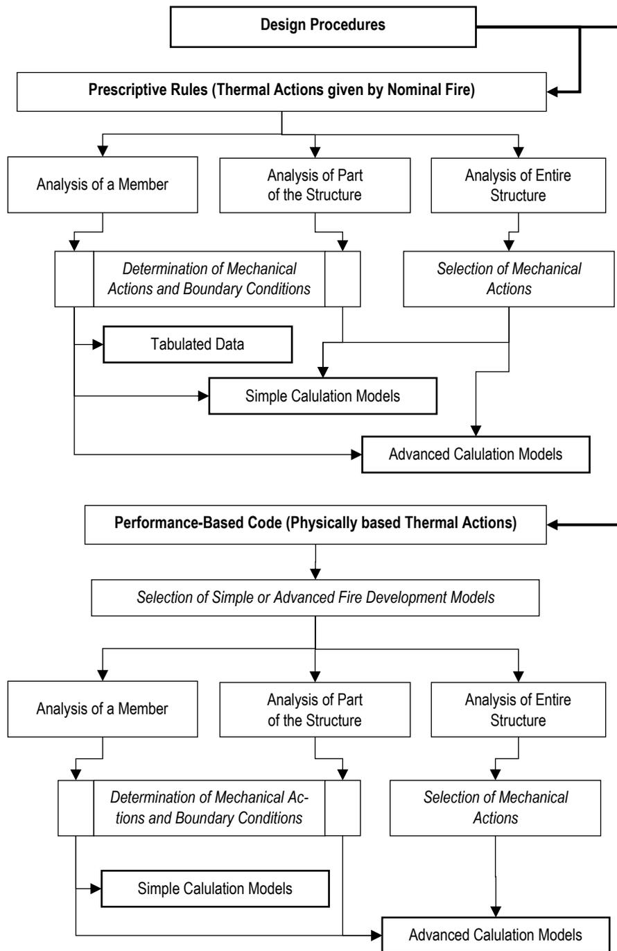
Figure 1–2 Alternative design procedures (according to Eurocode 1991-1-2)
