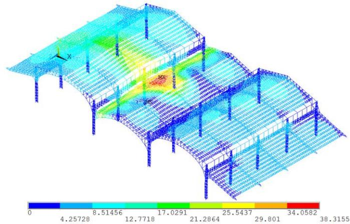
**Figure 6–26** The deformation of the steel structure of the example fire scenario.
