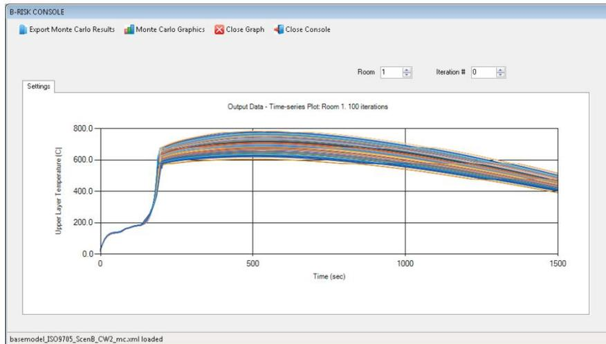
**Figure 2–5** Example time series plot of upper layer temperature for multi-iteration output [11].
