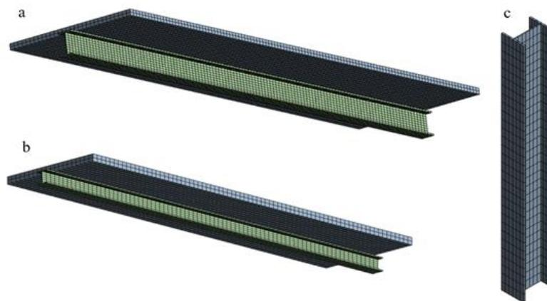
**Figure 6–38** Models of structural elements in ANSYS – a) girder, b) beam, c) column.
