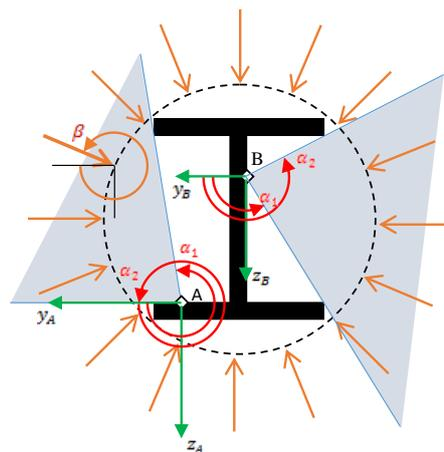
**Figure 3-12** Geometrical visualization of view angles  $\alpha_1$  and  $\alpha_2$  for an example of points A and B and corresponding angle of radiation vector  $\beta$ .
