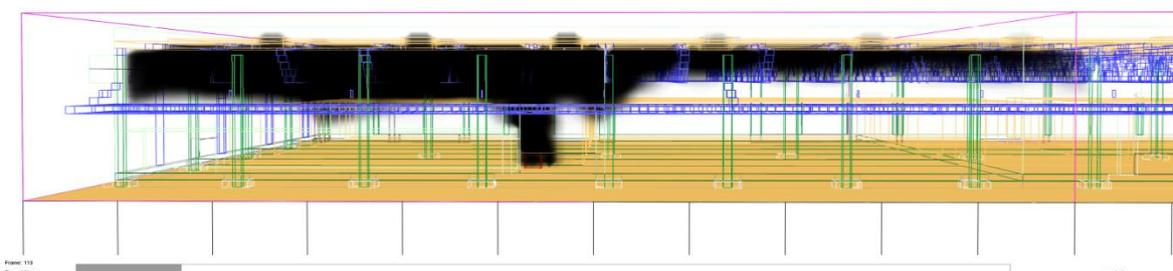
**Figure 6–20** Smoke spread at the end of a fire detection alarm time and evacuation time.
