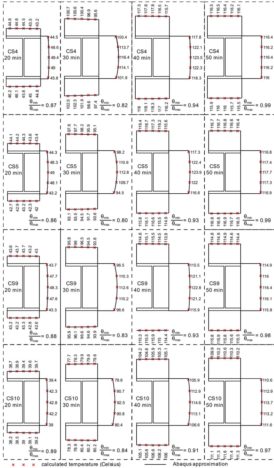
Figure 6-9 Temperature profiles at selected I-sections in a design fire and Abaqus approximation.
