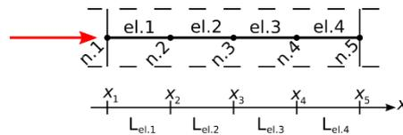
**Figure 3–10** An exemplary 1D heat transfer problem. Domain discretized into 4 finite elements, the external heat flux is applied to node number 1.
