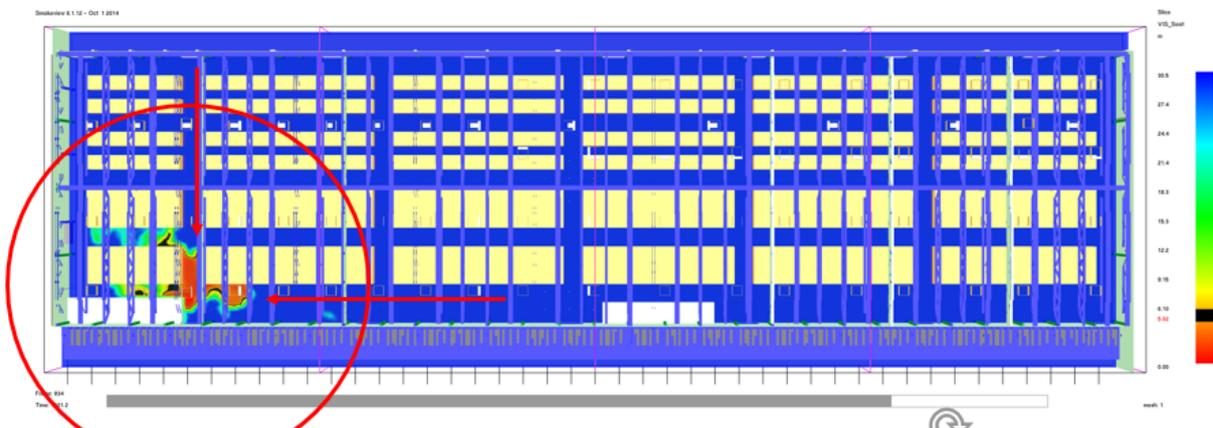
Figure 6–22 The length of visible route on a 2 m high plane at the beginning of the fire fighting intervention in the large set scene storage of the Opera Workshop Centre. The red circle connotes a 25 m radius. The red arrows indicate the possible directions of intervention.
