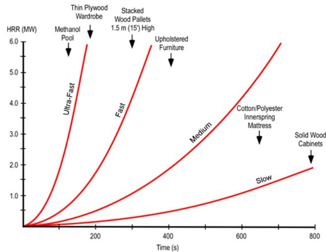
Figure 2-8 Growth phase of fire scenarios with different coefficients.
