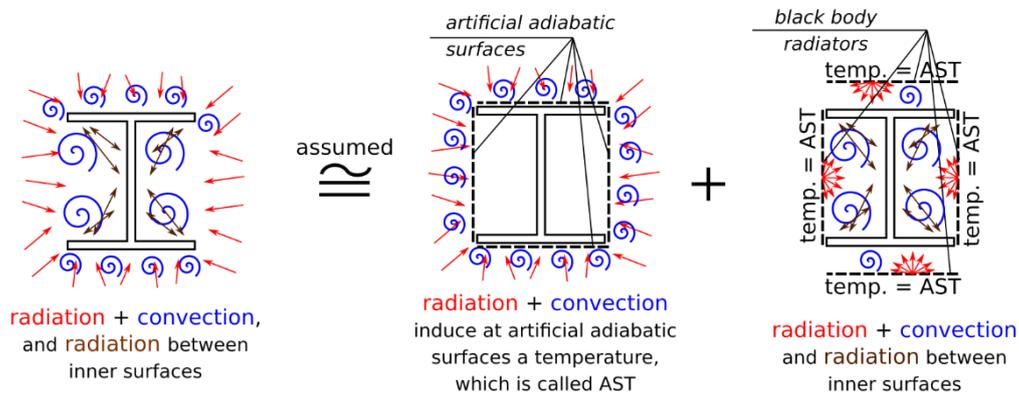
**Figure 3–14** The idea behind the heat transfer approach for a thin-walled cross-section that uses AST:
