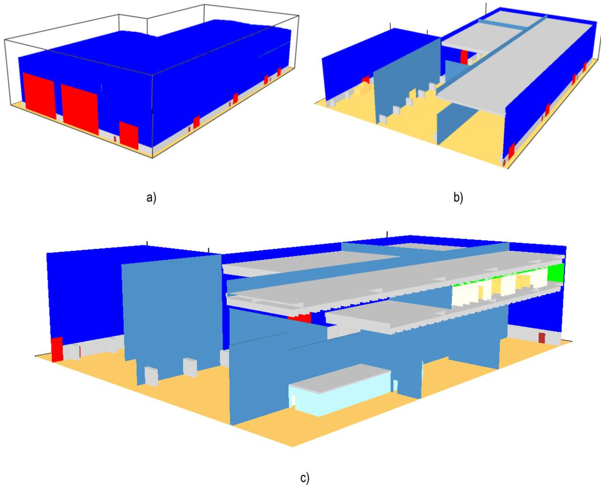
**Figure 6–3** Plot of CFD model: a) external view, b) and c) cross-sections.
