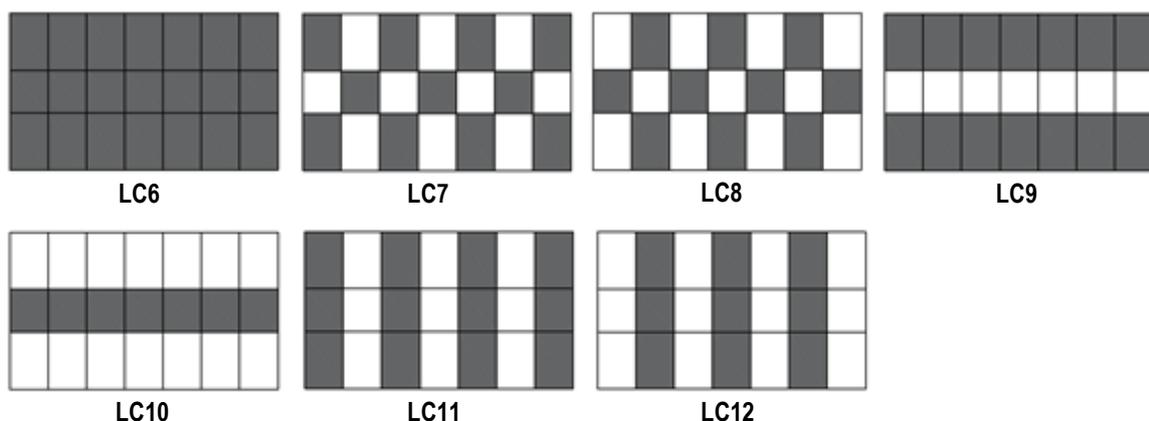
**Figure 6–36** Forms of a checker pattern arrangement of the applied surface traffic load with respect to the axis of the main bearing elements.
