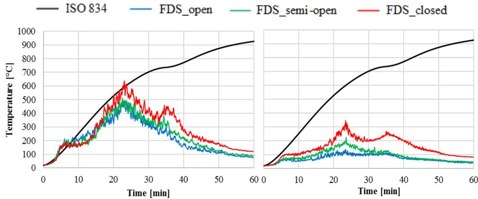
**Figure 6–33** Obtained steel beam surface temperatures in middle section (left) and end beam section (right).
