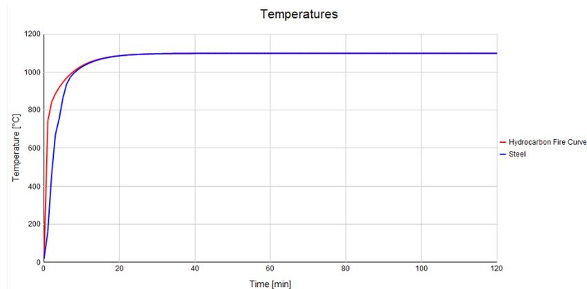
Figure 2–6 Example output from Ozone – Time vs. Gas and Steel profile temperatures.
