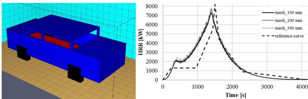
Figure 6–30 Geometry of modelled car (left) and mesh sensitivity analysis (right).
