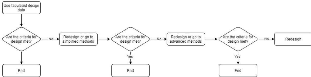
Figure 1–3 Design flowchart for the use of three level of methods in the Eurocodes
