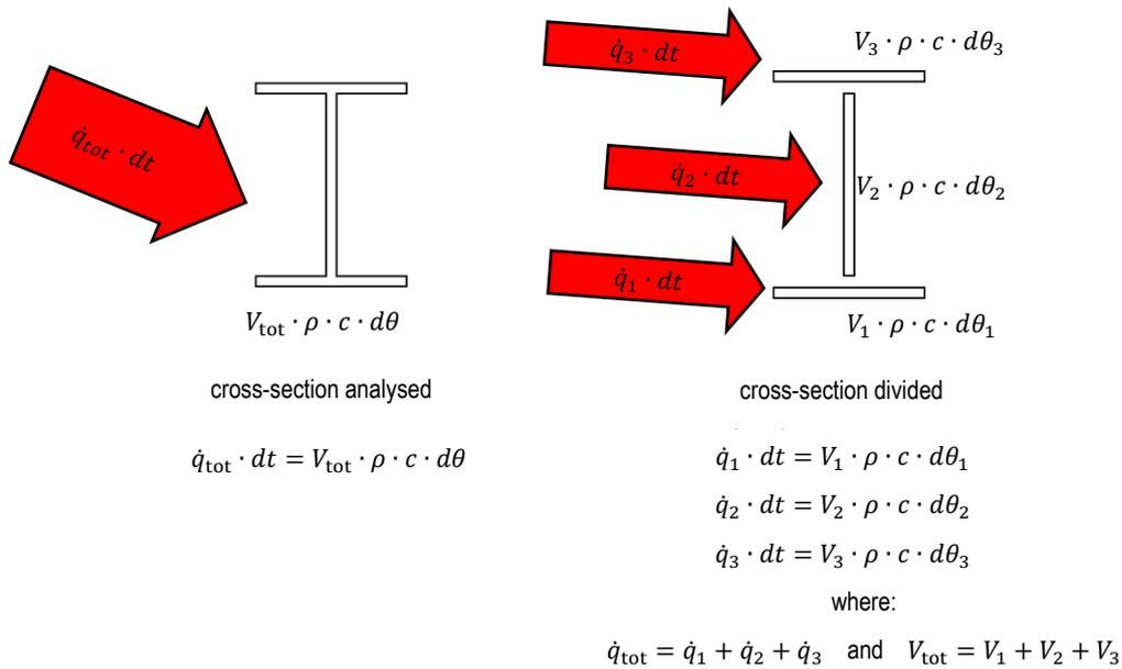
**Figure 3-7** Heat balance expressions for a cross-section analysed using the lumped heat capacitance model, analysed as a whole and divided into three components
