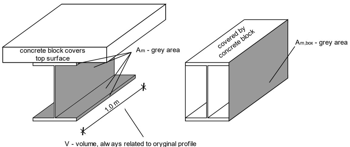
Figure 3–9 Interpretation of  $A_m$ ,  $A_{m,b} = A_{m,box}$ ,  $V$  for a cross-section exposed for fire from 3 sides.
