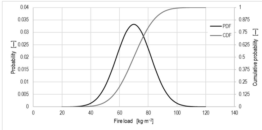
Figure 5–1 Exemplary PDF and CDF of an arbitrary fire load following normal distribution:  $\mu = 70 \text{ kg}\cdot\text{m}^{-2}$ ,  $\sigma = 12$ .
