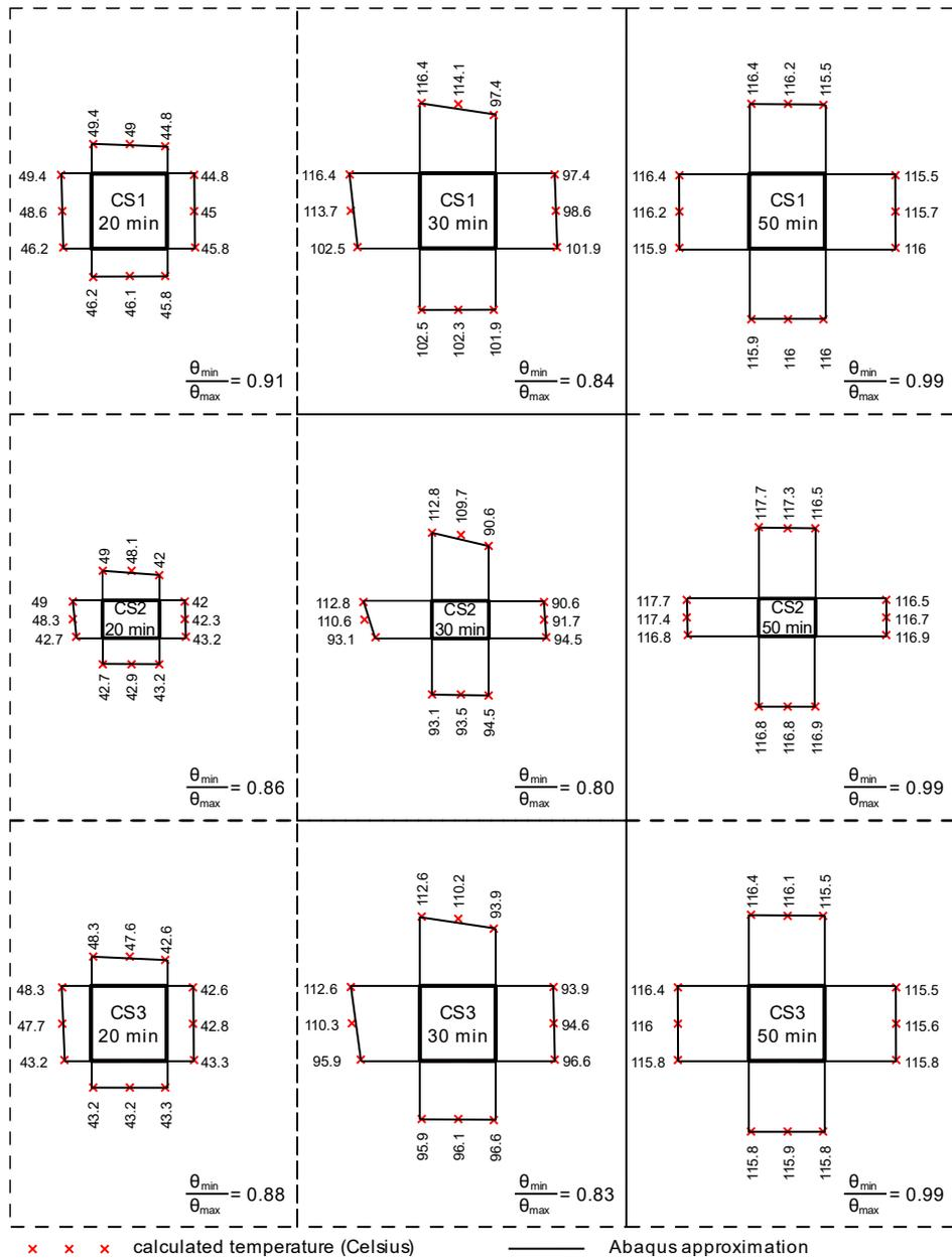
Figure 6-8 Temperature profiles at selected BOX-sections in a design fire and Abaqus approximation.
