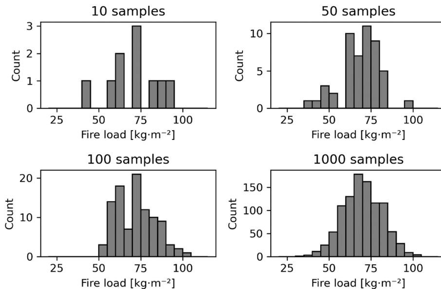
Figure 5–2 Example of simple random sampling from the arbitrary fire load distribution:  $\mu = 70 \text{ kg}\cdot\text{m}^{-2}$ ,  $\sigma = 12$ .
