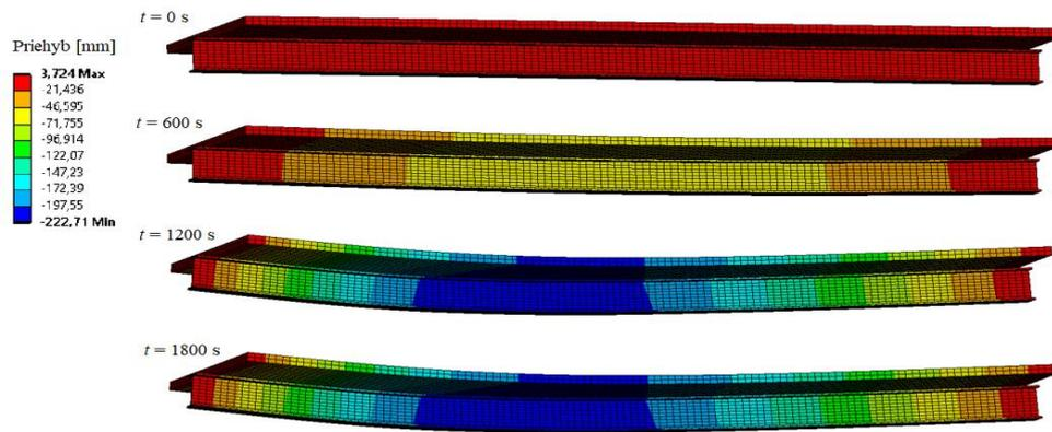
Figure 6–39 Example of the development of girder deflection under thermal exposure – scenario 2P.
