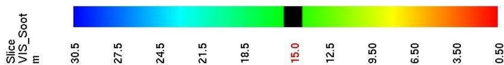
**Figure 6–17** Visibility scale at the evacuation period. Blue colour means a better visibility, while red does the worse from 0 to 30 m.
