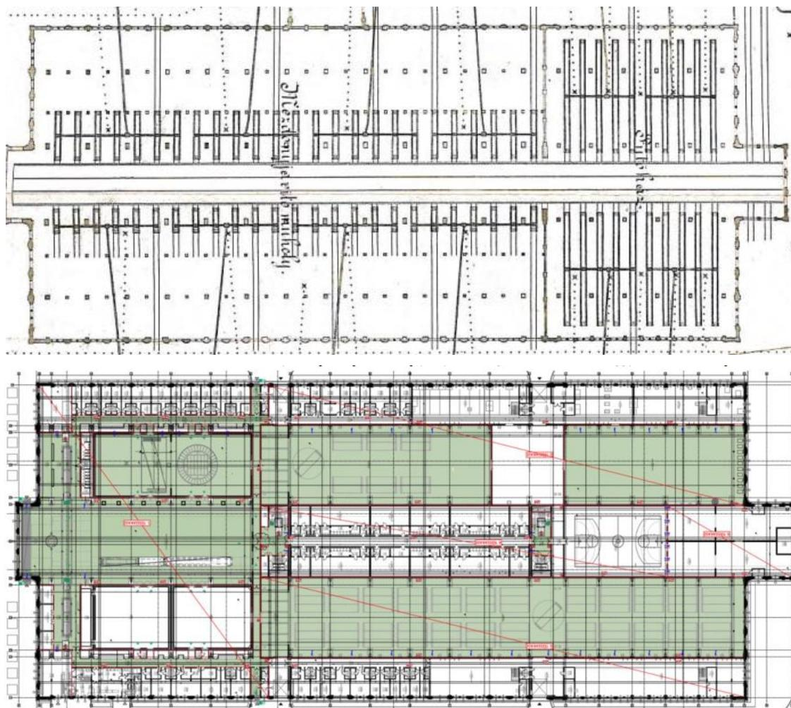
Figure 6-15 The original floor plan drawing of the hall [64], and the new layout.
