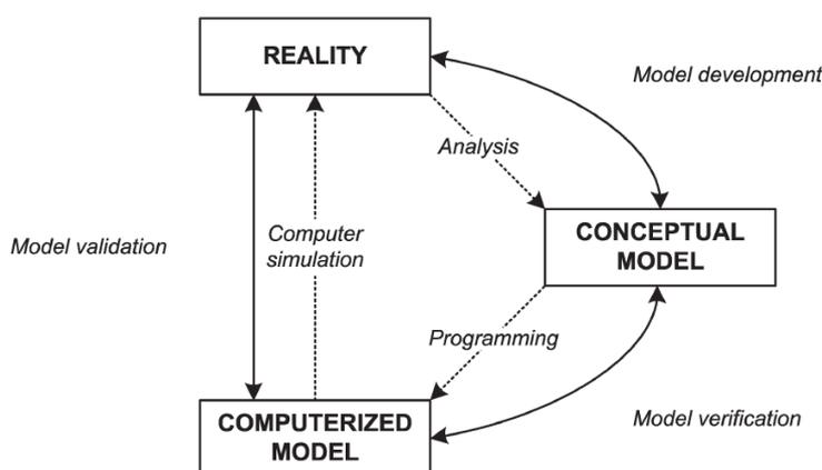
Figure 5–3 Conceptual representation of model verification and validation [52].
