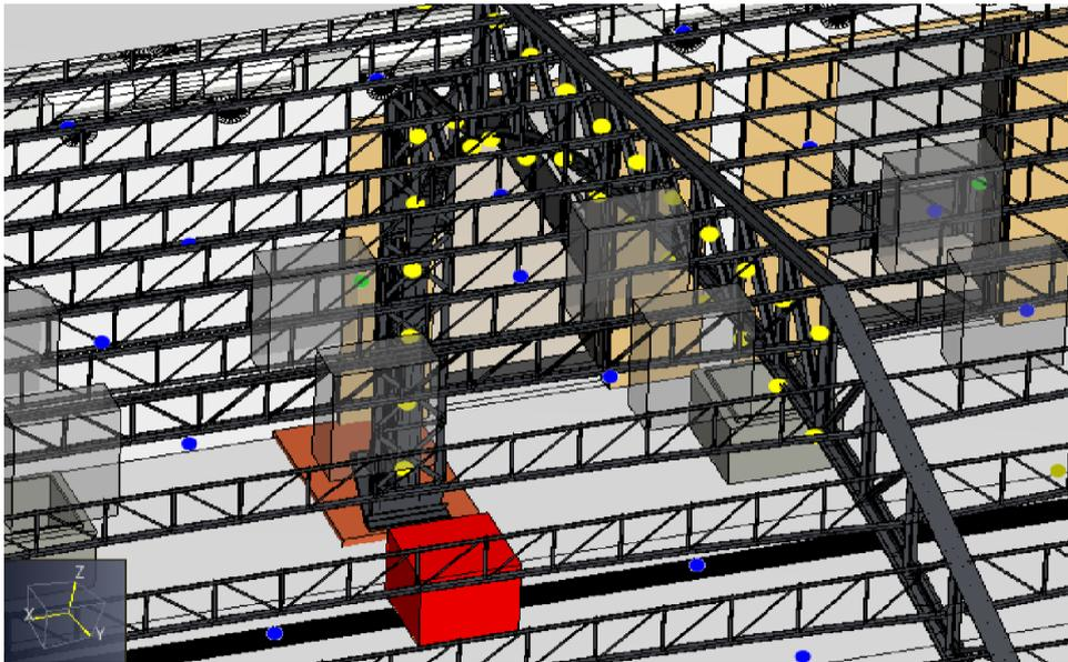
Figure 6-23 Temperature measuring devices around the structure over a fire scenario.
