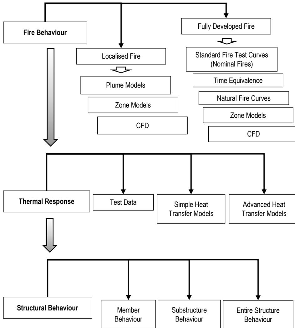
**Figure 1–1** Available methods to define the Fire Behaviour, Thermal Response and Structural Behaviour
