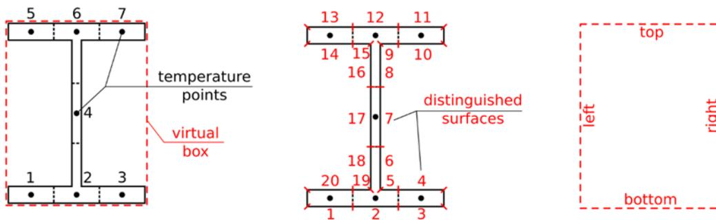
**Figure 3-16** Cross-section divided into 7 parts and corresponding: 7 temperature points, 15 surfaces at section edges, 4 surfaces of receiving envelope.
