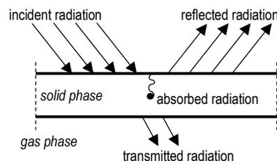
Figure 3-3 Effects of incident radiation on fluid-solid surface
