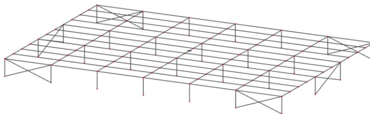
**Figure 6-34** Beam structural model of one floor of parking house.
