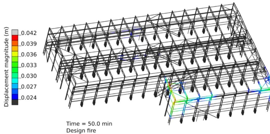
Figure 6-12 Displacement development at time 50 min for structure exposed to design fire.
