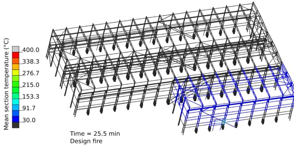
Figure 6–10 Mean section temperatures for the structure exposed to design fire at time 25.5 min.
