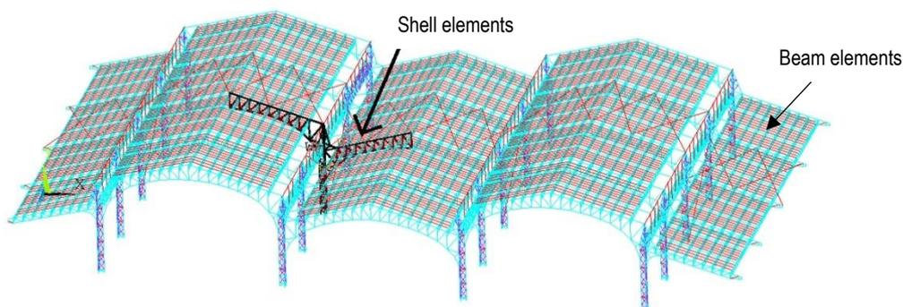
Figure 6-24 The combined shell-beam model in ANSYS.
