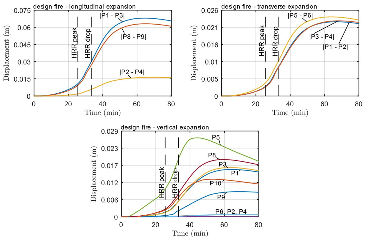
Figure 6-13 Longitudinal, transverse, and vertical expansion measured between selected points (see Figure 6-11).
