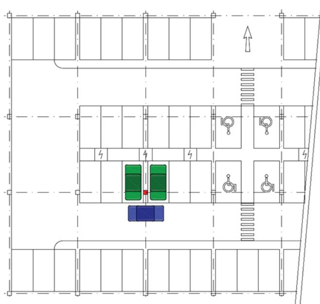
**Figure 6-31** An example of a fire scenario for CFD fire modelling.
