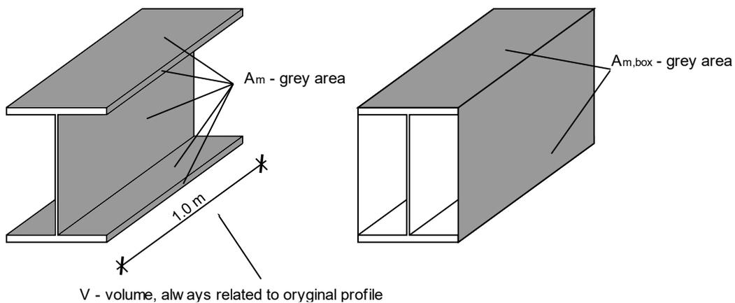
Figure 3–8 Interpretation of  $A_m$ ,  $A_{m,b} = A_{m,box}$ ,  $V$  for a cross-section exposed for fire from 4 sides.
