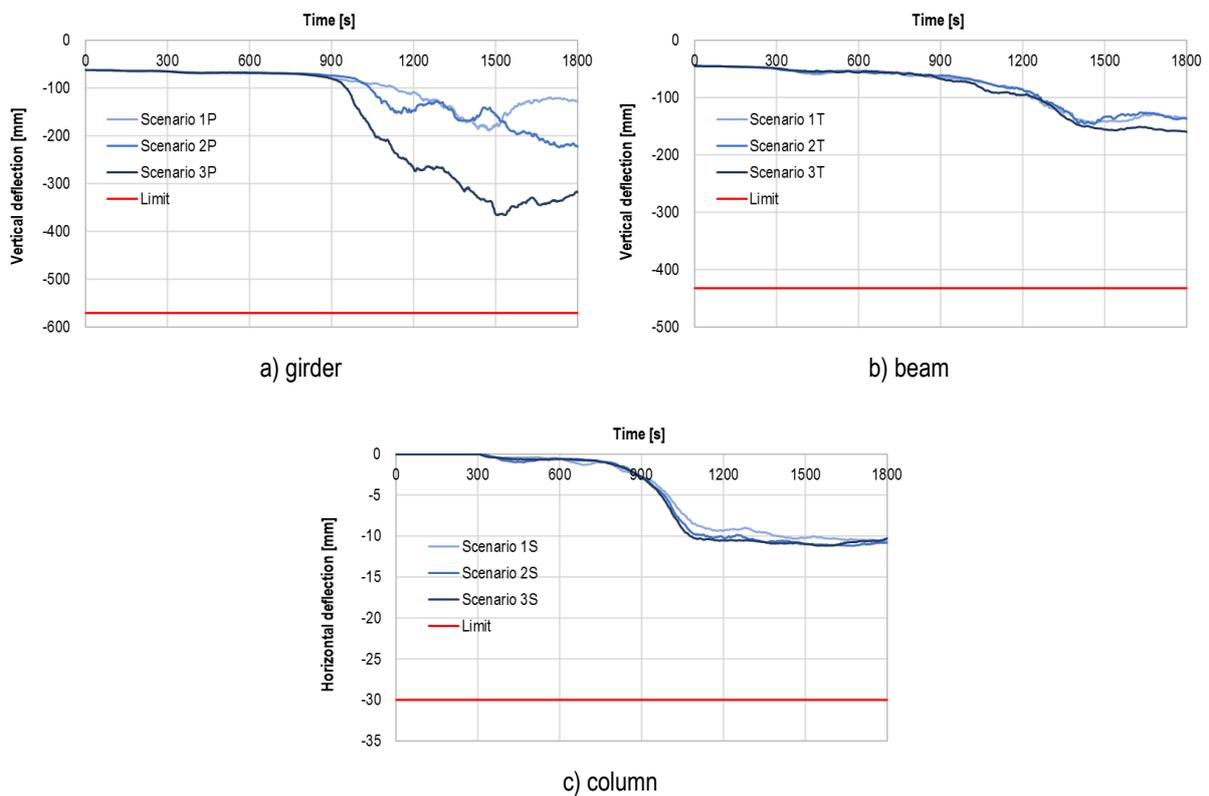
Figure 6–40 Structural modelling results – deformation – for the analysed construction members.
