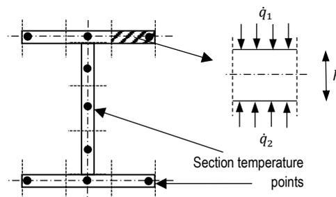
Figure 3–13 Section temperature points and related heat fluxes  $\dot{q}_1$  and  $\dot{q}_2$ .
