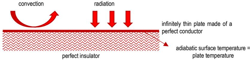
Figure 3-5 Physical model of an adiabatic surface
