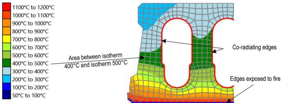
Figure 3–18 Representation of exact fire exposure and reciprocal radiation in section's voids on the example of concrete slab.
