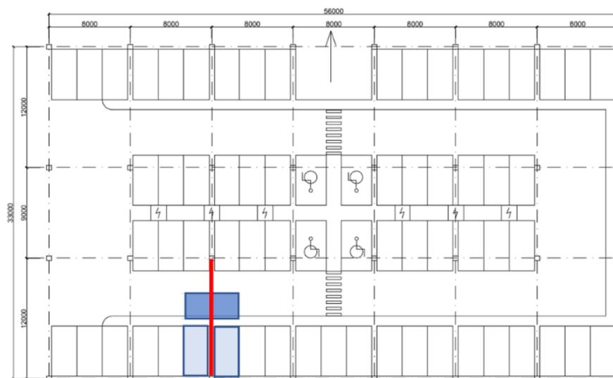
Figure 6-29 Floor plan of designed carpark with burning cars and analysed beam position.
