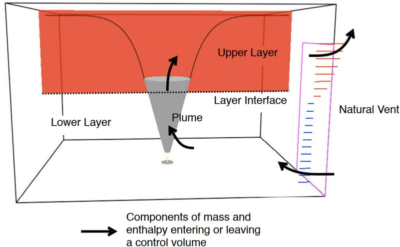
**Figure 2-2** Schematic of control volumes in a two-layer zone model [8].
