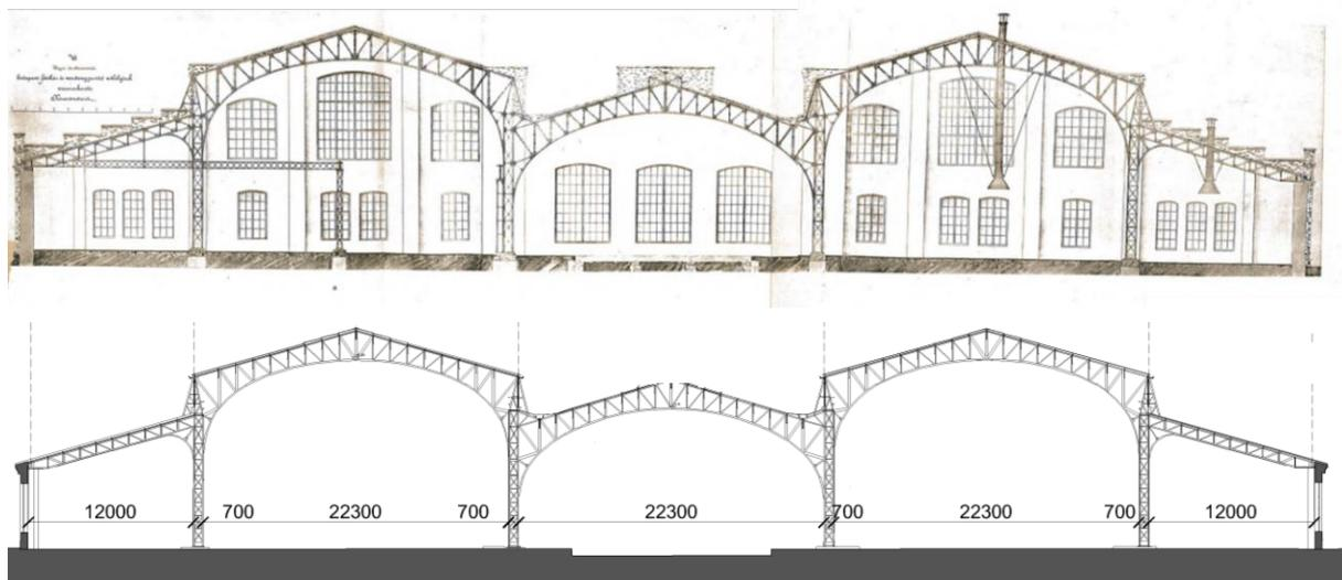
**Figure 6–14** The original cross-section drawing of the hall [64], and the main steel structure..
