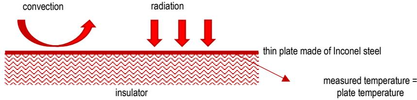
Figure 3–6 Scheme of the plate thermometer
