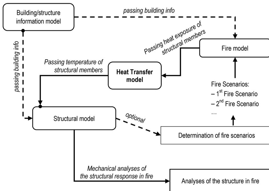
Figure 3–1 Integrated framework for analyses of structures in fire
