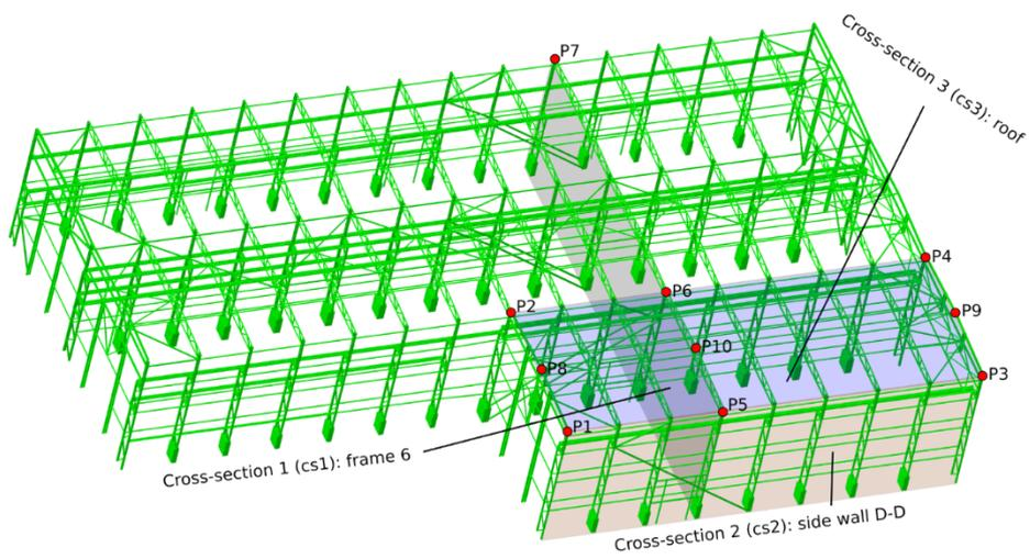
Figure 6–11 View of the structural model with displacement measurement points and cross-section being analysed.
