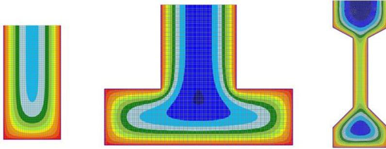
Figure 3–17 Colormaps representing different temperature profiles in concrete cross-sections.
