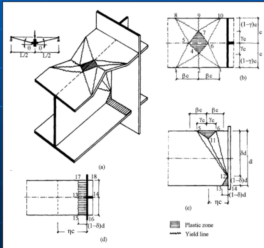
✓ Buckled shape of the compression flange is represented by a double-triangular plastic zone and several yield lines
