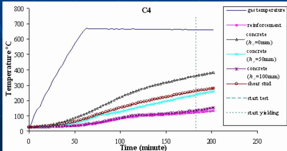
➤ Furnace temperature set between 650 and 800° C based on 7 to 10° C/min
