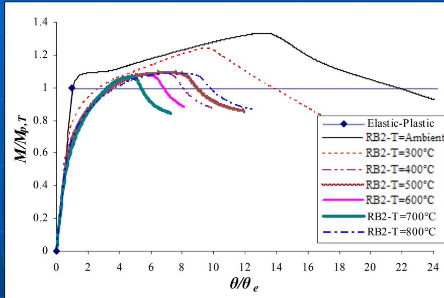
➤ Rotational capacity reduces as temperature increases
