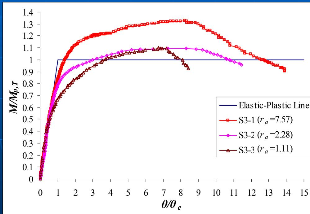
**Conservatism of design plastic moment capacity has reduced from up to 30% to a low of 10% as temperature increased to 615°**
