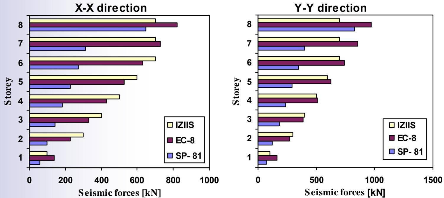
**Seismic forces obtained according to SP-81, EC8 and IZIIS Methodology**
