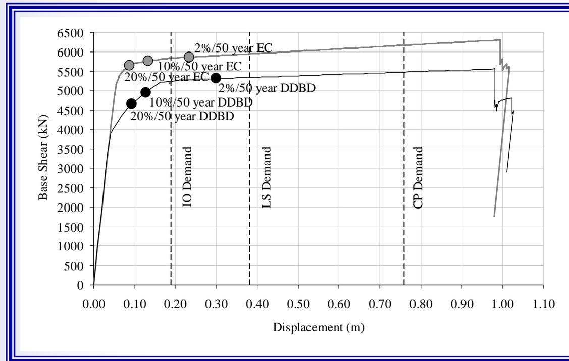
Capacity curve for building designed according to DDBD and EC8
