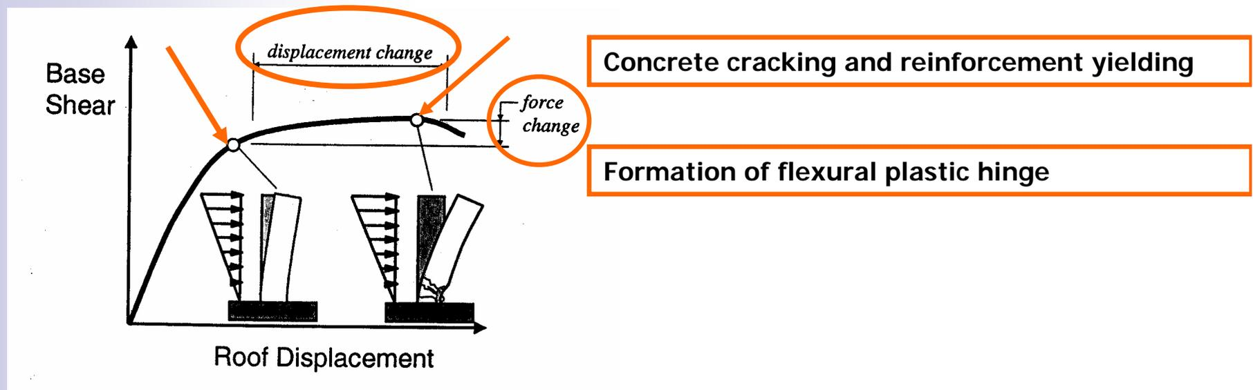
**The extent of damage is related to the amount of deformation (turn to displacement) in plastic hinge**
