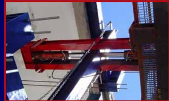
Close-up views of the reacting structure with the load jacks
