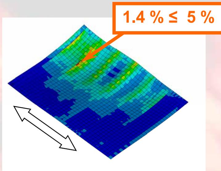
Strain of reinforcing steel
