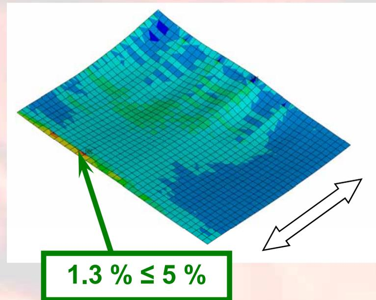
Strain of reinforcing steel
