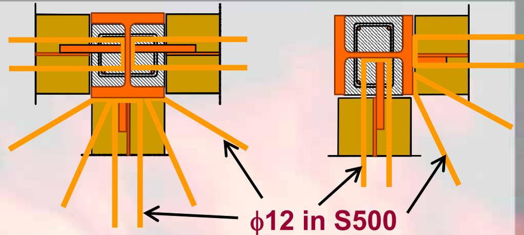
Maximum gap of 15 mm between beam and column and between lower flange of the beam
