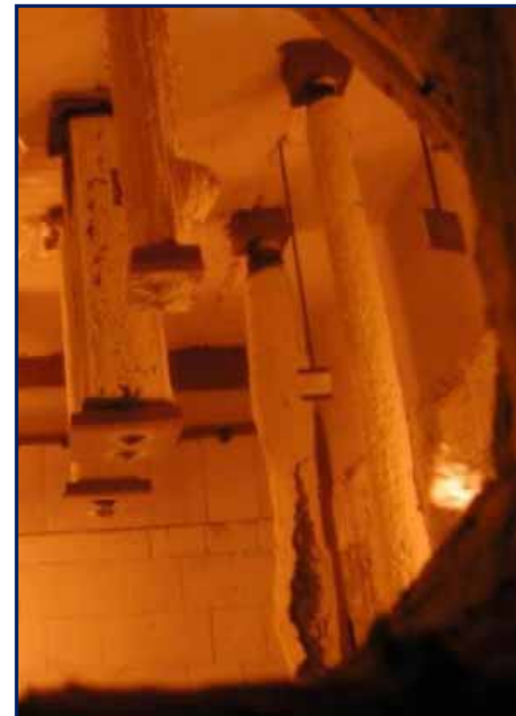
Fire test of intumescent coating
