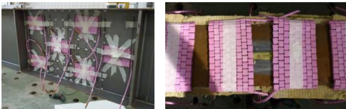
Figure 17: Photo of the distributed heating mats: *left) on the web, right) on the flange*
