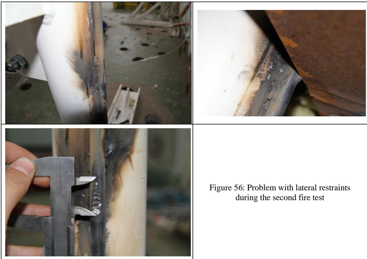
Figure 56: Problem with lateral restraints during the second fire test
