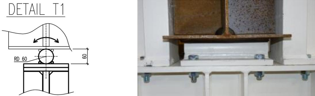
Figure 11: fixed articulation support: left) construction detail, right) side view of the finished support
