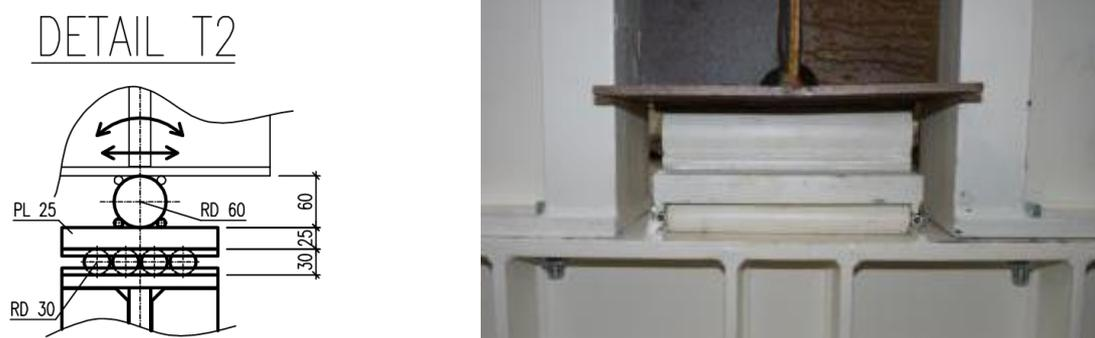
Figure 12: sliding articulation support: left) construction detail, right) side view of the finished support
