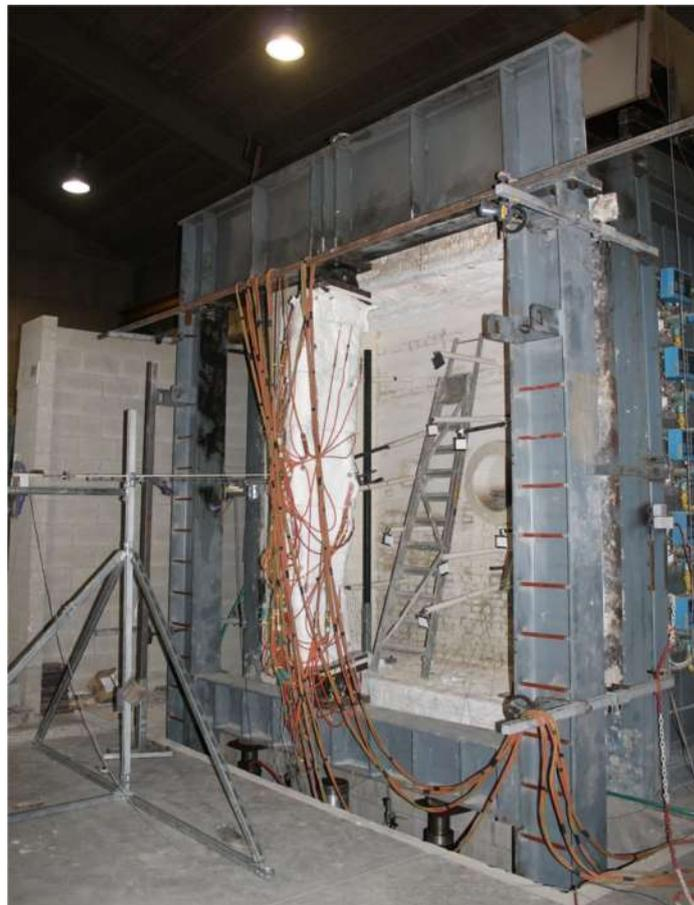
Figure 16: Testing frame for the experimental tests with the equipped column
