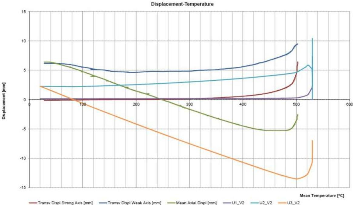
Figure 89: Displacements (mm) in function of temperature (°C) – ABAQUS comparison
