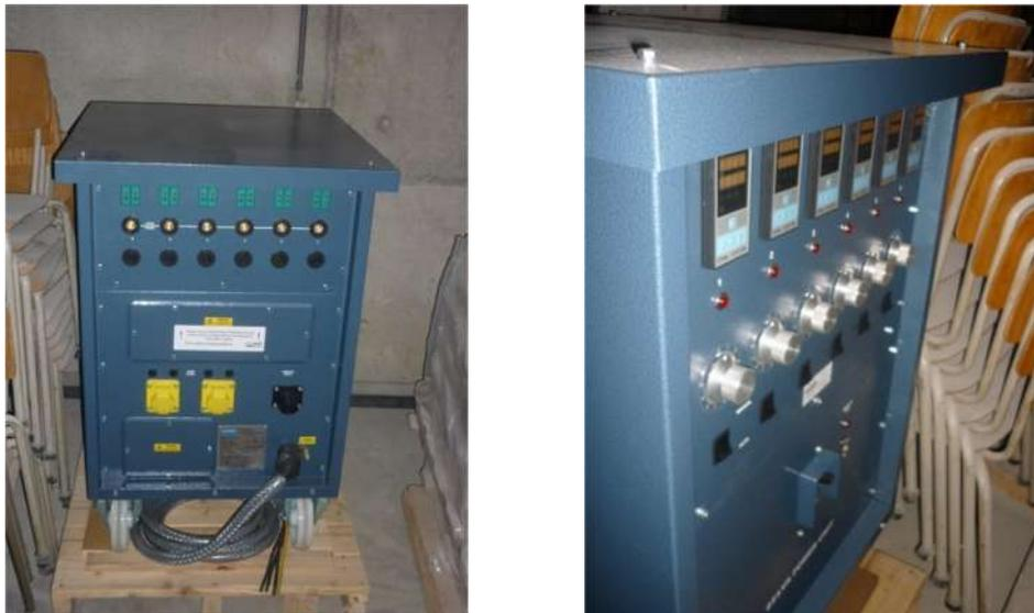
Figure 20: Mannings 65 kV.A power unit with six temperature controllers
