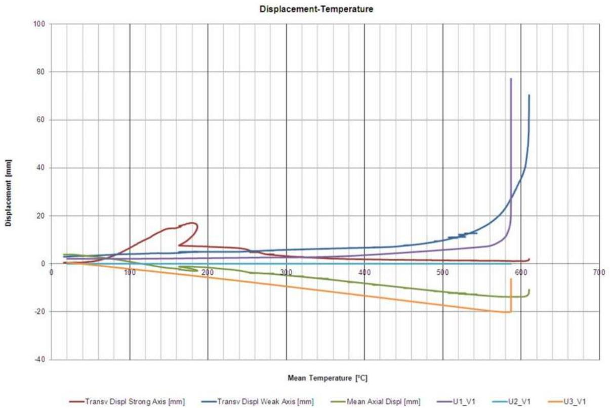
Figure 77: Displacements (mm) in function of temperature (°C) – ABAQUS comparison
