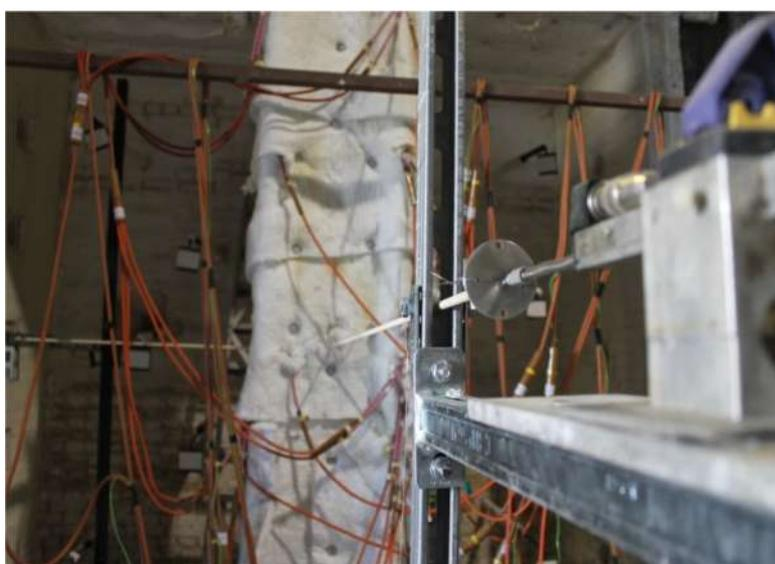
Figure 24: Displacement transducer
