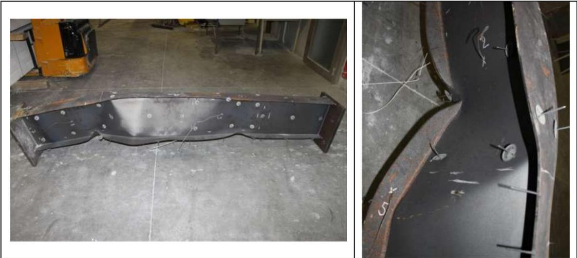
Figure 59: Deformed shape after test 5
