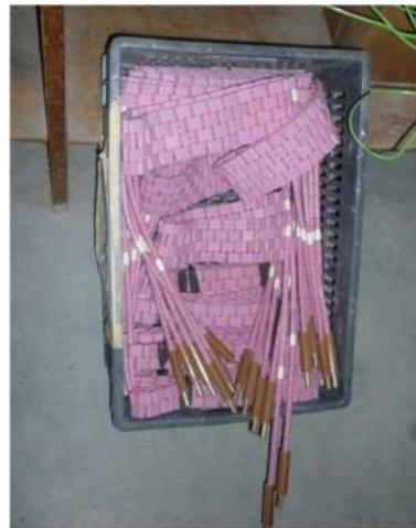
Figure 22: Ceramic pad heating elements
