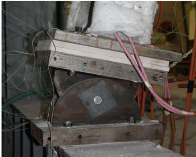
Figure 19: Pinned support with thermal disconnection
