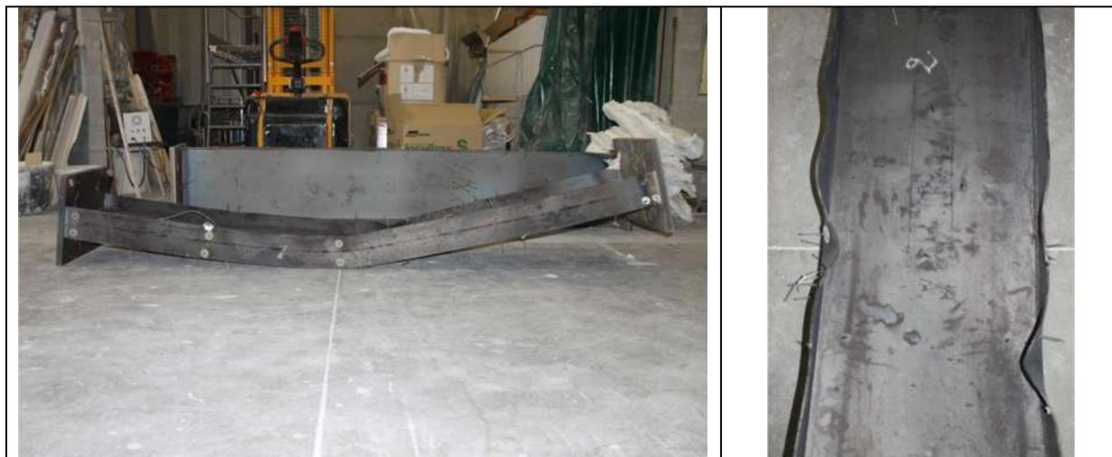
Figure 44: Deformed shape after test 2
