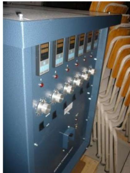
Figure 20: Mannings 65 kV.A power unit with six temperature controllers
