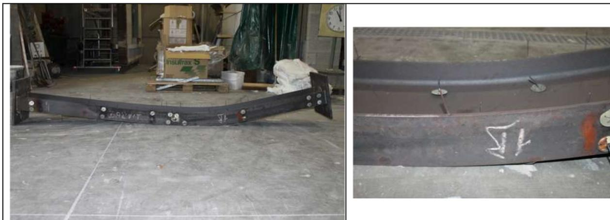
Figure 39: Deformed shape after test 1
