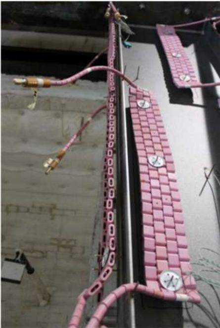
Figure 29: Location of the resistance (25 mm from the steel surface)
