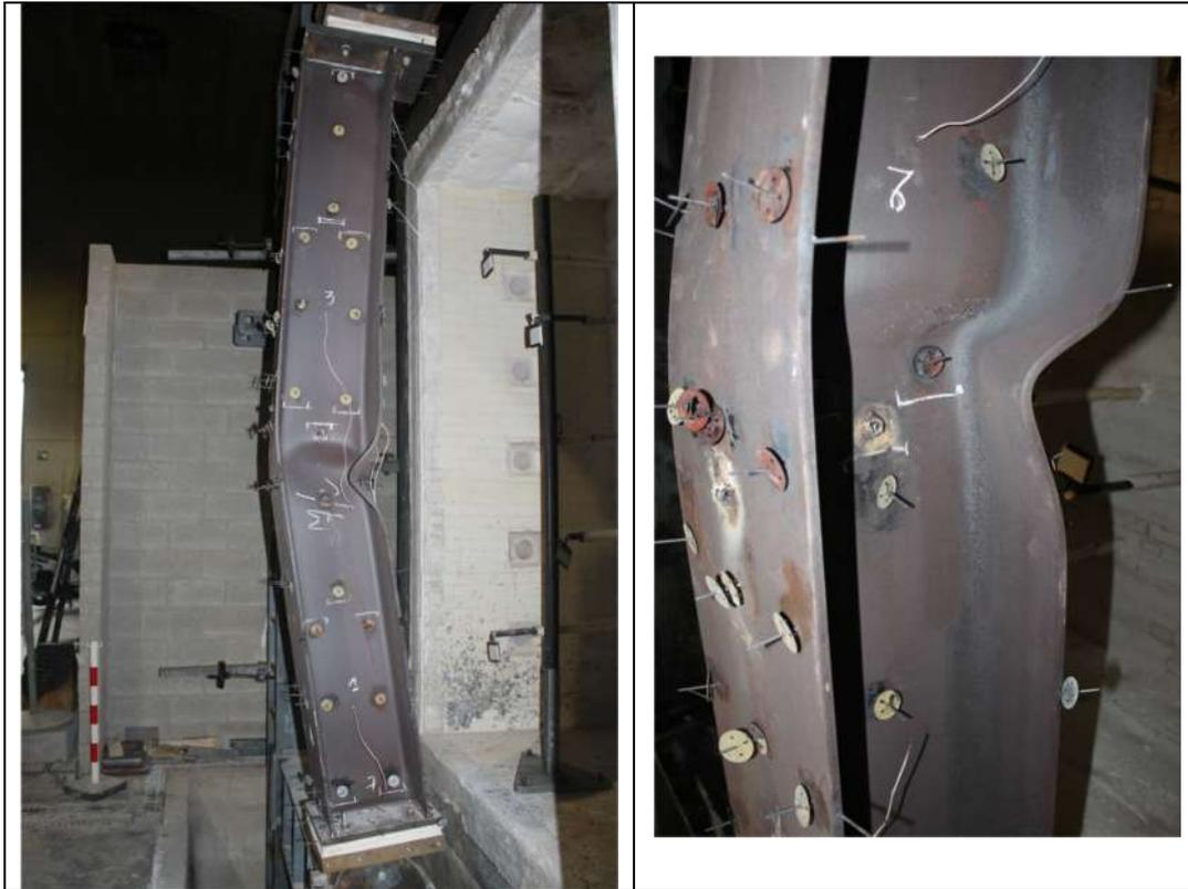
Figure 69: Deformed shape after test 7
