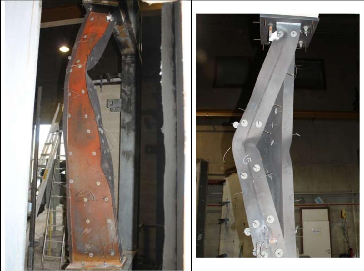
Figure 54: Deformed shape after test 4
