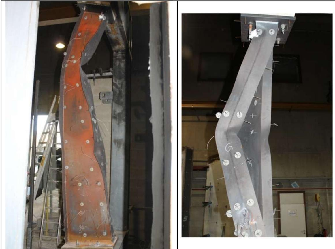
Figure 54: Deformed shape after test 4
