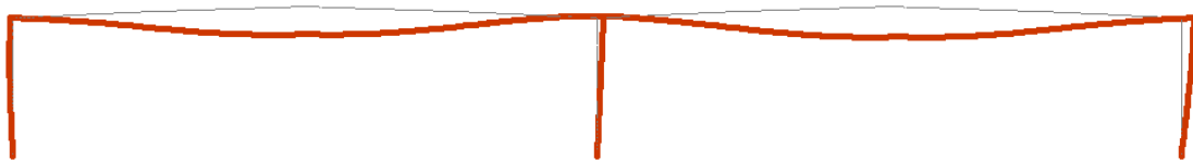
Figure 44: Deformed shape of the two span portal frame new beam model (35 kN) – internal column fire (x10)
