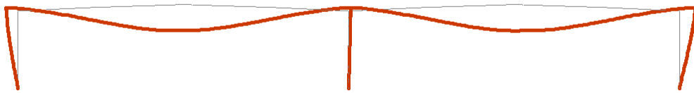
Figure 35: Deformed shape of the two span portal frame at 350 °C
