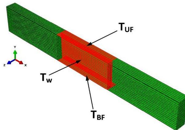
Fig. 7.7 Temperature distribution in numerical modeling
