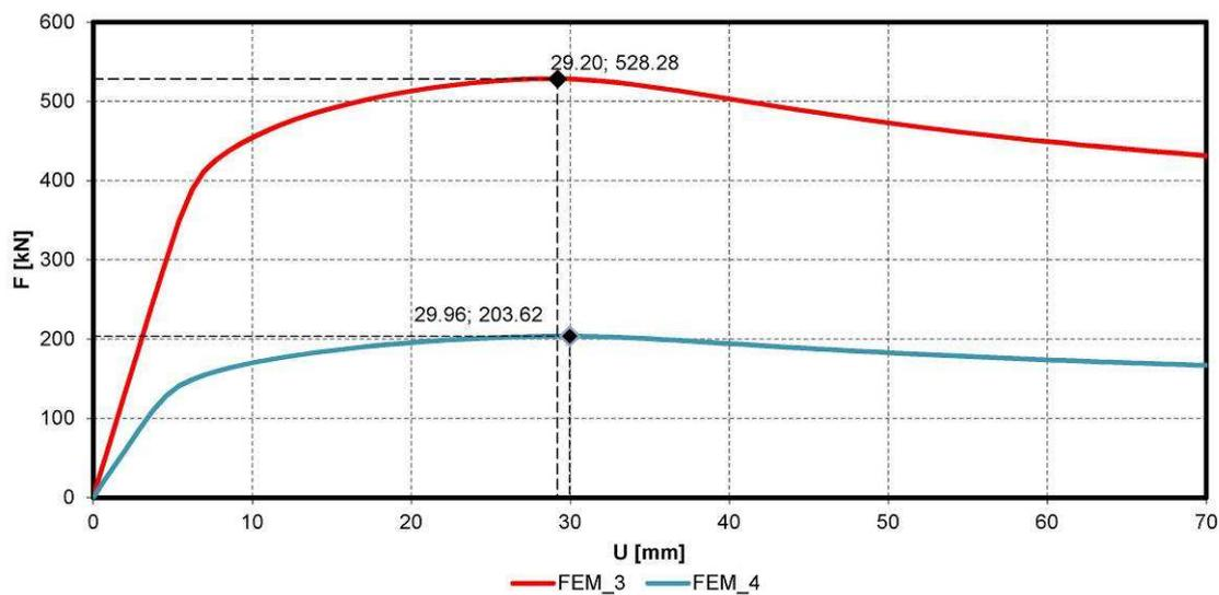
Fig. 7.11 Load-deflection diagram for simulation 3 and 4
