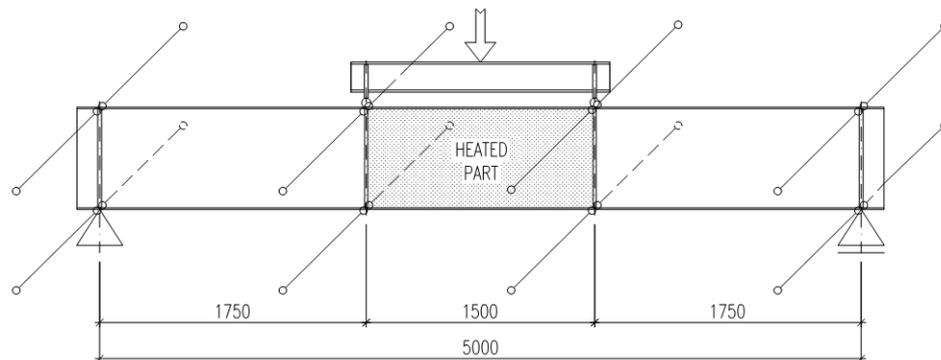
Fig. 7.1 Simulated beam
