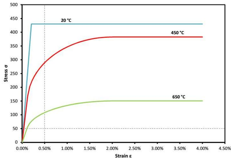
Fig. 7.5 Stress–strain relationship for steel S 355 depending on the temperature
