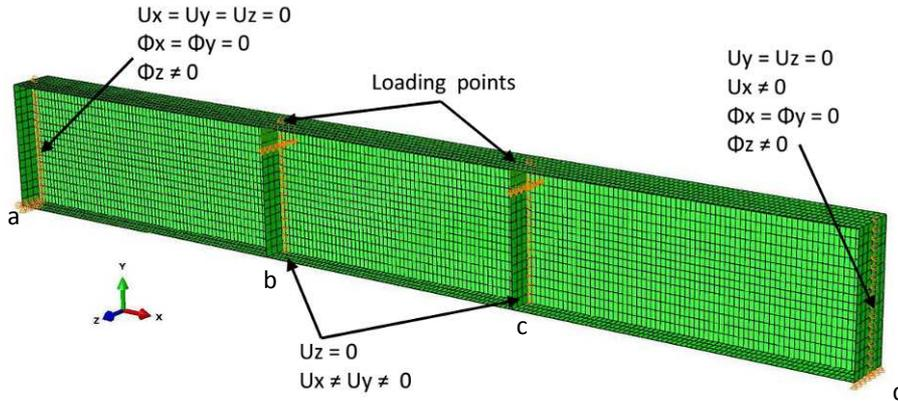
Fig. 7.6 Loading and boundary conditions for beam model
