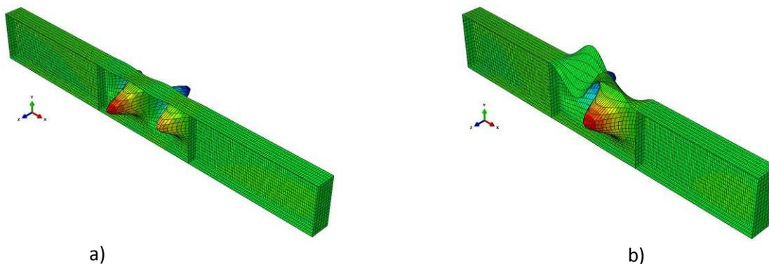
Fig. 7.4 The first elastic buckling eigenmode shape, a) simulation 1 and 2, b) simulation 3 and 4
