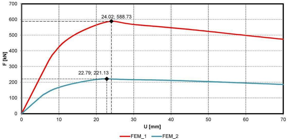
Fig. 7.9 Load-deflection diagram for simulation 1 and 2
