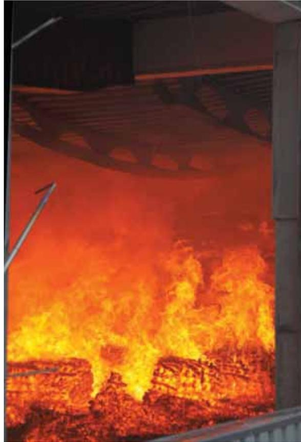
Fig. 5.7 - Deformed Angelina beam at the 48 min. of the fire test
