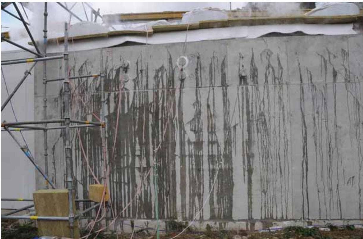
Fig. 4.46 - Water transport from the concrete on the wall at the 25. min of the fire
