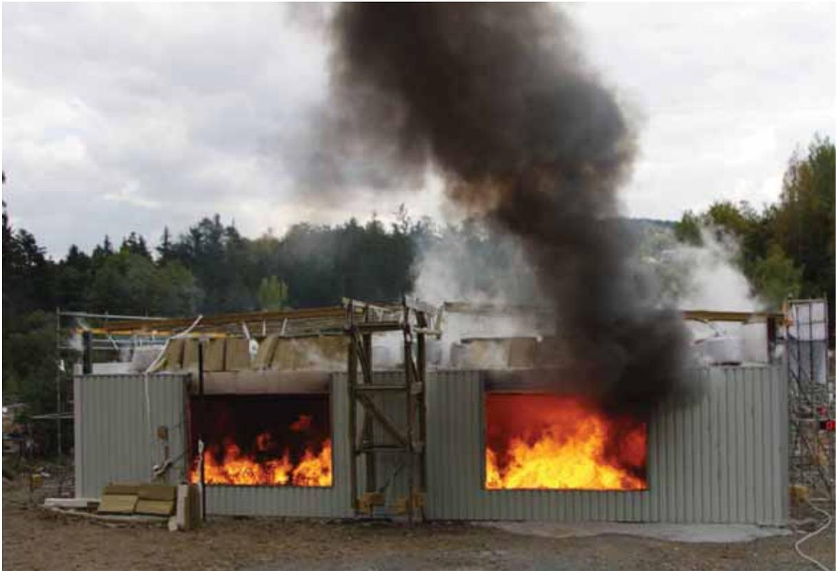
Fig. 3.11 - The view of the experimental structure; flames in the west opening at the 50. min of the fire test
