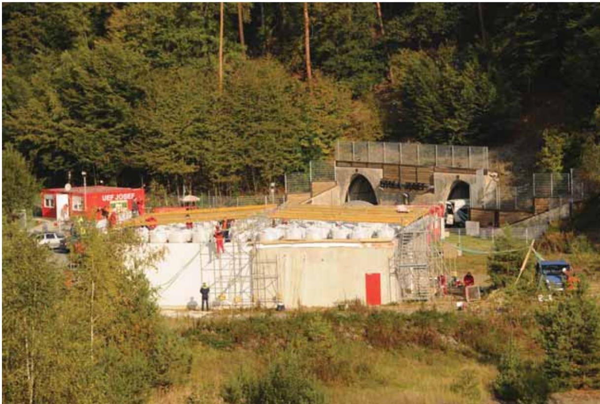
Fig. 5.4 - Independent scaffolding for deflection measurement
