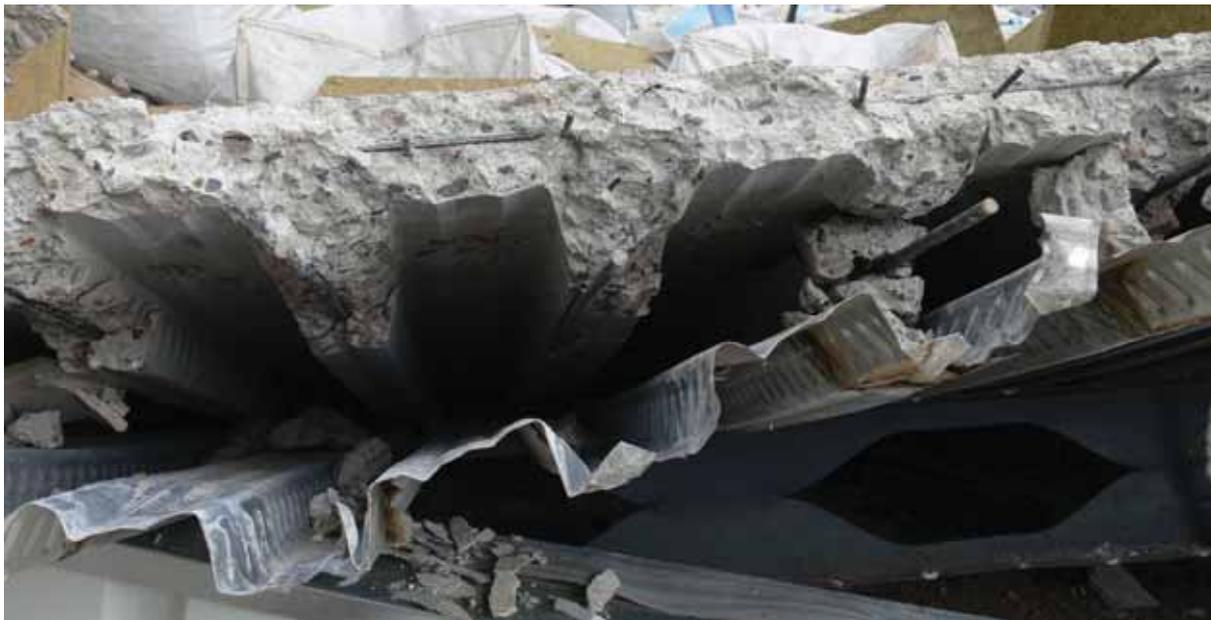
Fig. 4.33 - The cross-section of the composite slab after the fire experiment
