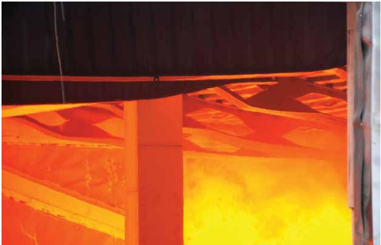
Fig. 5.6 - Deformation of castellated beams behind the deflected beams with corrugated web at the 37. min of the fire
