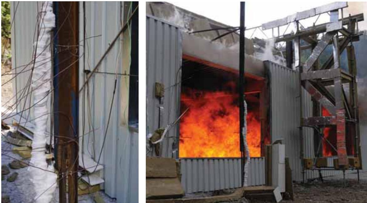
Fig. 4.29 - The thermocouples on the column before and during the fire test
