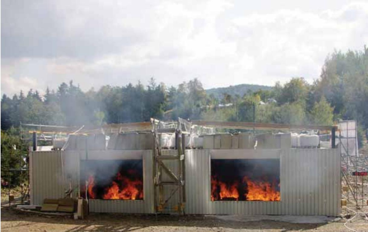
Fig. 3.10 - The view at the experimental structure; flames in the east opening at the 36. min of the fire test
