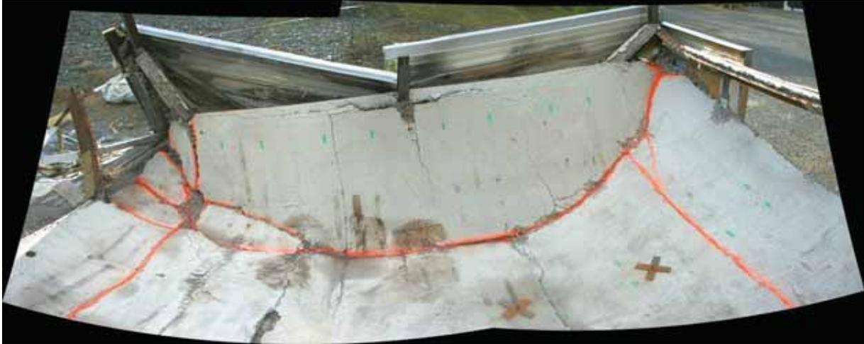
Fig. 8.4 - The panoramic top view of the slab under the castellated beams with visualised major cracks
