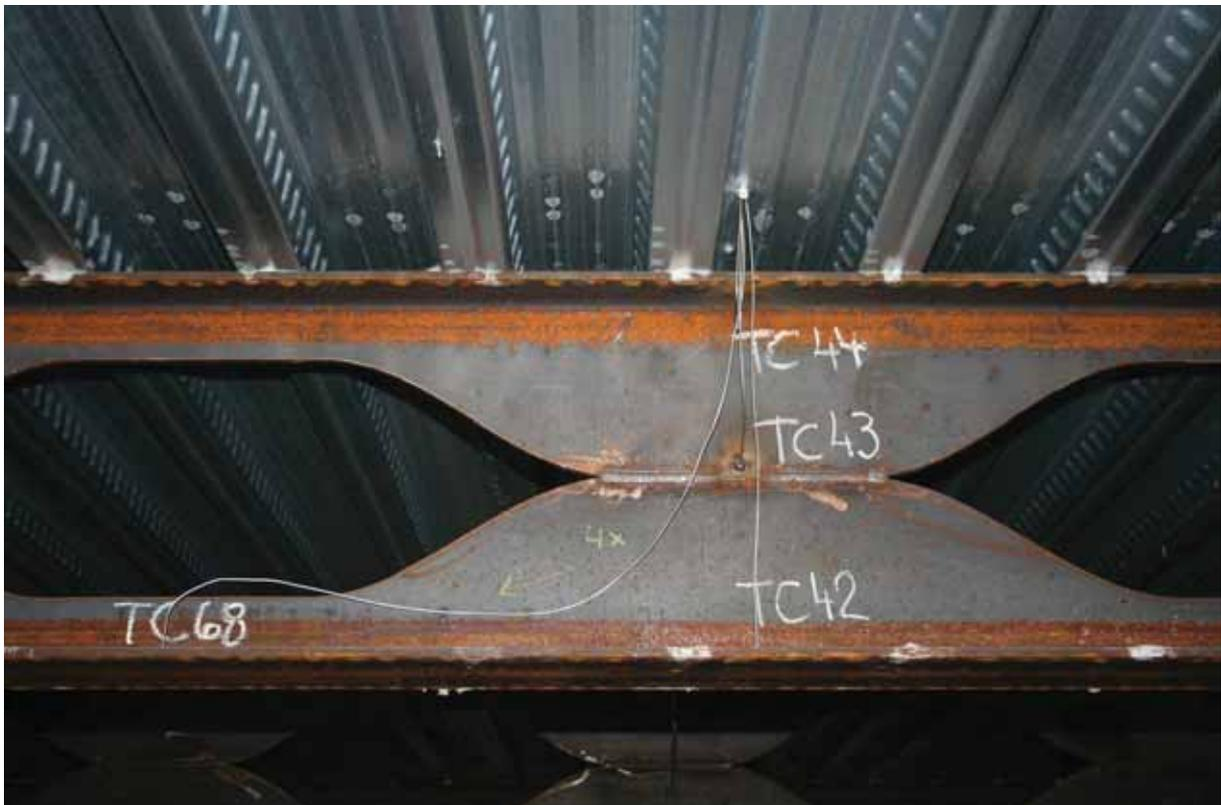
Fig. 4.7 - Thermocouples located at the midspan and along the height of the Angelina beam AS4
