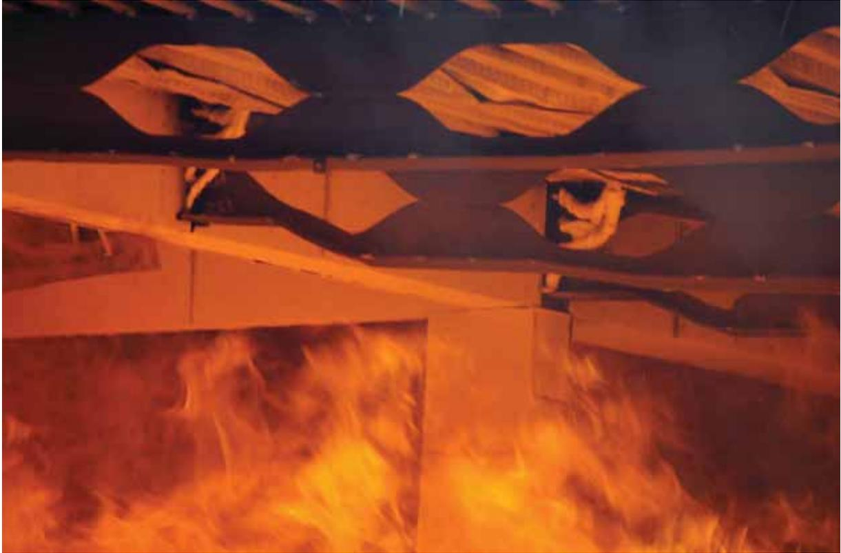
Fig. 5.5 - The deformed beams with corrugated web at the 25. min of the fire test
