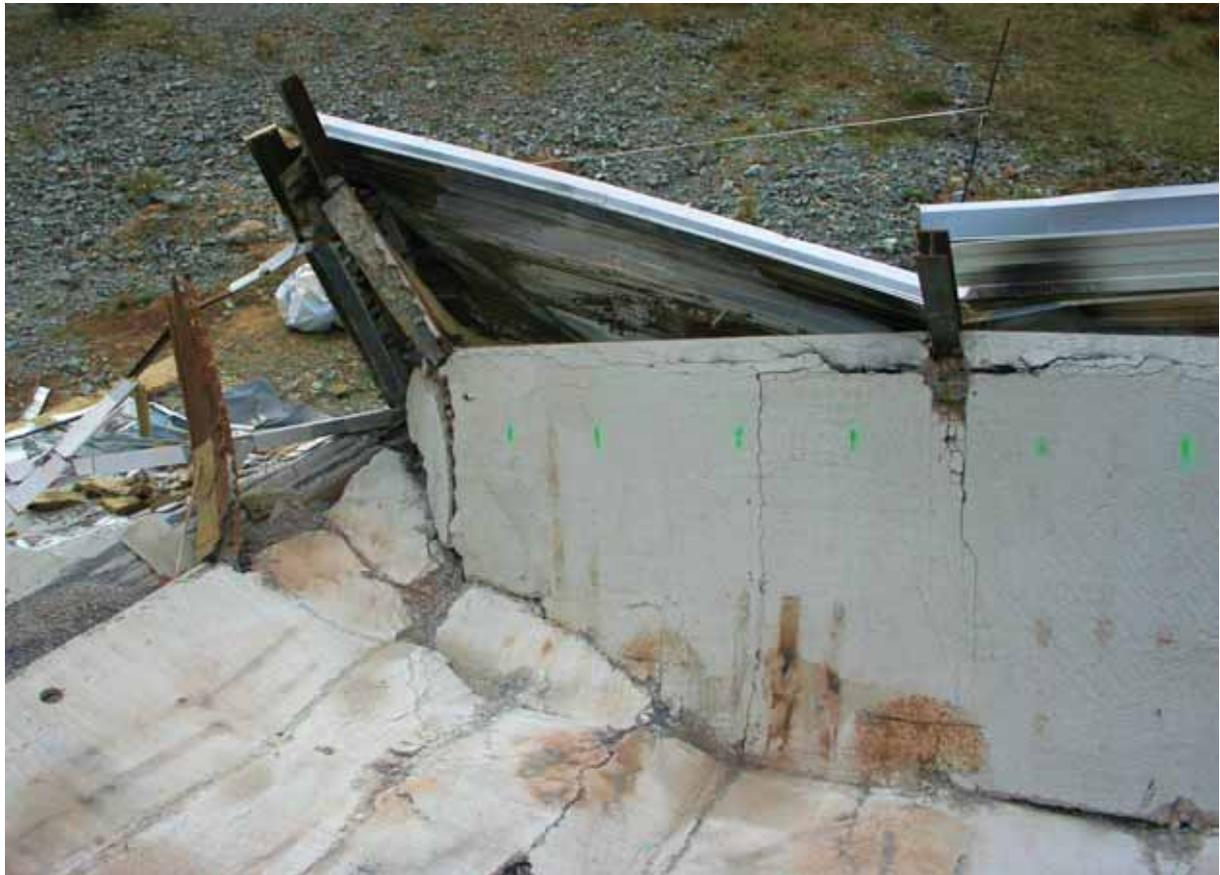
Fig. 8.7 - The edge beam in the corner of the slab after buckling
