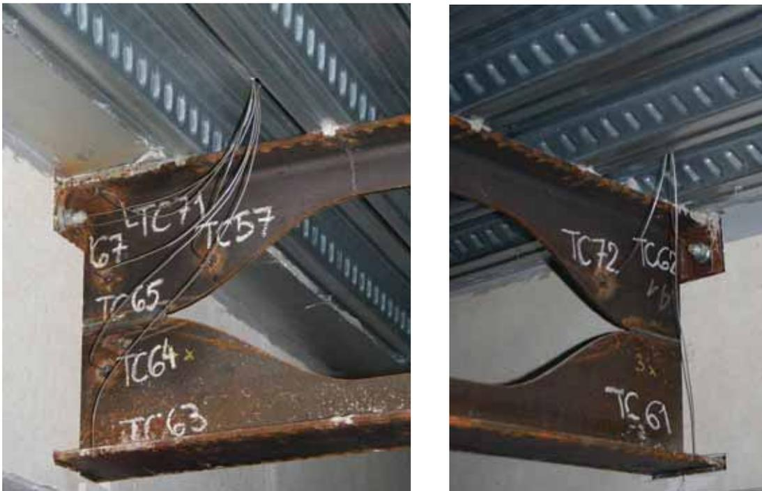
Fig. 4.16 - Location of thermocouples at connections A and B on Angelina beam AS5
