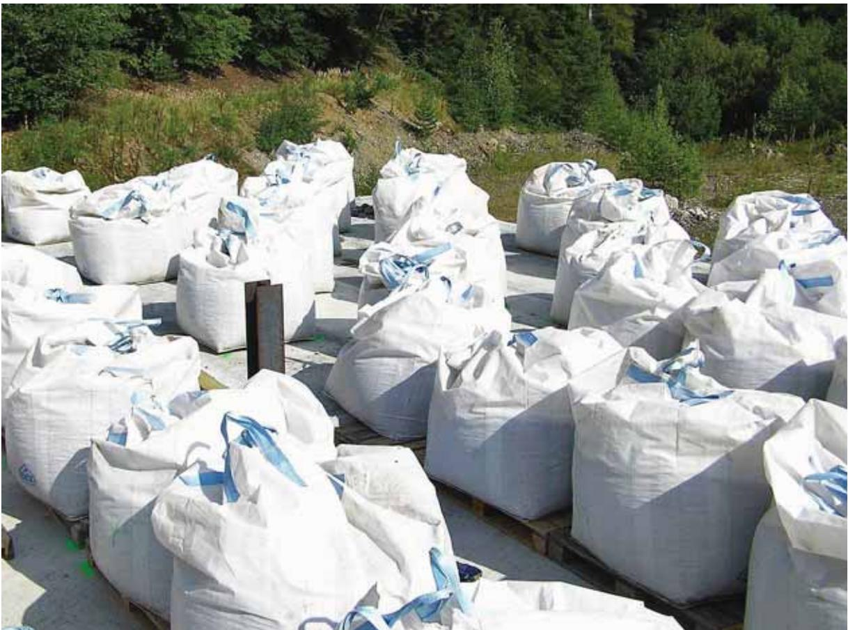
Fig. 2.3 - Mechanical load on the floor in bags on wooden pallets
