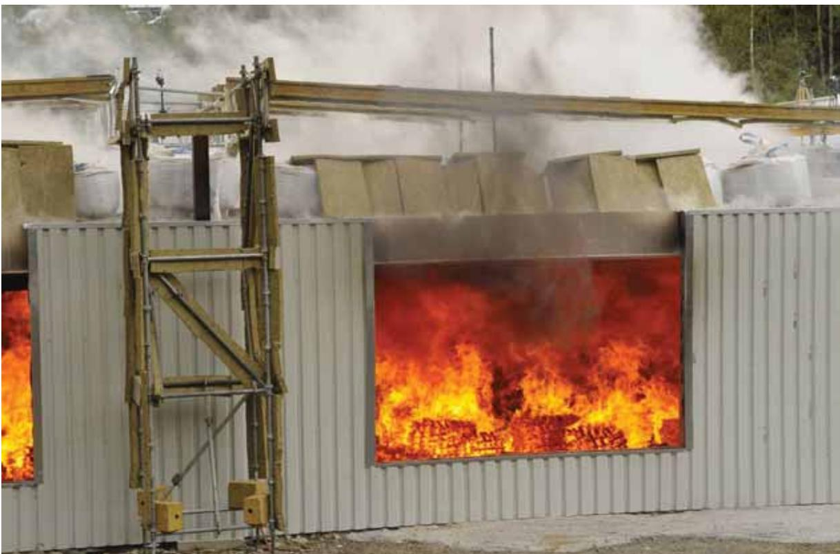
Fig. 3.12 - Flames in the west opening at the 52. min of the fire test
