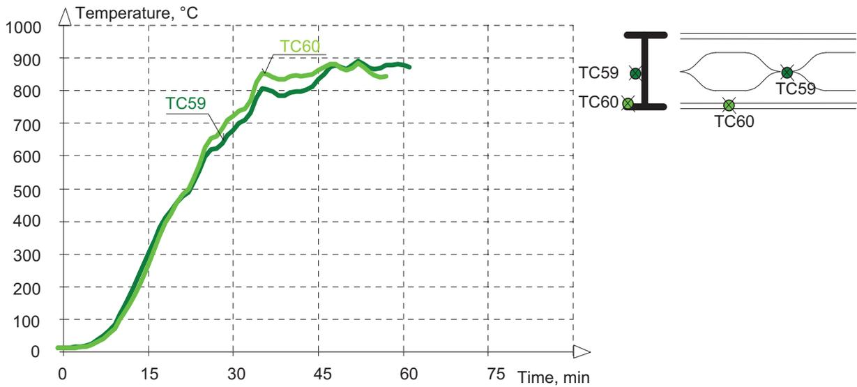
Fig. 4.3 - Temperatures measured at the midspan of the cellular Angelina beam AS5
