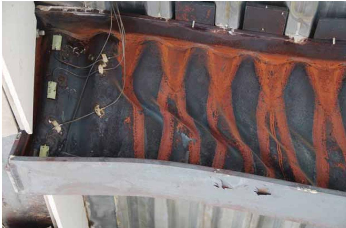
Fig. 6.4 - The web of the beam with corrugated web after the fire test with visible strain gauges and thermocouples
