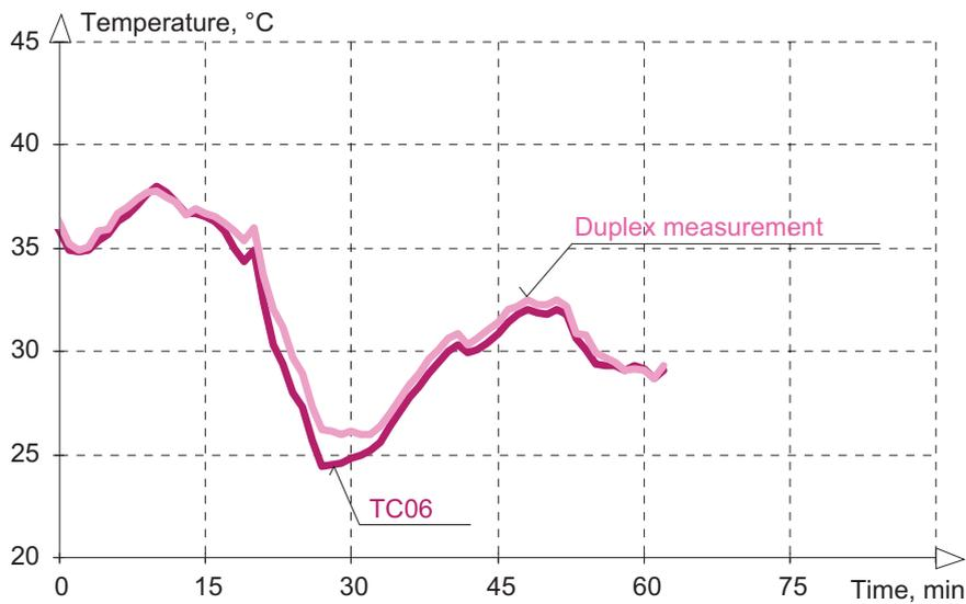
Fig. 4.35 - Temperatures measured in the middle of the external sheet of the sandwich panel, wall AB1
