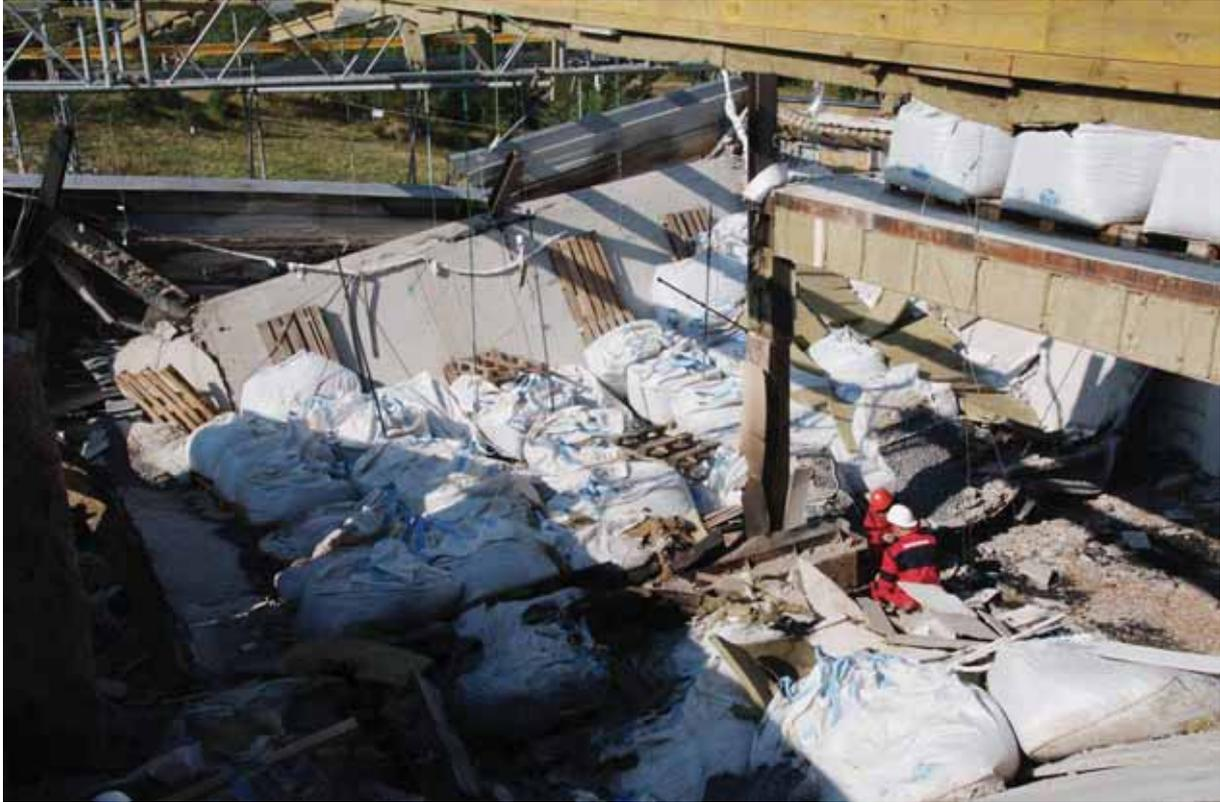
Fig. 8.2 - The top view of the slab under the castellated beams after the fire test
