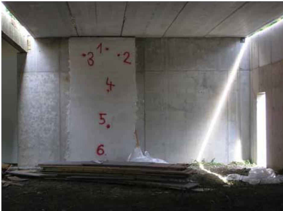
Fig. 5.52 - The view of the plaster wall in front of the concrete wall under hollow core panels in the fire compartment before the fire test
