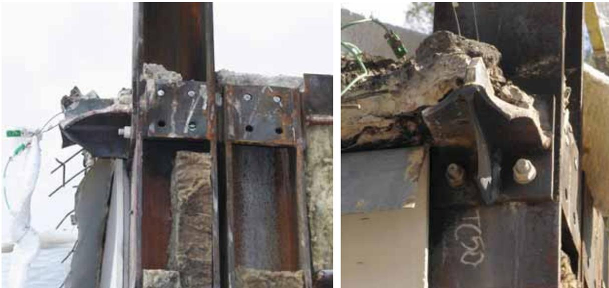
Fig. 8.9 - The rest of the Angelina beam to the central column connection after the break of the composite slab
