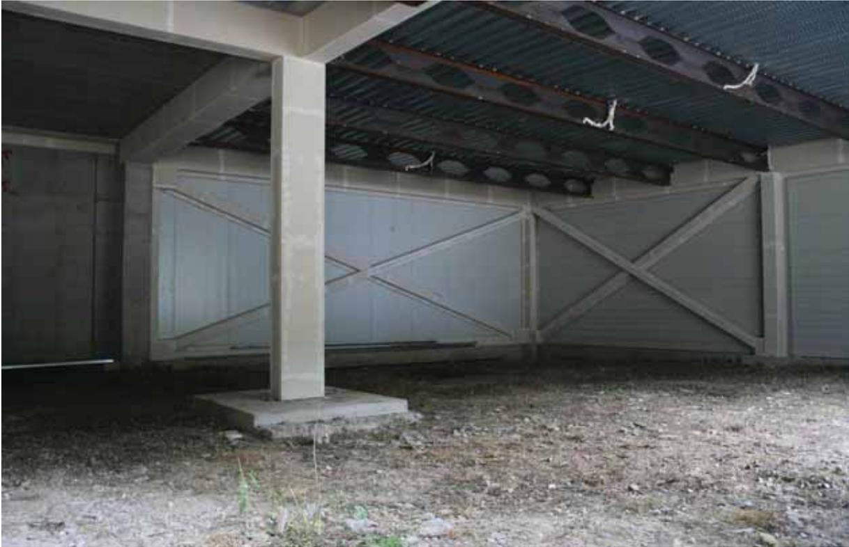
Fig. 1.8 - The west part of the fire compartment before the test
