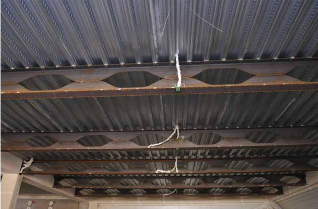
Fig. 4.6 - Thermocouples located at the midspan of the cellular beams and at their connections
