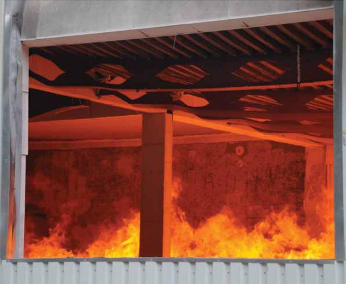
Fig. 4.47 - Spalling of the concrete on the wall at the 45. min of the fire
