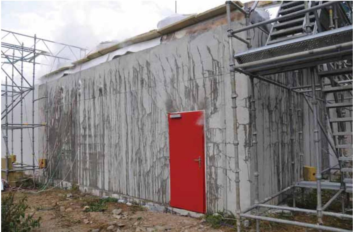
Fig. 4.45 - Transport of water to the external face of the concrete wall at the 30. min of the fire
