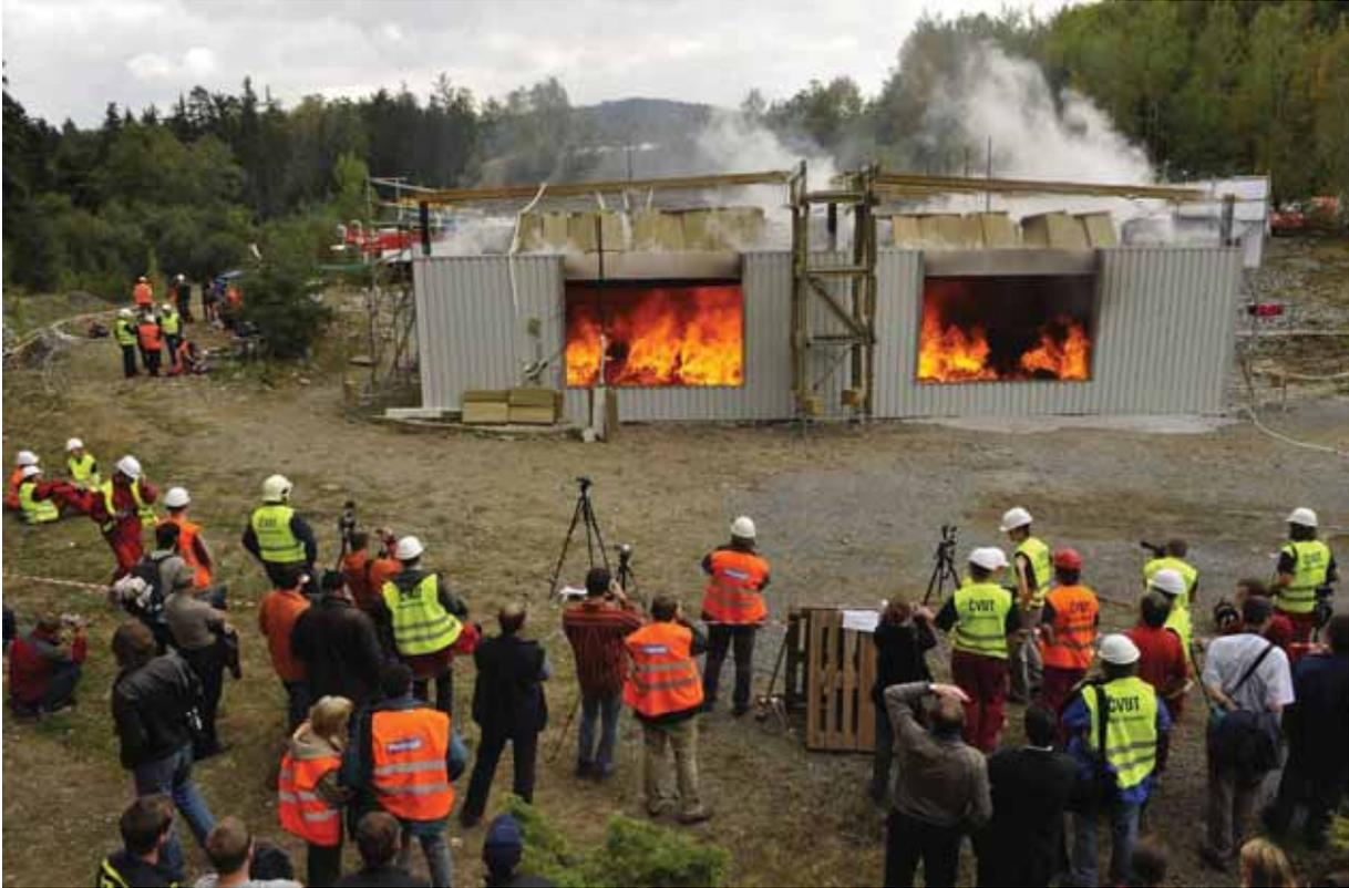
Fig. 3.9 - The view of the experimental structure; flames at the 35. min of the fire test
