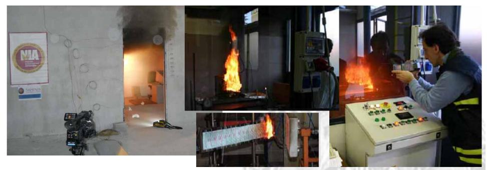
The parameters checked during full-scale fire experiments are then compared, through numerical model, with the output data of simulations carried out under the same conditions.
