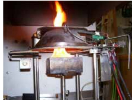
Pine exposed at Heat flux 35kW/m 2
