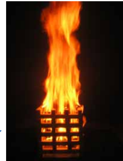
Untreated pine crib into the test.
