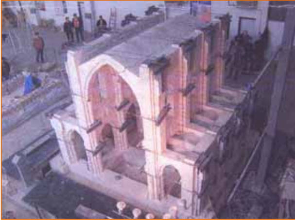
Fossanova Full scale Model – shaking table test
