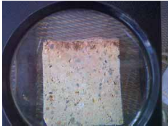
Thickness degraded - 2,70cm
