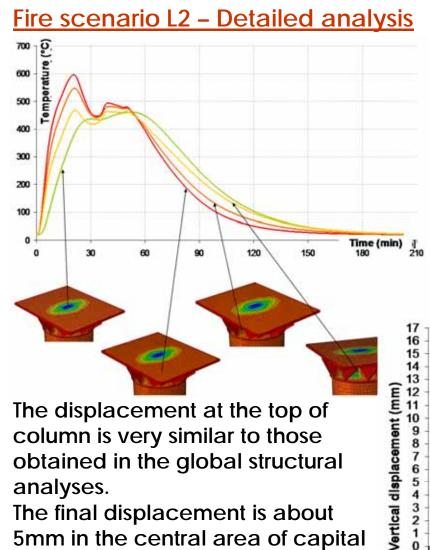
The 3D Thermal Analyses allowed to calculate more accurately the thermal field and stresses distribution in the capitals above the columns.
