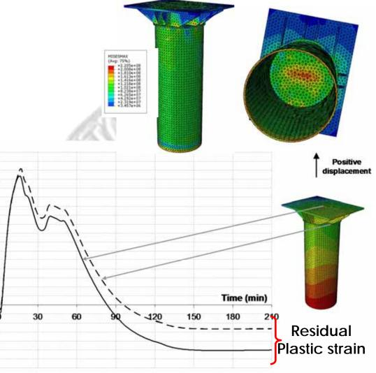
The displacement at the top of column is very similar to those obtained in the global structural analyses.
