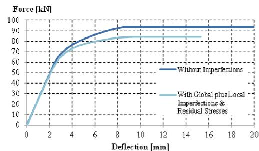
Figure 2 – Relation between imposed force and displacement
