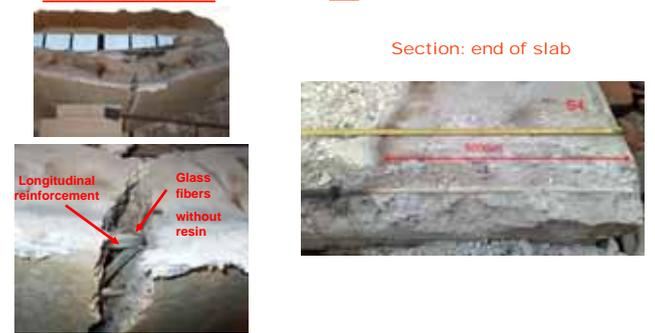
Fire resistance of concrete slabs reinforced with FRP bars. Experimental investigations and numerical simulation on the thermal field and the mechanical behaviour Antonio Bilotta, PhD - University of Naples Federico II - Department of Structures for Engineering and Architecture
