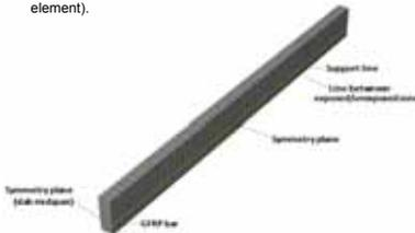
Each slab is divided into finite elements "Brick" type "Hex" (parallelepiped elements), with maximum dimensions of 70mm x 28mm x 20mm, 8 linear node (ABAQUS C3D8 element).
