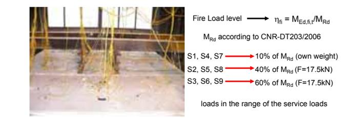
Fire resistance of concrete slabs reinforced with FRP bars. Experimental investigations and numerical simulation on the thermal field and the mechanical behaviour Antonio Bilotta, PhD - University of Naples Federico II - Department of Structures for Engineering and Architecture
