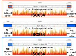
Fire resistance of concrete slabs reinforced with FRP bars. Experimental investigations and numerical simulation on the thermal field and the mechanical behaviour Antonio Bilotta, PhD - University of Naples Federico II - Department of Structures for Engineering and Architecture
