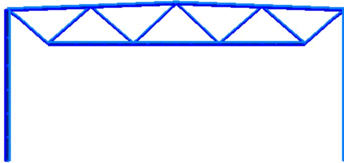
Figure 3 - Steel truss and columns of a sports hall
