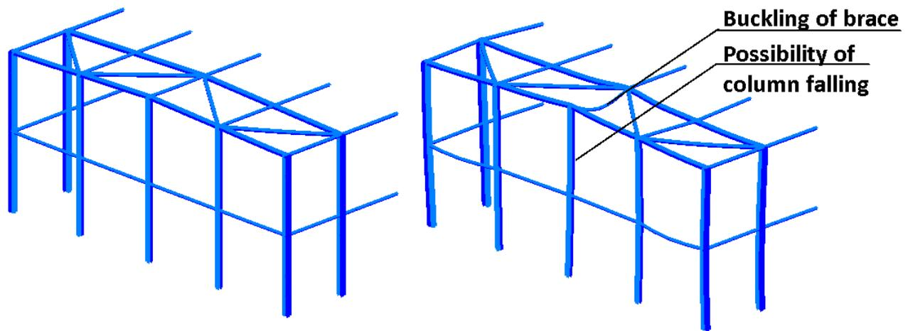
Figure 5 - Case 3, roof bracing under local fire
