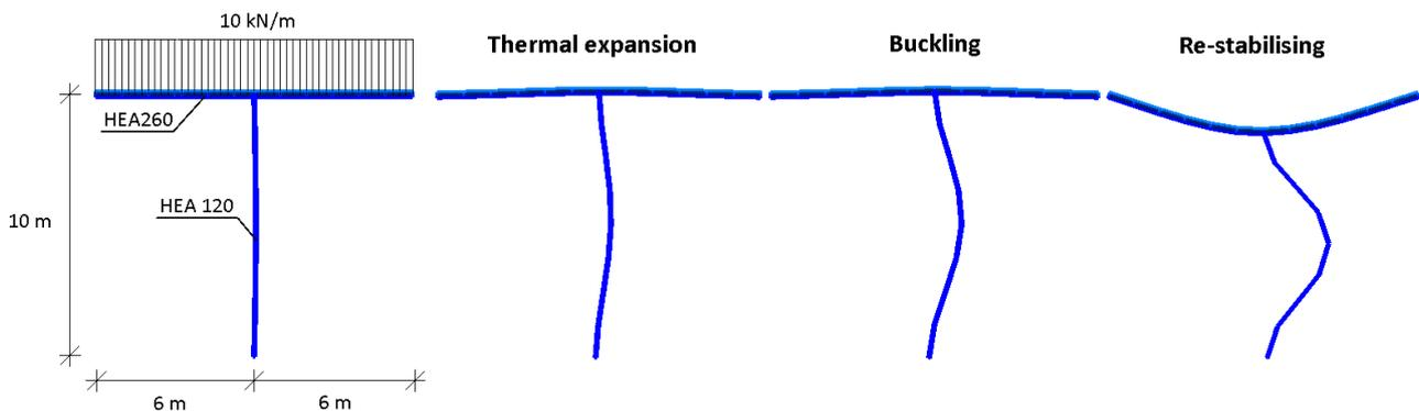
Figure 1 – The structure of case 1 and the deformed shapes at different stages of fire loading.
