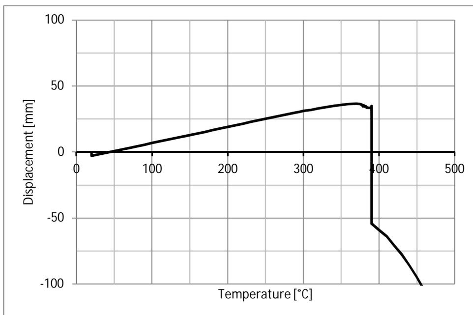
Figure 2 - The vertical displacement of the beam mid node.
