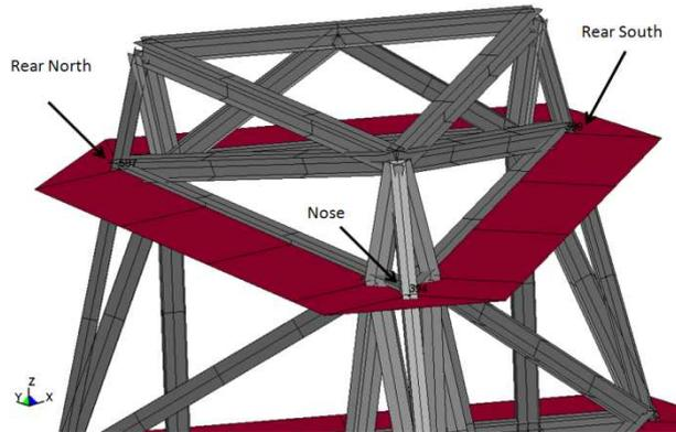
Fig. 2. Location of nodes for vertical deflection measurement.
