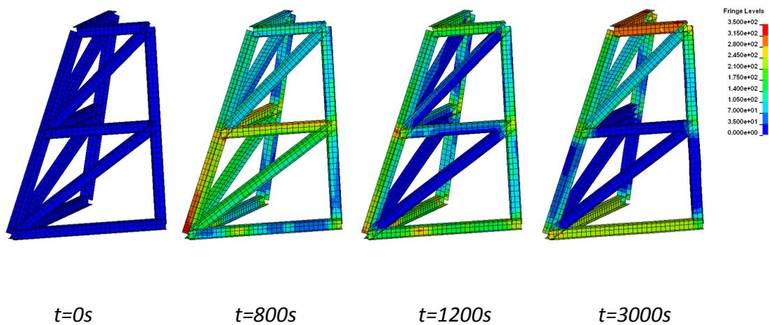
Fig. 8. Effective stress distribution in the part of frame modeled with shell elements.
