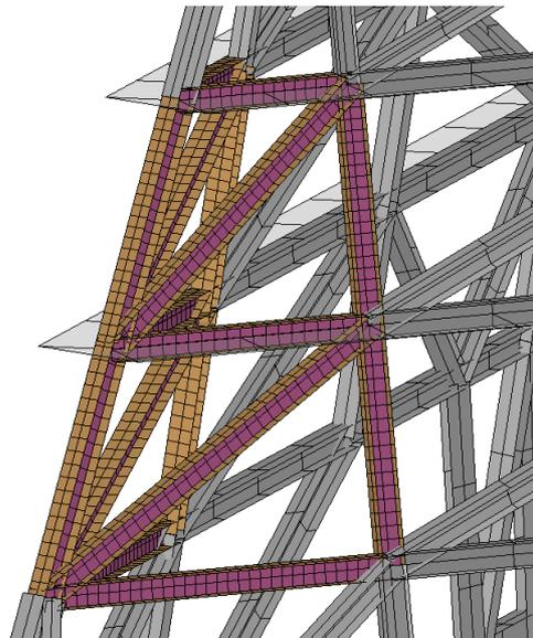
Fig. 3. Combined beam and shell element model of the frame.
