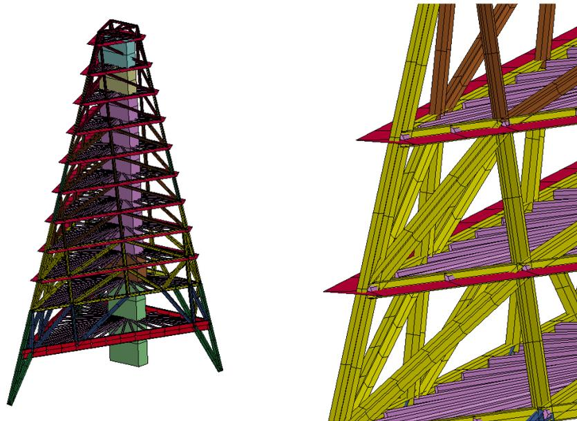
*Fig. 1. LS-DYNA model of a steel frame in ME Hotel Aldwych.*
