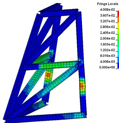
*Fig. 9. Development of plastic strains in the elements modeled using shell elements.*
