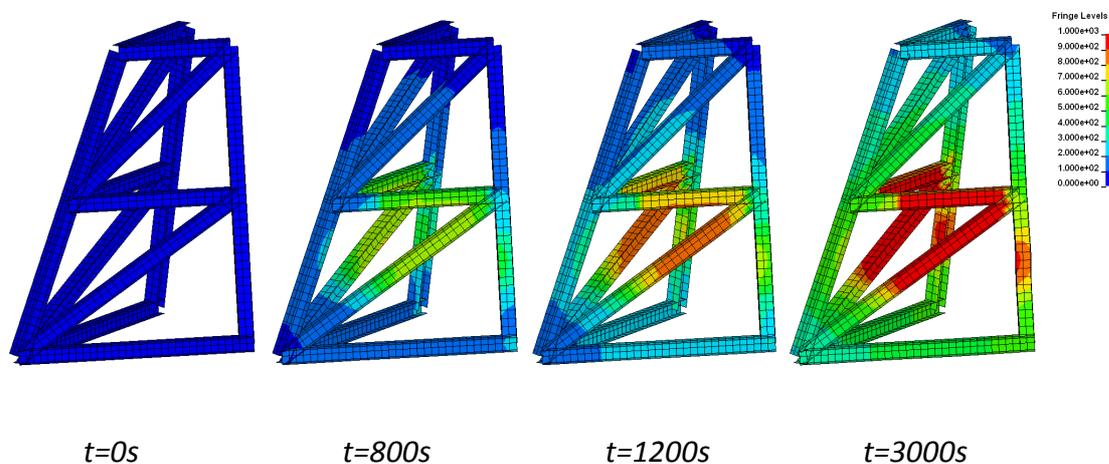
Fig. 5. Temperature distribution in the part of frame modeled using shell elements.
