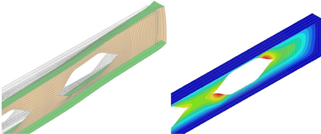
Figure 4: Deflected shape (left), iso values of out of plane displacement (right)
