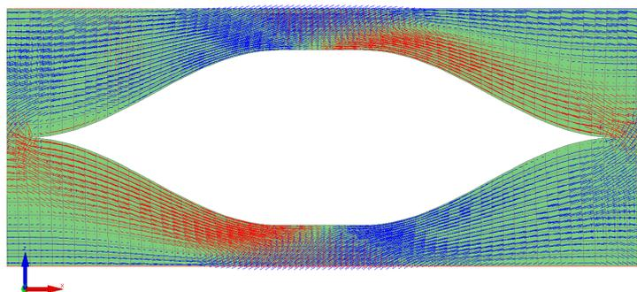
Figure 10: stresses for a time  $t = 923.5$  s (steel:  $673^\circ$ )
