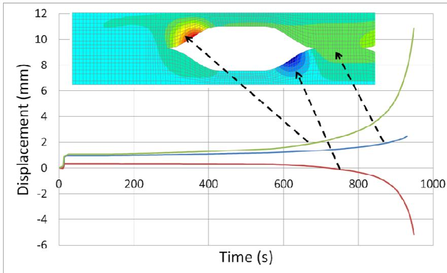
Figure 6: Out of plane displacements for the opening quarter and the intermediate web post without thermal expansion
