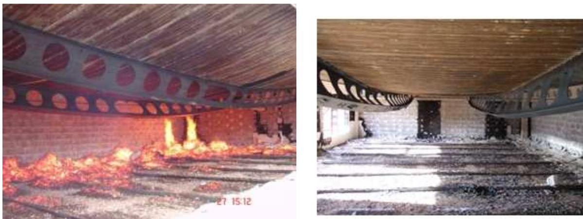
*Figure 1: Large scale fire test of cellular beams*
