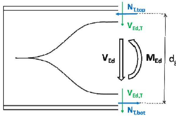
Figure 11: distribution of forces around an opening
