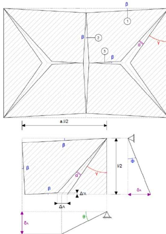
Figure 12: Assumed failure mode for the mechanism A
