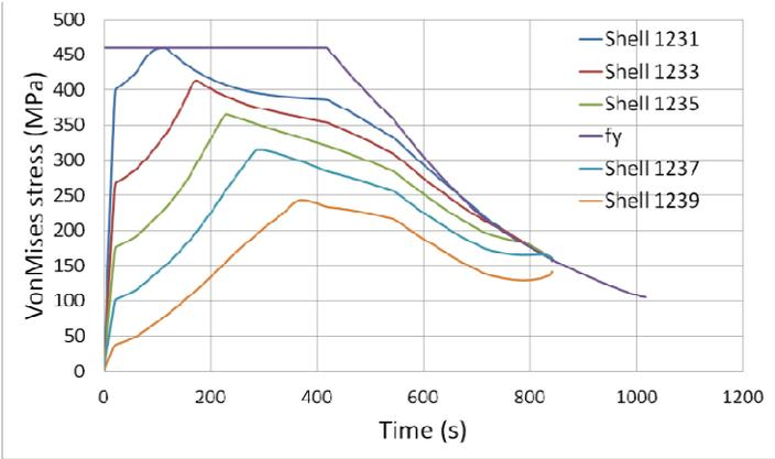
Figure 3: Equivalent vonMises stresses at an opening corner.
