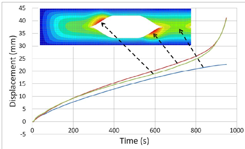
Figure 5: Out of plane displacements of the opening quarter and intermediate web-post
