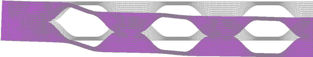
Figure 2: Formation of four plastic hinges in fire condition
