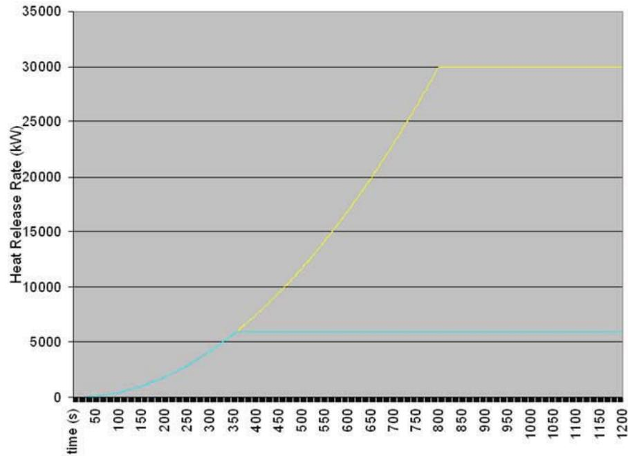
Fig. 15.5 Graph of HRR vs Time for Chosen Design Fires
