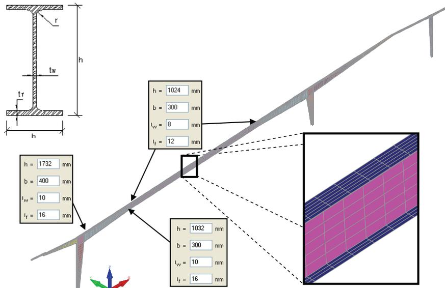
Fig. 14.5 Examples of the analysed cross-sections
