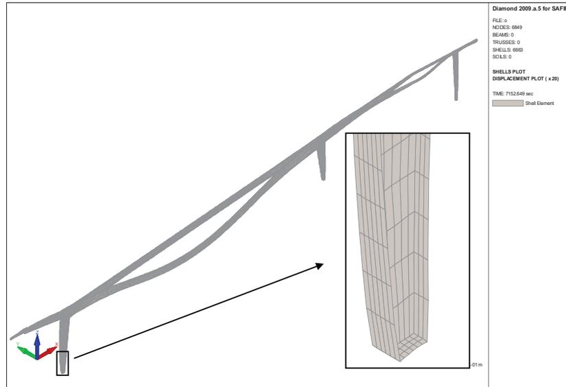
Fig. 14.12 The portal frame deformed shape, when subjected to the localized fire curve in Zone C and to the actions combination 1, at 120 minutes (x20)
