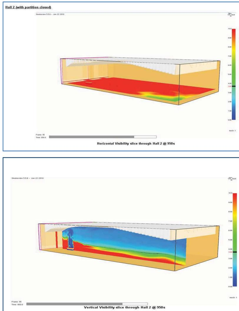
Fig. 15.6 CFD Model Slices of visibility at 950s in typical Worst Case Scenario at Tenability Limit
