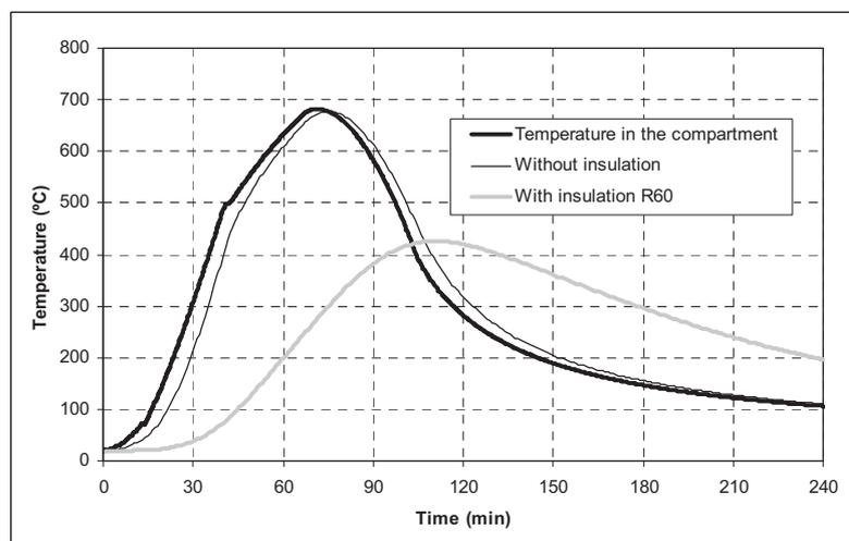
Fig. 14.6 Steel temperature evolution with and without protection
