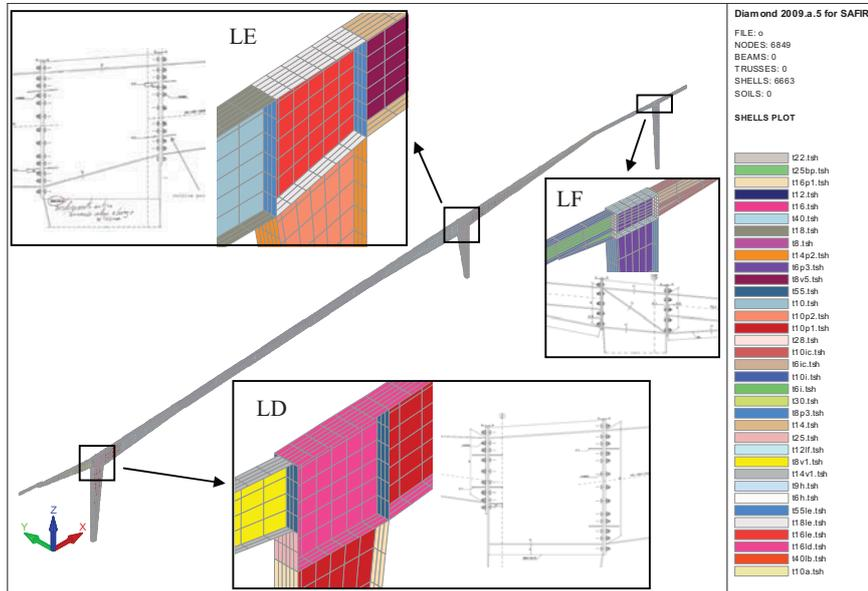
Fig. 14.7 Structural model and beam to column connection details
