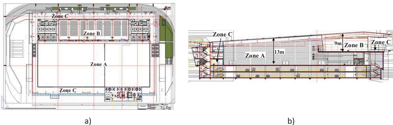
Fig. 14.1 The Oeiras Exhibitions Centre a) plan; b) cross section
