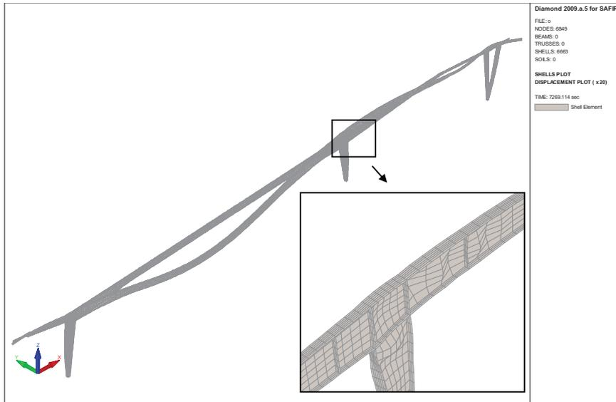
Fig. 14.10 The portal frame deformed shape, when subjected to the natural fire curve in Zone B and to the actions combination 1, at 120 minutes (x20)
