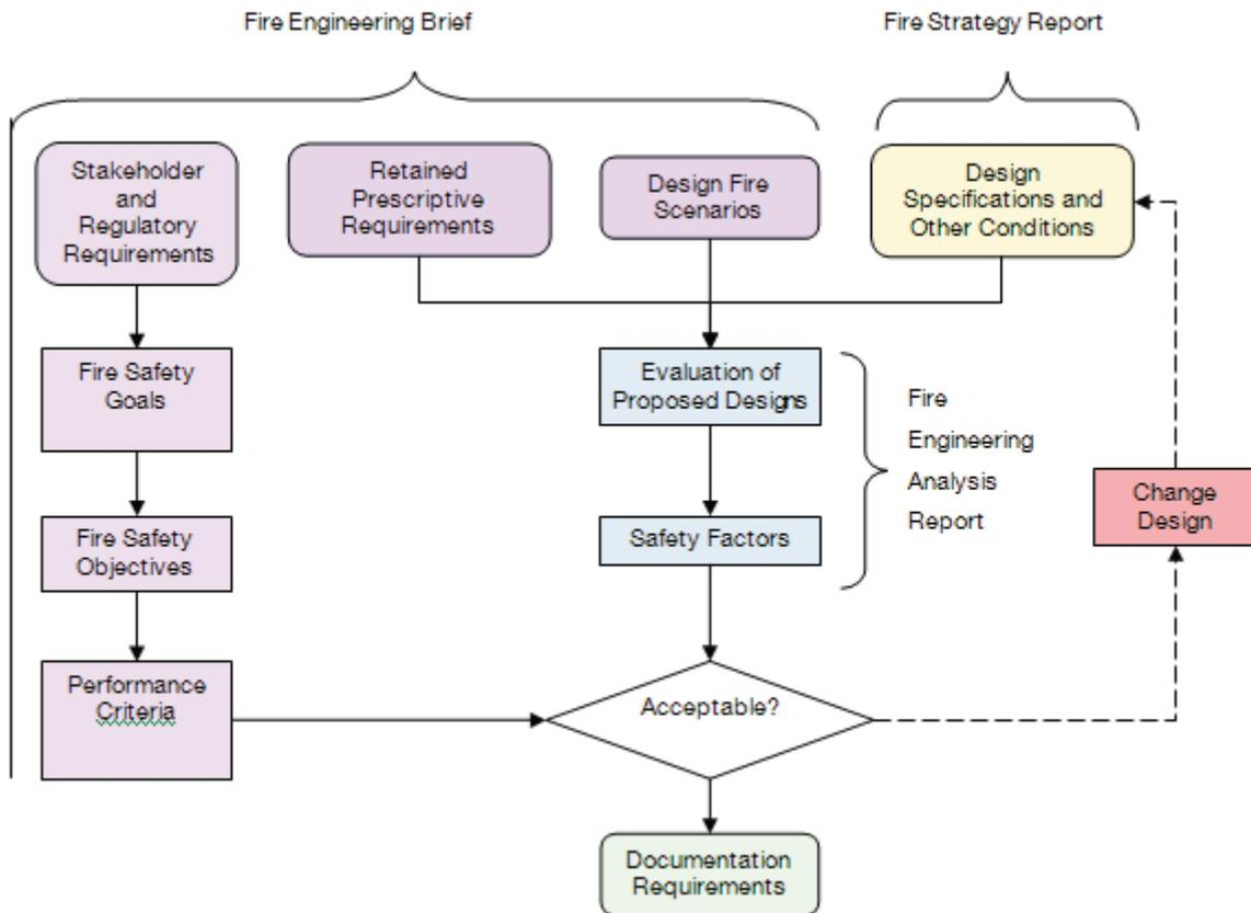
Fig. 15.3 Performance Based Life Safety Code Compliance Process
