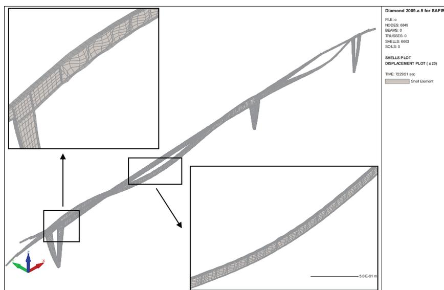
Fig. 14.9 The portal frame deformed shape, when subjected to the natural fire curve in Zone A and to the actions combination 1, at 120 minutes (x20)
