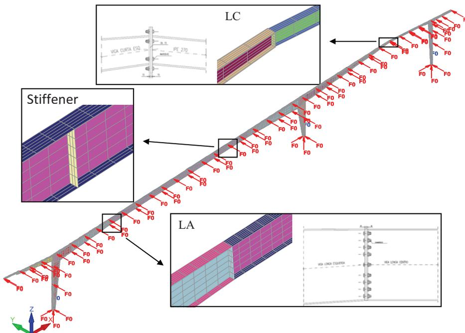
Fig. 14.8 Model restrictions and details of the beam to beam connections and of a transverse stiffener
