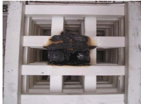
Fig. 18.5 Flame retarded crib at 350sec into the test
