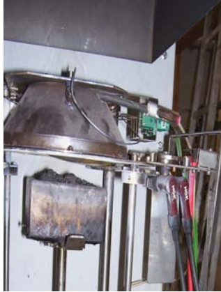
Fig. 18.4 Flame retarded Pine exposed at heat flux 35kW/m 2
