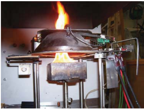
Fig. 18.2 Pine exposed at Heat flux 35kW/m 2
