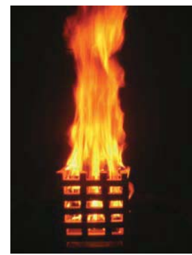
Fig. 18.3 Untreated crib at 350sec into the test
