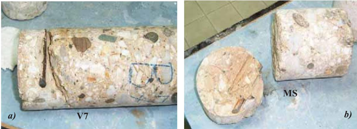
Fig. 31.3 Deterioration of surface layers of specimens
