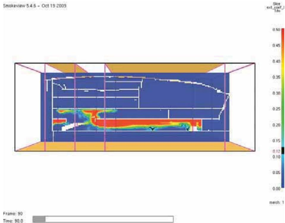
Fig. 29.13 Extinction in the 'head' after its modification in the 90th second
