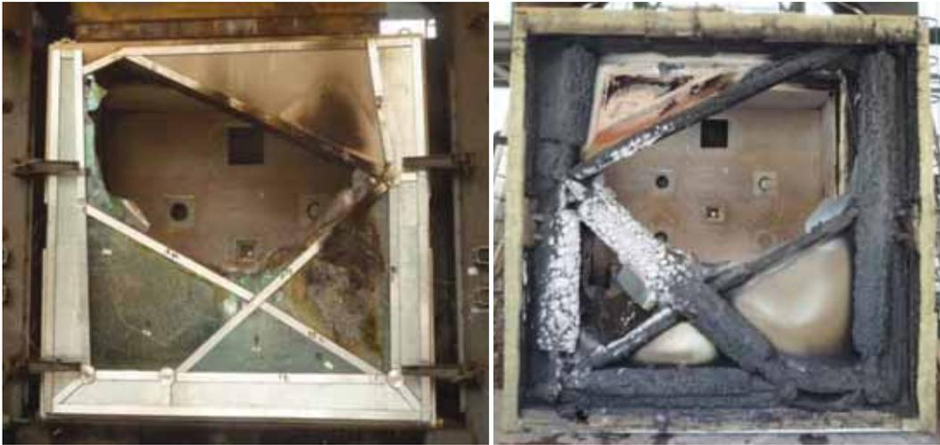
Fig. 29.17 Tested wall model after the fire resistance test
