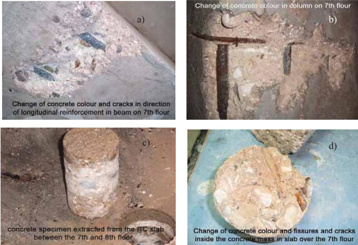
Fig. 31.1 Change of concrete color and characteristic damages of RC elements, recorded in situ
