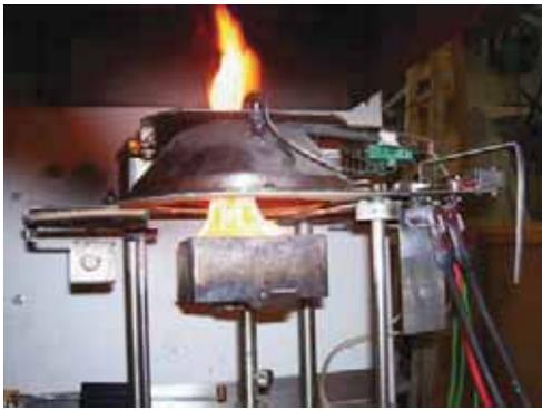
Fig. 18.2 Pine exposed at Heat flux 35kW/m<sup>2</sup>
