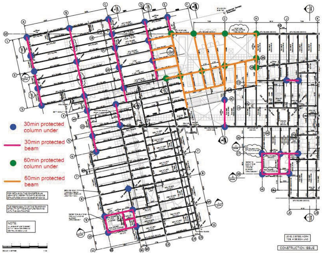
Fig. 26.6 Fire protection steelwork mark-up Level 2 (partial)
