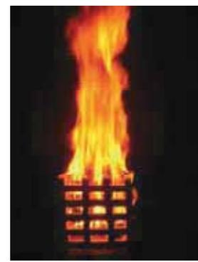
Fig. 18.3 Untreated crib at 350sec into the test
