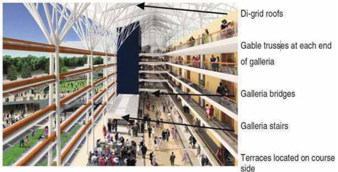
Fig. 8.8 Main structural steel components
