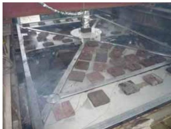
Fig. 29.20 Tested ceiling model after the fire resistance test
