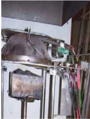
Fig. 18.4 Flame retarded Pine exposed at heat flux 35kW/m<sup>2</sup>
