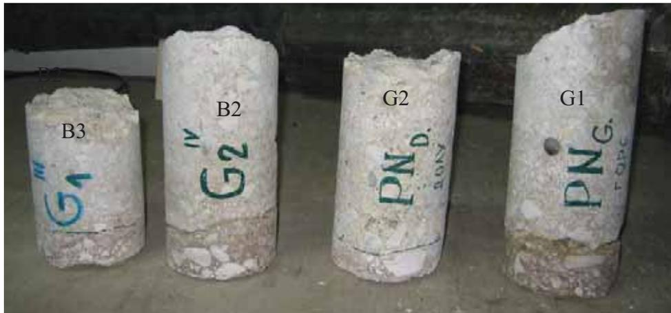
Fig. 30.3 Concrete specimens before testing
