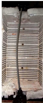
Figure 9. Configuration of the deformed C column after test
