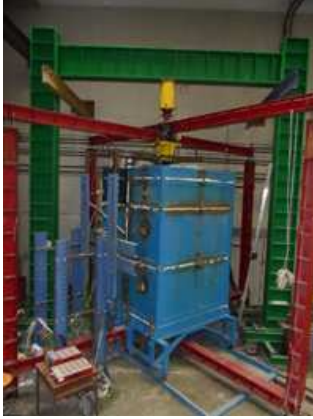
Figure 2. Test set-up for CFS columns
