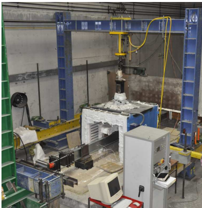
Figure 3. Test set-up for CFS beams
