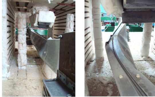
Figure 11. Configuration of the deformed 2R beam after test
