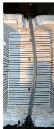
Figure 10. Configuration of the deformed lipped I column after test
