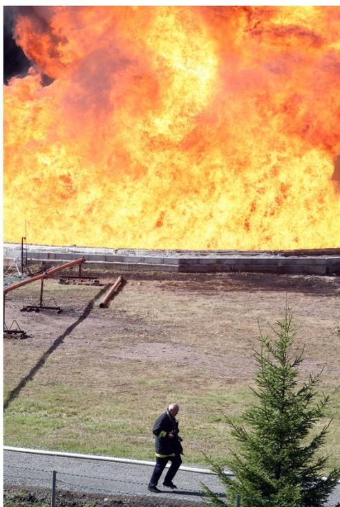
SP Fire Technology recently undertook two fire tests on 20,000 l each of denaturalized ethanol and E85, respectively, in Borlänge. The tests were part of the ETANKFIRE project, the main goal of which is to provide a platform of knowledge ensuring proper investment in fire protection of ethanol storage facilities.
