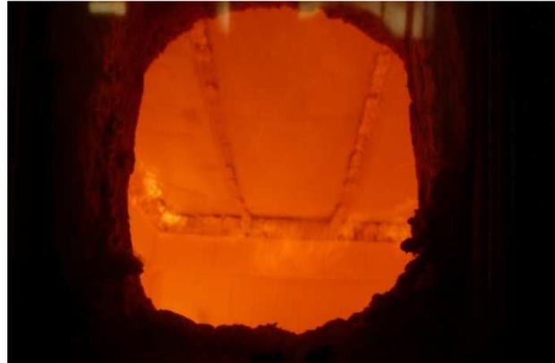
Fig. 14.6 Charring of timber at 45 mins
