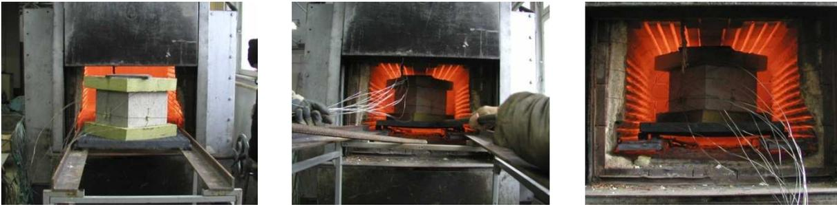
Fig. 9.3 Sample photos of a specimen 30 x 30 cm in the furnace chamber
