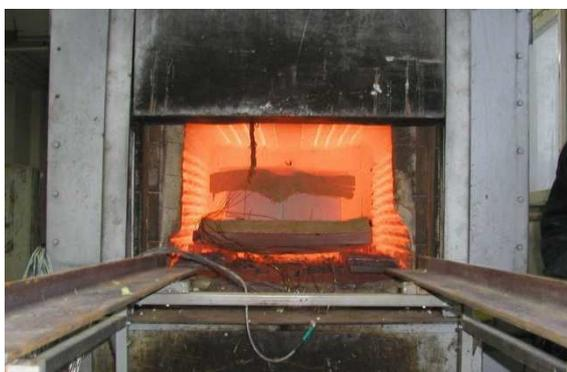
Fig. 9.5 Specimen in the furnace chamber
