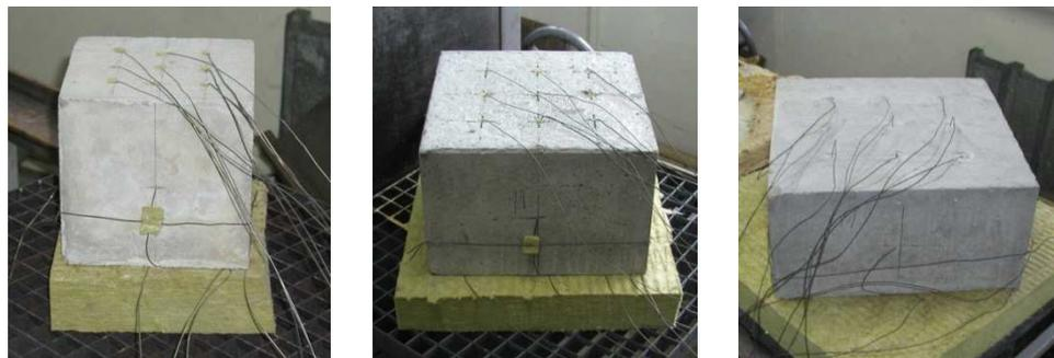
Fig. 9.2 Photographs of specimens with cross sections of 20 x 20, 30 x 30 and 40 x 40 cm
