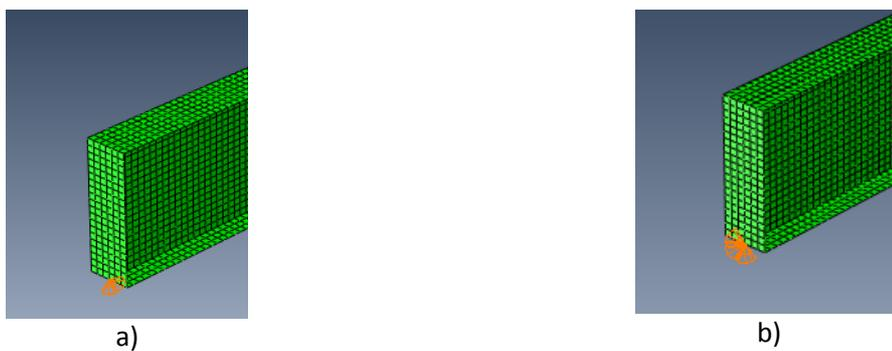
Fig. 6.5 Pin point supports: a) free; b) fixed
