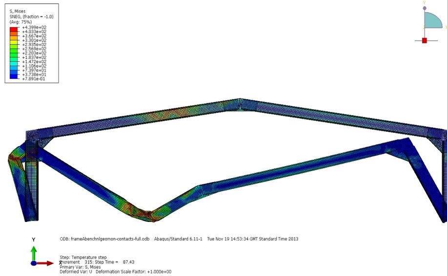
Fig. 21.12 FE Shell Idealisation (nlgeom included) at 403 °C
